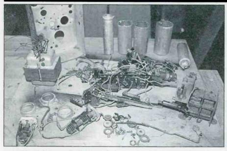
Photo 2. Stripping off everything is the first step in saving the original chassis.
