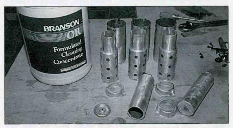
The aluminum tube shields and IF coil covers sport a renewed luster. Weaker areas of the aluminum are beginning to show signs of erosive etching from the action of the organic cleaning agent, however.
