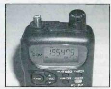
The R2 provides a clear and easy-to-read display (with the slight exception of the "bank" indicators which are small, and very few controls to clutter the front). It takes a bit of getting used to, but it's easy to maneuver once you've spent some time with this receiver.
