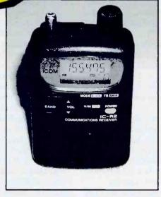
Barely larger than the average pager, the R2 makes a highly portable package. Note the SMA antenna connector on top. These are quickly becoming standard equipment on many portable ham radios and probably won't be too far behind on many scanners, particularly small ones.
