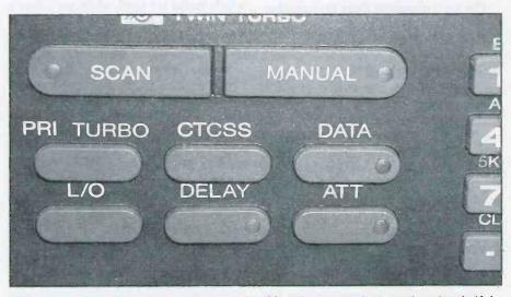
This Uniden BC-9000 scanner features a CTCSS option to restrict incoming signals if the transmitter is carrying a hidden or sub-audible tone. Also note the channel switchable attenuator which can be used only when needed.
