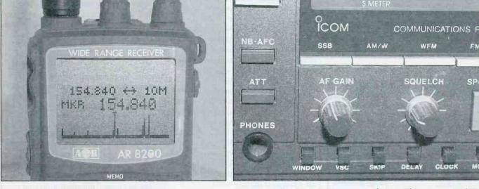
A band scope or spectrum display helps find signals that you may not have known about. Centered on 154.840, this display is 10 MHz wide. So at the left end is 149.840 and at the right side is 159.840. It takes some time to step through all the channels and generate this picture, whereas a true spectrum display unit (SDU) can do it almost in real time.
