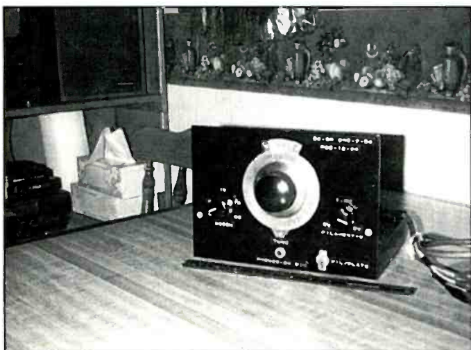
Reader Robert Davey constructed the two-tube regenerative "DX-ER" from plans taken from a 1936 Shortwave Craft Magazine article. The dial is a National Radio type "N." Cardwell Capacitor still produces similar radio dials.
