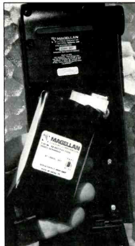
The battery pack can run the GSC 100 for several hours of E-mailing.
