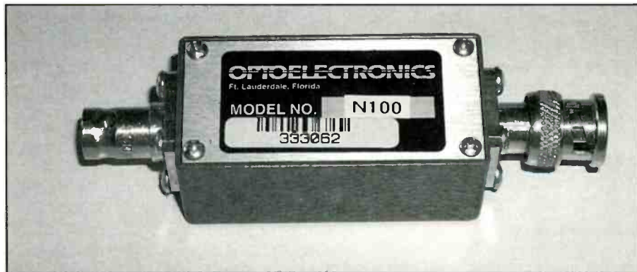
This model N-100 filter from Optoelectronics is an excellent FM broadcast band reject filter, sometimes called an FM Trap. It rejects signals in the 88-108 range and eliminates interference from these strong broadcast signals. This particular one is especially convenient because it has BNC connectors to match your antenna jacks.
