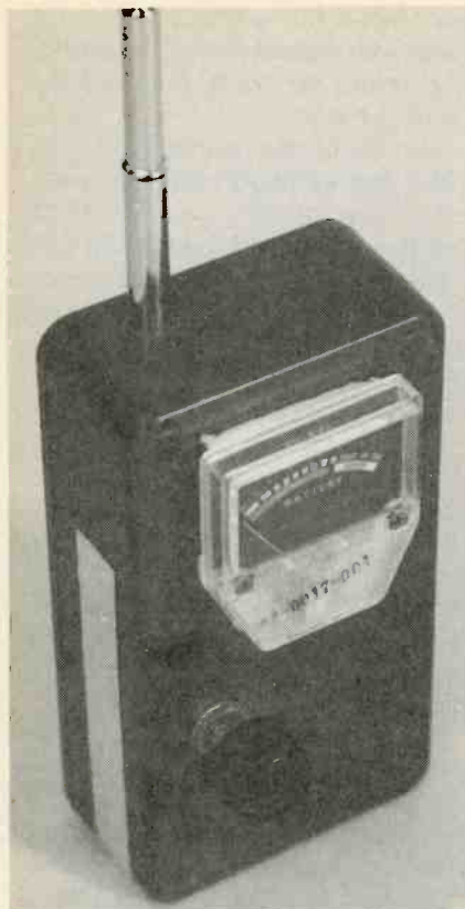
Fig. 1. The Ion Detector is a rather simple circuit consisting of three transistors, (two PN2907 PNP units, and a single PN2222 NPN unit), three resistors, a telescoping antenna (which is used as the ion pickup), and an LED.
