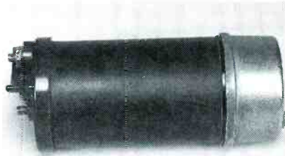
Here's a profile of the induction coil from Vintage Auto Parts. The vibrator mechanism is concealed beneath the metal cap on the right. The input and output connections are on the left.
