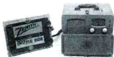
The Zenith 1940 portable had an "airplane luggage" case and a removable loop antenna with suction cups for mounting on car windows.
