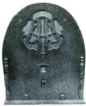
The Cathedral-style Gloritone screen-grid set represents the transitional period of radio-receiver development. Note that the tuning dial is viewed through a tiny window.
