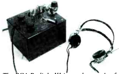
The RCA Radiola III is good example of a typical regenerative receiver. Its two-tube circuit made loudspeaker operation possible, especially on strong local signals.
