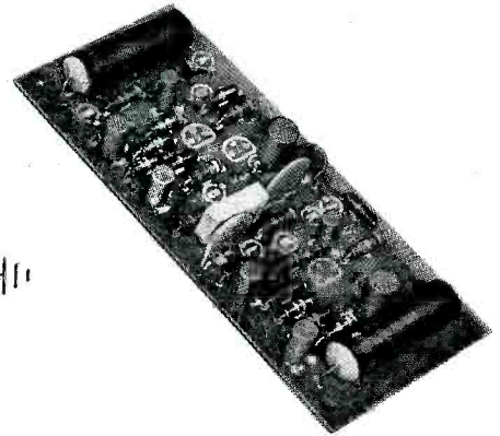
Fig. 12. The author's prototype of the straight preamplifier before installation of transistors.
