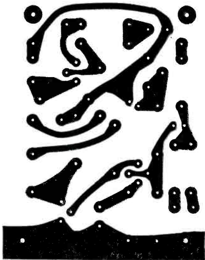
Fig. 2. Actual-size printed board for amplifier. The two power transistors and associated components are mounted externally due to their heat dissipation.
