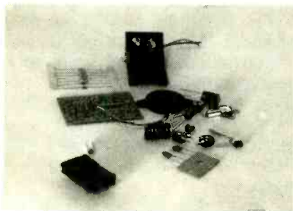
The buzzer used in the project is about 1\frac{1}{8} inches in diameter at its circular center and has red (positive) and black (negative) leads to identify their polarities.
