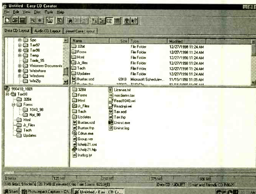
You can skip Easy CD Creator's Wizard and just drag the files you wish to include on your CD-R/RW down to the bottom panel.
