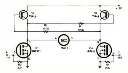
Fig. 4. This circuit differs from previous ones in that it combines a pair of PNP bipolarjunction transistors (Q1 and Q2) with a couple of N-channel HexFETs.
