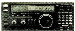
High-end microwave scanning receivers (typified by the Icom models R-7000, R-7100, and R-8500, as well as the AOR 3000, 5000, and 7000) are multi-mode receivers capable of receiving AM, FM, CW, SSB, and sometimes video and digital modes
