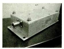
Downconverter/receiver combinations are available to down-shift selected portions of the microwave spectrum for reception via a shortwave or VHF ham-radio receiver.
