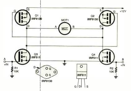
Fig. 6. This circuit, built around a pair of IRF9130 P-channel (Q1 and Q2) and a couple of IRF511 N-channel (Q3 and Q4) HexFETs, operates like the previous circuit.
