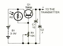
Fig. 8. This simple Light-Activation Circuit can be added to any of the transmitters, except those powered from 12-volt sources, allowing the transmitters to turn on whenever the light level detected by R2 dips below the threshold set by potentiometer R1.
