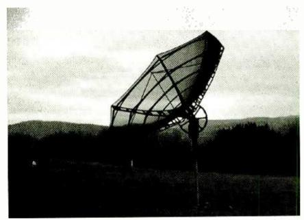
Though many other antenna types have been used successfully, by far the favored antenna for amateur SETI use is the parabolic reflector (or dish). For reception in the 1.3 to 1.7 GHz L-band region, which is highly favored for amateur SETI activity, optimum dish size is about three to five meters in diameter.
