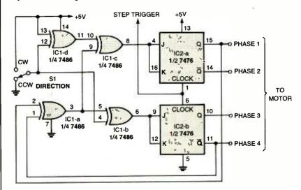
three or four times more. It is important | Fig. 4. A stepper-motor translator circuit can be easily built using a pair of TTL ICs.
