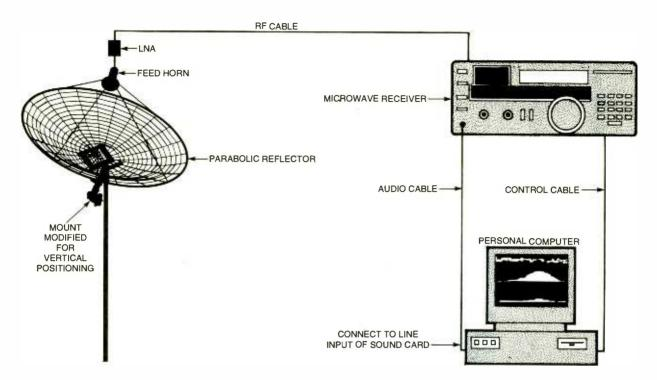
Fig. 1. While no two amateur SETI stations are ever exactly alike, they all have much in common—all contain some sort of antenna, an amplifier, a receiver (aownconverter), and a computer.
