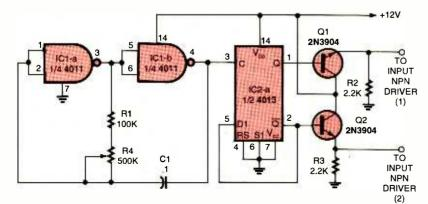
Fig. 3. The complementary outputs of this AC-driver circuit can be connected to the two 68 inputs of any of the NPN-input voltage-reversal circuits.
