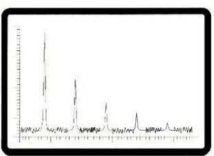
Fig. 2. Spectrum analyzers are essentially swept receivers that display output on a cathode-ray oscilloscope. The amplitude-vs.-frequency plot shown here is an example of such output.
