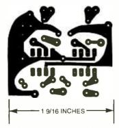
Fig. 4. The author's prototype of the circuit was assembled on a printed-circuit board, measuring 1 % by 1 % inches. A full-size template of the author's board is shown here.
