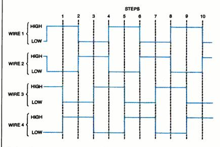
Fig. 2. An alternate to wave-step actuation of four-phase steppers is the enhanced on-on/off-off actuation sequence shown here.
