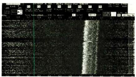
To accomplish their objective—to reach farther and farther out into space in the hopes of contacting intelligent life forms—SETI stations use digital signal processing. Shown here is an example of the first candidate signal received by The SETI League in May of 1996, which turned out to be interference from a classified military satellite.
