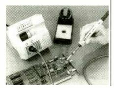
because the heating element is located directly under the tip. Providing tip-to-ground continuity for soldering sensitive electronic devices, this station has a thumbwheel for adjusting the tip temperature from 65° to 450°C (150° to 840°F).
