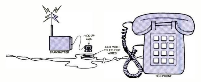
Fig. 5. The telephone pick-up coilltransmitter combination is sensitive enough that it can be used to inductively snare conversation from a coiled section of telephone line.
