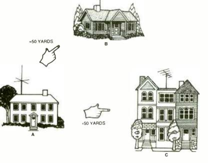
dustrial and mobile. Fig. 1. This diagram shows the layout of one of the first EMI trouble spots I looked into. House "A" was the site of the CB equipment involved, while "B" and "C" were sites of interference.
