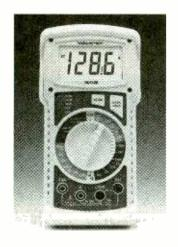
Functions include a 1500 VDC/1000 VAC voltage range; measurement of current to 10A and resistance to 20 megohms; and continuity, diode test, and data hold. A unique Safety Tester feature quickly checks for live circuits and indicates the presence of common power-supply voltages with a series of LEDs. Other features are high-voltage alerts, thirty-minute autooff to preserve battery life, anti-skid rubber holster, and tilt-stand.
