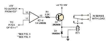
Fig. 5. In this circuit, the dual monitoring system opens up a load relay should the supply voltage fall outside the preset voltage range.
