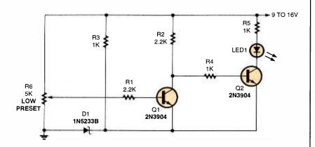
Fig. 7. Use this simple low-voltage monitoring circuit to check any drop in the supply voltage below a preset level.
