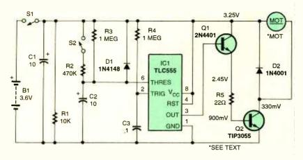
Fig. 1. The Flight Timer is a very simple circuit built around a single integrated circuit, a pair of transistors, a motor, and a handful of support components.
