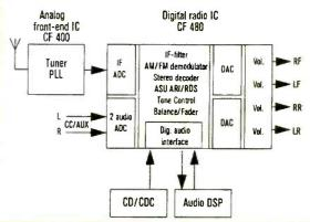
As a result of high-integration strategies, the complete functionality of a top-level car radio has been reduced to a two-chip set. The digital radio IC contains additional inputs for both analog and digital sources plus a communications interface for digital signal processing.
