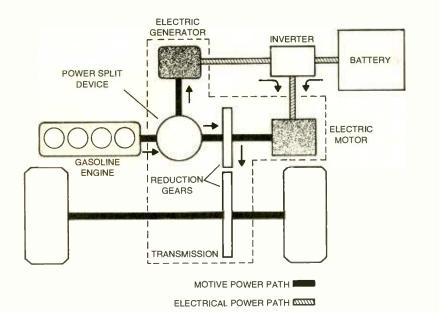
Fig. 5. The Toyota Hybrid System used in the Prius. The Toyota Hybrid System uses a small 1.5-liter, 58-horsepower gasoline engine, a 30-kW motor-generator, a constantly-variable transmission, and a NiMH battery pack. (Toyota)
