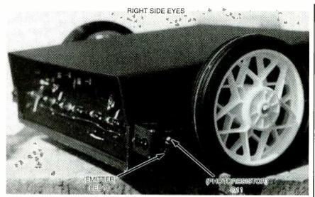
Mounted on brackets to either side of the Seeing Eye Robot's enclosure are an IR LED/phototransistor pair that give the unit human-like peripheral vision. If the unit is housed in a semi-spherical enclosure, the shape of the enclosure and the positioning of the IR LED/phototransistor pairs allow the unit's vision circuit to more closely emulate human sight.
