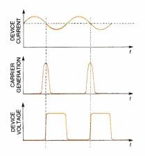
Fig. 3. Examples of IMPATT voltage and current waveforms.
