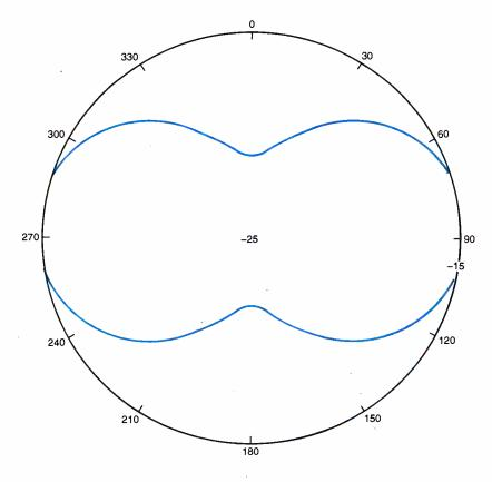
Fig. 3. Azimuthal antenna pattern at 9.75 MHz. Here the pattern is similar to the conventional dipole—both in gain and orientation.
