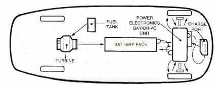
Fig. 1. The typical HEV has a small internal-combustion engine, motor/generator, and some form of energy-storage device—usually a battery, although a flywheel or ultra capacitor might be used. Only one power source, usually an electric motor, is used for propulsion in a series HEV system. The other source, typically an ICE, is used for battery charging and an additional source of power when needed such as for acceleration or high climbing. (General Motors)
