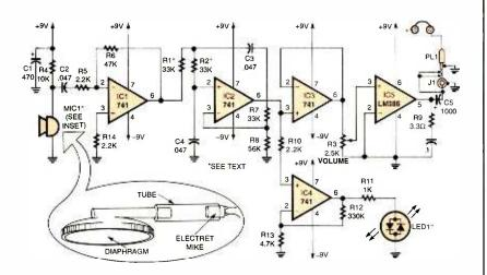
Fig. 6. This high performance electronic stethoscope is much more sensitive than the standard mechanical types, and can also be used in any number of different projects.
