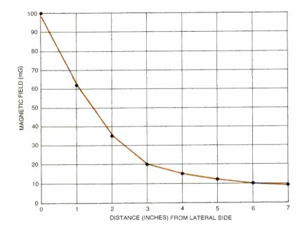
Fig. 3. Shown here are variations in the strengths of the magnetic field generated by a steam iron depending on the distance from its lateral side.
