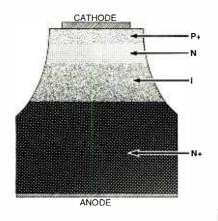
Fig. 2. A vertical IMPATT diode structure.
