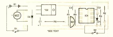
Fig. 3. Assemble the Flight Timer's printed-circuit board guided by this parts-placement diagram, starting with the passive components, followed by the semiconductors.
