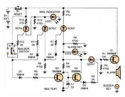
Fig. 5. Here's a mailbox monitor circuit that not only alerts you when the mailbox is opened, but incorporates an alarm feature which goes off when the box is opened by unauthorized personnel.
