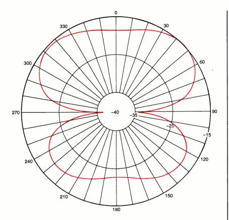
Fig. 4. Azimuthal antenna pattern at 15 MHz. Major lobes are now in North-South direction with sharp nulls broadside to the antenna orientation.
