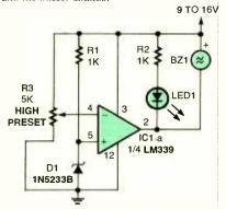
Fig. 2. In this over-voltage monitoring circuit, should the supply voltage rise above the nominal 6-volt Zener reference, the light and buzzer are activated.
