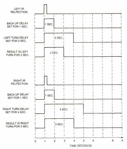
Fig. 3. As shown by these timing diagrams, the circuit's operation depends heavily on fairly precise timing/delay cycles that cause the two driven wheels of the robot to act independently and in concert.
