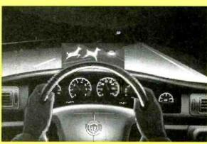
The head-up display projects a virtual image onto the windshield, allowing the driver to keep his eyes on the road.
