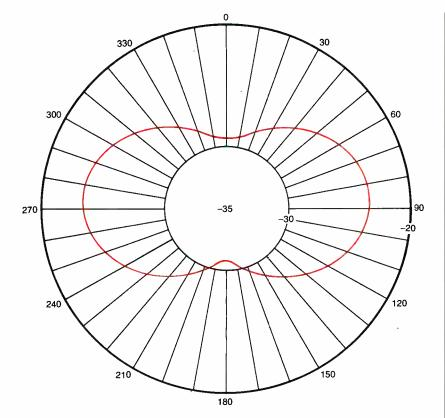
Fig. 6. Azimuthal antenna pattern for a 100-foot horizontal end-fed configuration (random-length Marconi antenna) at 5 MHz. Pattern is similar to a classical dipole antenna at the half-wavelength frequency.
