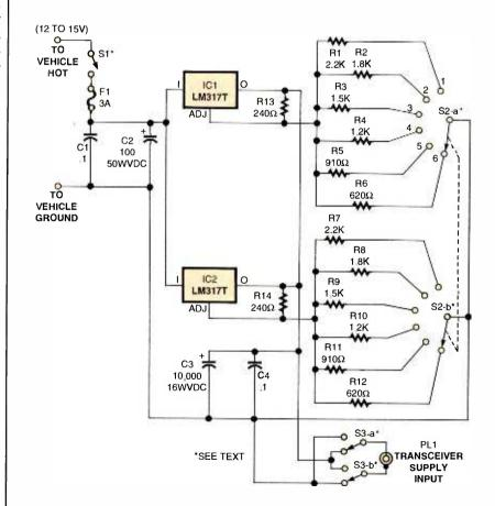
Fig. 4. This handy adjustable DC power supply, driven by your automobile's battery, can provide regulated voltages from 4.5 to 13 volts with output currents up to 3 amps. It's ideal to power up a handheld ham transceiver in you car.
