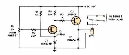
Fig. 8. In this over-voltage monitoring circuit, the relay removes the load from the supply should the 58 supply voltage exceed a preset value.
