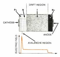
Fig. 1. An example of a typical IMPATT diode structure.
