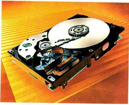
Pictured here is Seagate's Cheetah 9LP hard drive, which has the fastest average seek time of any Winchester-type disc drive, as low as 5.2 msec during read operations. The drive also delivers top 36 performance with sustained data transfer rates reaching over 20 Mbps.
