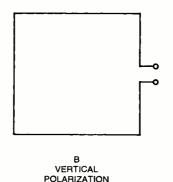
Fig. 2. By feeding the square loop in either horizontal side, as in A, the quad exhibits horizontal polarization; when the feed is changed to either side, as in B, vertical polarization occurs.
