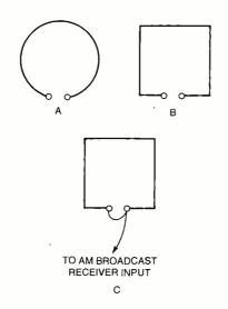
Fig. 1. This figure illustrates three configurations of loop antennas. The balanced loop is circular in (A) and rectangular in (B). In (C), a rectangular loop is shown fed as a single-ended source using ground as a return path.
