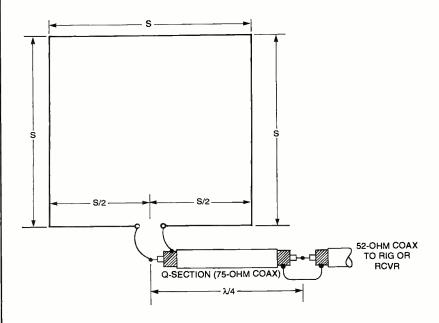
Fig. 1. The one wavelength quad loop antenna is horizontally fed and uses a ( $\lambda/4$ ) Q-section for matching to 52-ohm coax transmission line.
