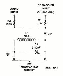
Fig. 4. This simple circuit is a great way to produce amplitude modulation. Experiment with the diode for best mixing characteristics.
