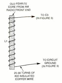
Fig. 4. Without an external or pull-up antenna? Use this coupling antenna as an alternative.
