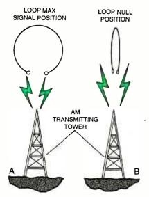
Fig. 5. This figure illustrates the proper positioning for a loop antenna. In (A) when the loop antenna is broadside (maximum area exposed to the incoming RF energy), the reception will be maximized. As the plane of loop is rotated 90 degrees, as in (B), the signal strength is minimized, or nulled out.
