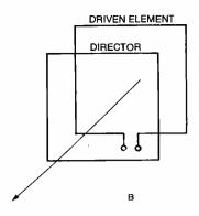
Fig. 3. A two-element cubical quad antenna consists of the driven element and a parasitic element. When the parasitic element is placed in back of the driven one, as in A, it is called a reflector. With the parasitic element placed in front, as in B, it is called a director. Electrical characteristics of both configurations are essentially the same—main beam is perpendicular to the plane of the loops in the direction shown.
