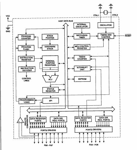
The Atmel/MVS 1200 microcontroller block diagram. This microcontroller can run with no (!) external components, provides 15 bits of I/O, has 512 words of flash program memory, 64 bytes of EEP-ROM, an analog compactor, and supports in-circuit programming. With care, you can program it directly via the serial or parallel port of a PC.
