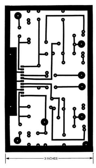
Fig. 3. The Portable CD Amp was assembled on a printed-circuit board, measuring 3 by 51/16 inches. A template of the author's printed-circuit layout is shown here full-size.
