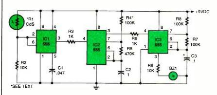
Fig. 5. This fun circuit simulates the chirp of a cricket—complete with a photo cell, which shuts down the circuit when a light shines on the "cricket!"
