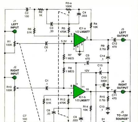
Fig. 1. At the heart of the Portable CD Amp is an LM2877 dual four-watt audio-power amplifier (IC1), a single-inline monolithic chip that requires few external components and can be operated from supply voltages ranging from 12- to 20-volts.
