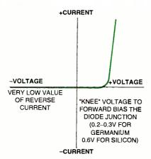
Fig. 3. Voltage-current characteristics of a typical diode.
