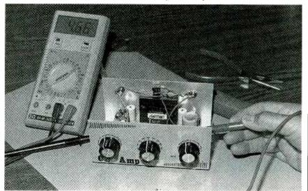
When taking resistance measurements, be sure to turn power to the Portable CD Amp off; failing to do so will damage the resistance measuring circuitry of the meter. When taking voltage measurements be sure that the meter is set to the DC scale and on a range that is higher than the anticipated voltage in the circuit.
