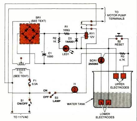
Fig. 7. Here's a useful circuit around the homestead that will always ensure a full water tank. It takes a little skill to set up and adjust those electrodes. Equivalent electrical parts for the circuit are RadioShack 276-1067 for SCR1 and RS 276-1101 for the 1N4001s. You can always use their modular rectifier unit, such as the RS 276-1146, to save some space.
