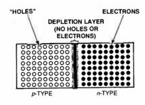
Fig. 1. A PN junction with no voltage applied. **DEPLETION LAYER**
