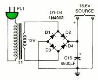
Fig. 2. The author's version of the Portable CD Amp was powered from a 12-volt DC power supply comprised of T1 (a 12 volt, step-down transformer), D1-D4 (four 1N4002 1-amp, 100-PIV rectifier diodes, which form a full-wave bridge rectifier), and C16 (a 6800-\(\mu F\), filter capacitor).
