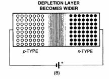
Fig. 2. When a positive voltage is applied (forward bias), as shown in (A), the depletion region becomes narrow and a high forward current flows; when this voltage is reversed (reverse bias), as in (B), the depletion layer becomes wider and very little current flows.
