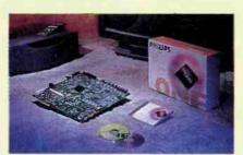
Philips Semiconductors' TriMedia programmable DTV reference platforms allow hardware and software manufacturers to quickly develop ATSC products.
