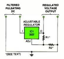
Fig. 1. Here's the typical adjustable regulator circuit. This time we are going to use it to control current rather than voltage.
