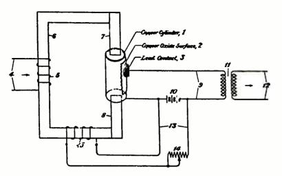
Fig. 1. Was this the first solid-state amplifier? It used a magnetic field to control the current across a copper/copper-oxide junction. The inventor, Russell Ohl, was a respected scientist who later invented the PN junction, so the amplifier probably worked. Unfortunately, tubes were on center stage in 1930.
