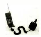
When the caller presses the red button for at least two seconds, the attached cellular phone automatically dials 911, cpening a line to the agency that monitors cellular 911 calls. If an emergency occurs during a routine call in progress, pressing the red button immediately terminates that call and initiates a 911 call instead. The red button is well-illuminated for enhanced nighttime visibility.
