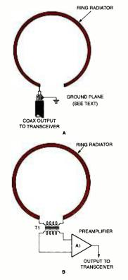
Fig. 1. Two cases of the ring loop antenna. In (A), the antenna is unbalanced, or single-ended. requiring a good ground connection; while in (B) the balanced ring loop antenna is trans-60 former-coupled to a differential preamplifier.
