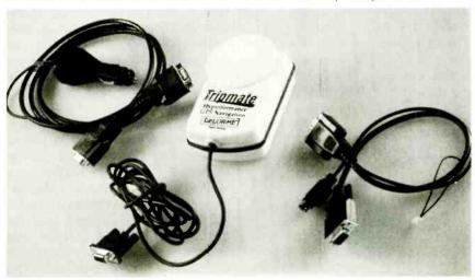
The DeLorme Tripmate, which has two different power adapter kits, can be powered from 4 AA batteries, or through a cord that allows it to receive power from the vehicle's cigarette lighter or from the laptop itself.
