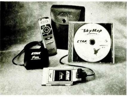
The Etak SkyMap package consists of a 12-channel PCMCIA card GPS receiver, a GPS antenna, and two CD-ROMs containing the digital database to map the continental US. The package also features a Sony IR remote control that can be used in addition to a mouse and keyboard.
