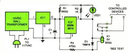
Fig. 5. Experiment with Hall-effect switches! In this circuit, the magnetically-activated Hall-effect switch, IC2, controls operation of a low-power relay.
