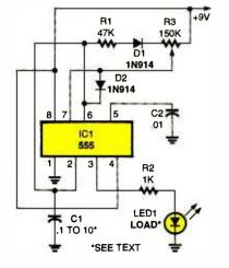
Fig. 5. This little pulse-width generator can drive low-current devices.
