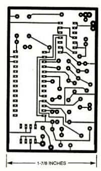
Fig. 2. The Telephone HangUp Module was assembled on a printed-circuit board, a full-size template of which is shown here.
