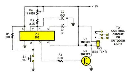
Fig. 2. With this circuit, you can activate an outdoor light or other devices and keep them turned on for a short period of time.
