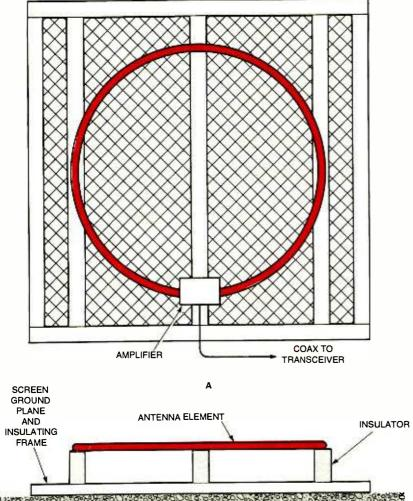
Fig. 2 Mounting the ring antenna in the horizontal plane. In (A) the top view is shown over a conductive screen ground plane, while (B) illustrates the front view including the insulated supports.
