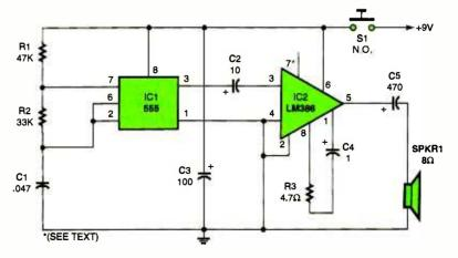
Fig. 2. Replace your electromechanical buzzer with this simple solid-state circuit.
