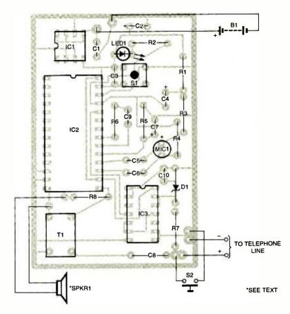
Fig. 3. Assemble the Telephone Hang Up Module's printed-circuit board guided by this parts-placement diagram.
