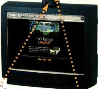
2. The transmitter on the TV sends input from the keyboard to your PC—through walls, reilings and floors up to 100 feet away—via RF technology.
