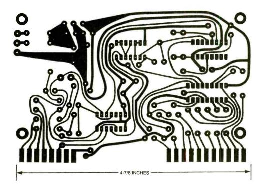
Fig. 2. The Digital Capacitance Meter was assembled on a pair of printed-circuit boards: the main board and the display board. A template for the main printed-circuit board is shown at full size.
