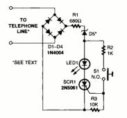
Fig 6. Build this neat "ON-HOLD" circuit to completely silence conversations on both ends end of the phone line.
