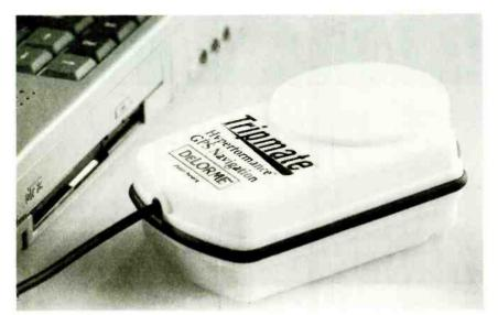
The DeLorme Tripmate Hyperformance GPS Navigation system offers capabilities similar to those of Etak's SkyMap through a 12- channel GPS receiver that plugs into the laptop's serial port via a six-foot vable. It's CD-ROM map database covers the entire North American continent and the Caribbean—and includes about 66,000 restaurants, hotels, and other points of interest.
