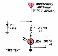
Fig. 6. Want to find out if your ham or CB transmitter is generating any RF output? Then bring the monitoring antenna close to your transmitter and key-down the rig—wait and see the LED lights.
