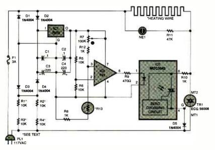
Fig. 1. The Heated Pet Pad is comprised of a 7812 12-volt, 1-amp, voltage regulator (ICI); a 741 op-amp (IC2); and an MOC3042 zero-crossing, Triac-driver, optoisolator/coupler (IC3); a negative-temperature-coefficient (NTC) thermistor (R13); a 15amp, 600-volt Triac (TR1); 19 feet of Nichrome heating wire; five 1N4004, 1-amp, 400-PIV rectifier diodes (D1-D5); and a few additional components.
