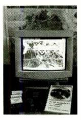
Connecting the demodulator between the computer's serial port and a SSB shortwave communications receiver, enables digital radio transmissions to be received, displayed, printed, or recorded on to disk. SSC's Windows FSK demodulator allows the program to operate in the background.
