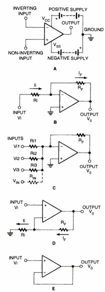
Fig. 1. The commonly accepted schematic symbol for the operational amplifier is shown in A. The op-amp's inverting configuration is shown in B, a summing amplifier is shown in C, the non-inverting configuration is shown in D, and E shows a non-inverting voltage follower configuration.
