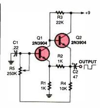
Fig. 7. Here's a neat circuit to generate squarewaves in the audio range. Try using this output to clock other circuits.
