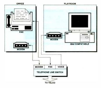
Use a telephone-line switch "backwards" to avoid outgoing line contention.
