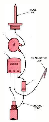
Fig. 7. The RF Sniffer was assembled in two sections—the probe and the amplifier/annunciator. Details on building the probe, which was built into the body of an old BIC pen, are shown here.
