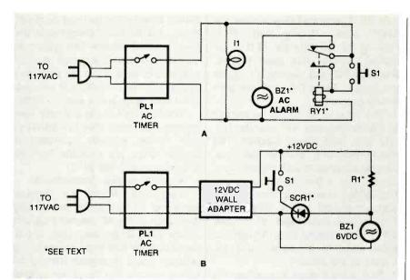
Fig. 4. The circuit in (A) uses the programmed AC timer to set the buzzer/relay after a known amount of time. A similar circuit in (B) uses a 12-volt adapter to supply the power to the low voltage components.
