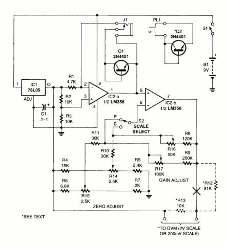
Fig. 10. The Electronic Thermometer can be used to convert any digital voltmeter (DVM) into a reasonably accurate thermometer capable of measuring from about  $-40^{\circ}$  (C or F) to over 150°C (302°F). Or, if desired, a dedicated digital voltmeter module can be permanently connected to the circuit.
