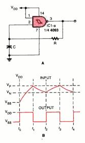
Fig. 2. A single gate from the 4093 can easily be configured as an oscillator as shown in A. The input/output characteristic waveforms for that circuit are shown in B.
