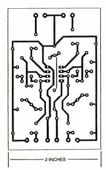
Fig. 4. The Magnetic RIAA Phono Preamp was assembled on a small printed-circuit board. A template of the printed-circuit artwork is shown here full-size.
