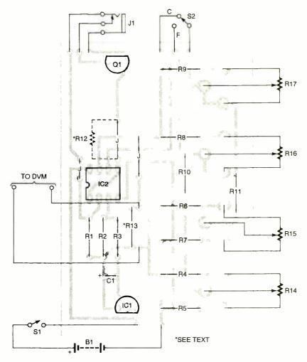
Fig. 12. Assemble the Electronic Thermometer, guided by this parts-placement diagram. Once the board is fully assembled, it can be housed in an enclosure of your choice.
