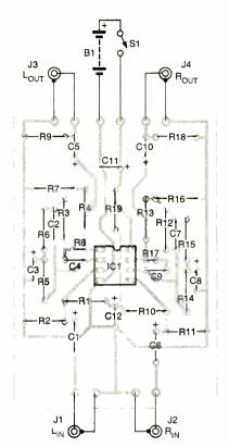
Fig. 5. Assemble the printed-circuit board for the preamp guided by this parts-placement diagram. Be sure to use shielded cable to make the connections between the circuit board and the input/output jacks.
