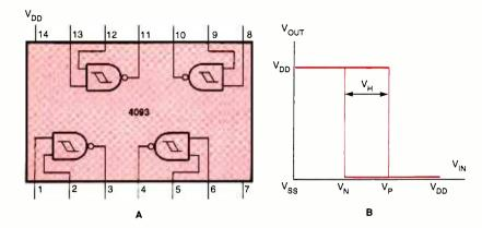
Fig. 1. The 4093, which is housed in a 14-pin package, is comprised of four 2-input NAND Schmitt triggers (as shown in A) that can be used independently. Transfer characteristics for the 4093 quad NAND Schmitt Trigger are shown in B.
