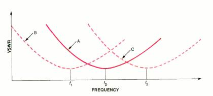
curve that is centered on the desired | Fig. 2. Family of VSWR-vs.-frequency curves illustrating off-resonance conditions.
