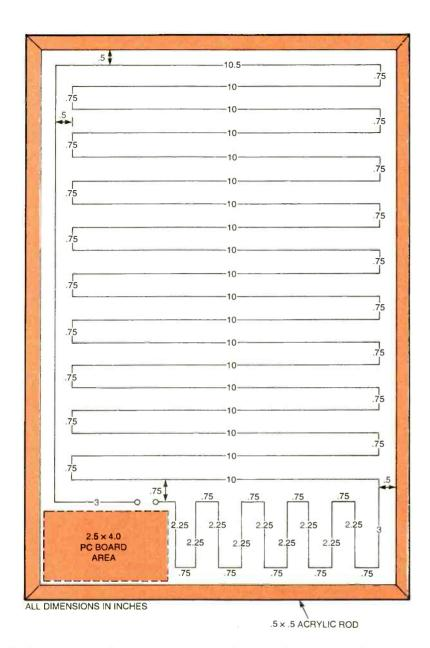
Fig. 3. Glue four lengths of  $V_2$ -inch square acrylic bar stock (mitered to  $45^{\circ}$  to form good  $90^{\circ}$  corners, as shown) around the edges, using a thickened clear acrylic cement. Following the pattern shown, lay down the #30 enamel insulated Nichrome wire heating element, and tape it in place with #69 Scotch glass-cloth electrical tape.
