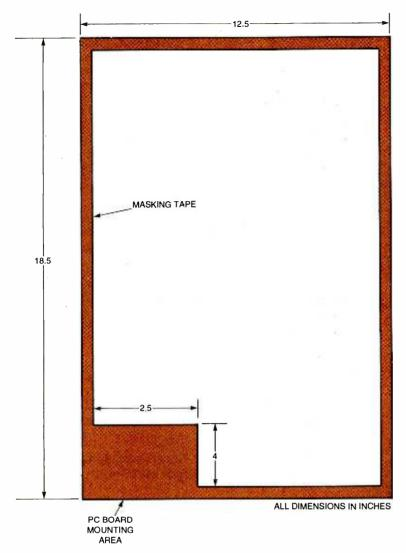
Fig. 2. The Heated Pet Pad was assembled in two steps. Outlined in this illustration is the beginning of the heated pad (with heating element) and its enclosure. Start by cutting two pieces of ABS plastic sheeting (one piece 0.098-inch thick for the top and the other 1/8-inch thick for the bottom) to 12-1/2 by 18-1/2 inches. Then cover the edges of the 0.098-inch piece with 3/4-inch masking tape. Also mask an area of 2-1/2 by 4 inches in one corner, for the unit's printed-circuit board.
