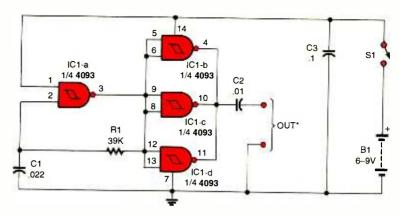
Fig. 3. The oscillator circuit shown in Fig. 2 can be used to form the basis of a simple Signal Injector. The oscillator portion of the circuit is built around IC1-a, which produces a square-wave output. The other three gates are used to boost the output current to a level sufficient to drive the input of the circuit to be tested.
