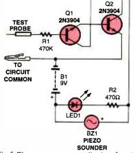
Fig. 5. There are numerous applications for this tester—when the probe senses any voltage greater than 1.5 volts, the buzzer will sound and the LED will light.
