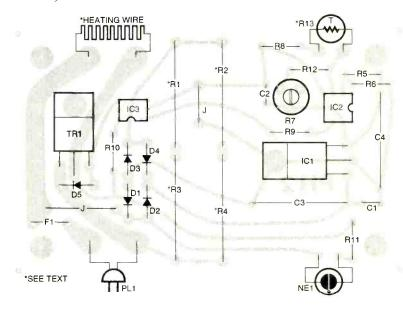
Fig. 5. Assemble the printed-circuit board according to this parts-placement diagram, saving the heating element for last. Connect the thermistor to the board via a pair of 6-8inch lengths of insulated hookup wire and cover the solder joints at the thermistor with heat-shrink tubing or some glass tape.
