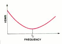
Fig. 1. VSWR-vs.-frequency curve.
