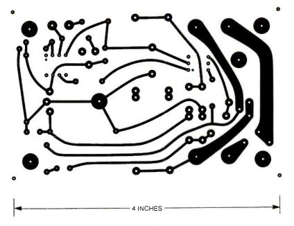
Fig. 4. Most of the electronics for the Heated Pet Pad were assembled on a printed-circuit board, measuring 2-1/2 by 4 inches. A template for the printed-circuit layout is shown here full size.
