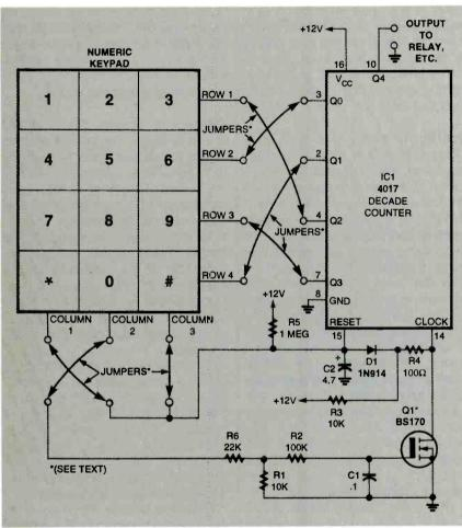
Fig. 6. In this circuit, a standard telephone-type keypad is used to provide a digital lock. The relay will not operate unless it receives the correct four-digit code.
