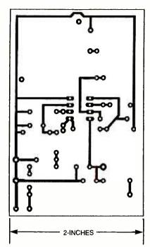
Fig. 8. The second half of the RF Sniffer, the amplifier/annunciator, was assembled on a small printed-circuit board. A template of that board layout is shown here full-scale.
