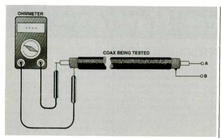
Fig. 3. Resistance checks of a coaxial cable.
