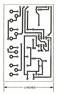
Fig. 11. The Electronic Thermometer was assembled on a small printed-circuit board, measuring 2 by 3 inches. A template of the printed-circuit-board artwork is shown here full-scale.
