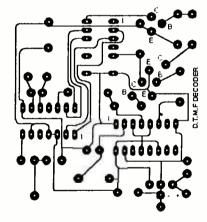
Here is a cleaned-up version (less the ink bleed runovers) of the tone-decoder foil pattern of Fig. 5, page 41 (Popular Electronics, July 1997).
