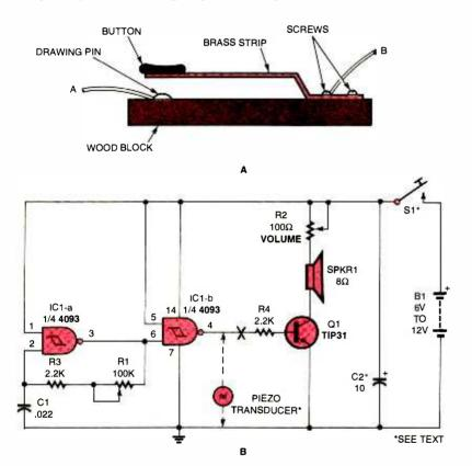
Fig. 7. This circuit was designed with the aspiring ham or Boy Scout working toward an award in communications in mind. The circuit is comprised of the homebrew sending key shown in A and the variable-frequency oscillator shown in B. Switch S1 represents the sending key.
