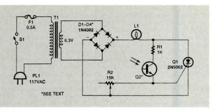
Fig. 7. This trick circuit uses a photo-transistor and SCR to control lamp L1. Light impinging upon Q2 turns on the lamp—removal of the light turns the lamp off.
