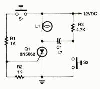
Fig. 3. In this case, auxiliary switch S2 turns off the lamp by reversing polarity of the voltage across the SCR.
