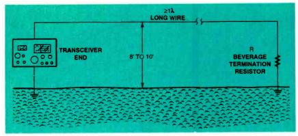
Fig. 1. The Beverage antenna for low frequency reception.
