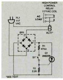
Fig. 6. Here the SCR is used to control the turnon of an AC relay coil that operates an AC load. Switch S1 is tied back to the load—controlling operation of the relay.
