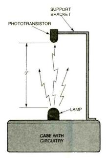
Fig. 8. The magic lamp circuit can be constructed in this small enclosure.
