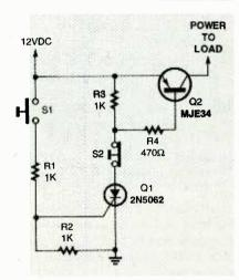
Fig. 5. This neat circuit operates as an on/off latching switch to control power to a load. Closing switch SI sends power to the load, while pressing switch S2 removes this power flow.
