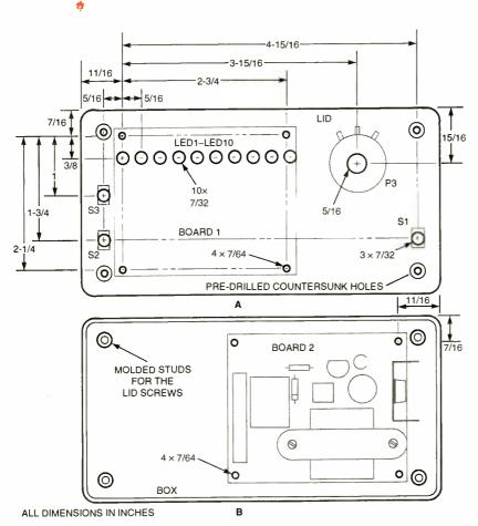
Fig. 4. The placement and dimensions of holes for mounting board 1 to the lid are shown in A, while B shows the mounting location of board 2 in the bottom of the enclosure. Board 1 is mounted to the lid on  $l_{1_2}$ -inch spacers. Board 2 is mounted on  $l_{1_4}$ -inch spacers to the bottom of the enclosure.
