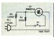
Fig. 9. In this circuit, a triac is used to control power to load the RI.
