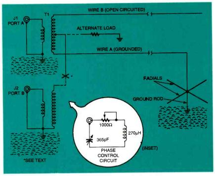
Fig. 10. Steerable-notch Beverage antenna.
