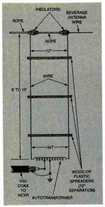
Fig. 9. Zepp-fed Beverage antenna.
