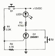
Fig. 2. With the LED on, auxiliary switch S2 can be used to turn the lamp off by providing a shuat path around the SCR.
