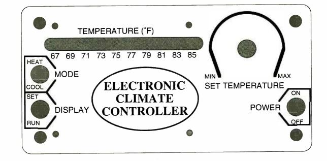
Fig. 5. Shown here, at full size, is the author's front-panel layout for the ECC. The layout can be photocopied and glued to the lid of the enclosure to give the unit a professional-looking finish.
