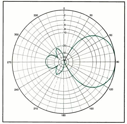
Fig. 3. Directivity pattern for a  $1\lambda$  Beverage terminated in its characteristic impedance.
