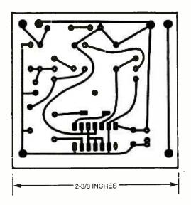
Fig. 2. For ease of construction, while reducing the possibility of construction errors, it is recommended that the project be assembled using this template of the author's printedcircuit layout, which measures  $2-3_{l_8}$  by  $2-l_{l_8}$  inches.
