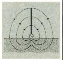
Fig. 2. Electric field lines as source of ground currents (side or elevation view).
