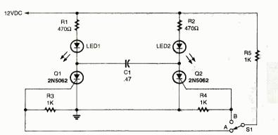
Fig. 4. Here's an arrangement of SCRs in a flip-lop circuit. Each LED's turn-on will toggle in accordance with the position of switch S1.
