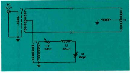
Fig. 11. Balanced version of the steerable-notch Beverage.
