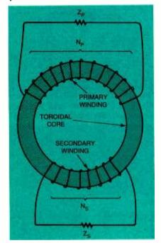
Fig. 6. Toroid transformer for the receiver end.
