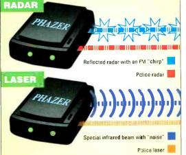
waveguide antenna, effectively confusing the computer inside the radar gun. The laser component transmits an infrared beam that has the same effect on laser Lidar units.
