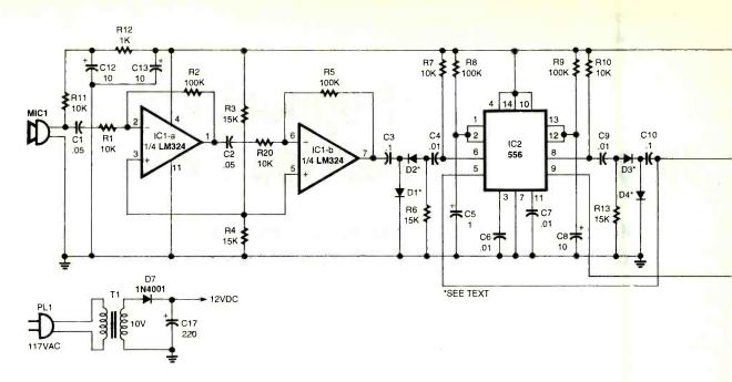
Fig. 3. Here's another amazing circuit. The two output relays can control a number of electronic devices. Just a clap of your hands twice, or almost any other quick double sound within a one second interval will activate operation.
