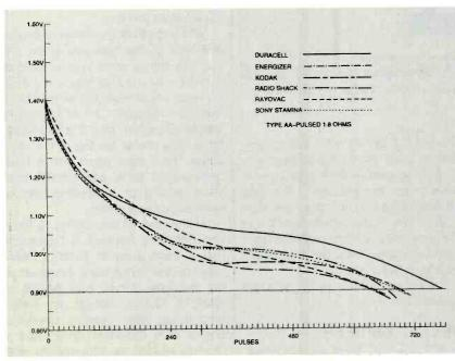
Battery output voltage versus pulsed 1.8-ohm load.
