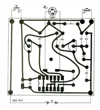
Fig. 3. Once you've etched your printed-circuit board and obtained all of the components listed in the Parts List, assemble the printed-circuit board, using this parts-placement diagram as a guide. Be sure to pay close attention to the orientation of the polarized components.
