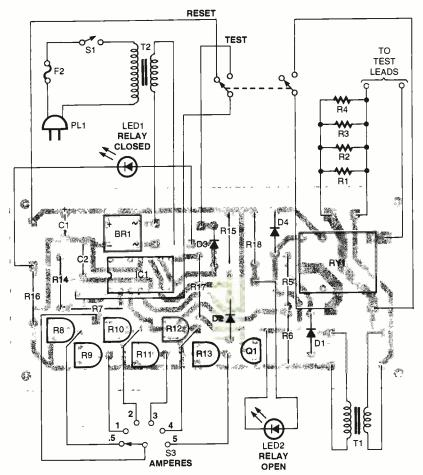
Fig. 3. Assemble the Fusesaver guided by this parts-placement diagram. When assembling the Fusesaver, be certain that the 117-volt, AC components are kept safely isolated from the DC circuitry. Also be sure that the four 0.47-ohm, 5-watt, power resistors (R1-R4) are afforded ample airspace to avoid overheating.
