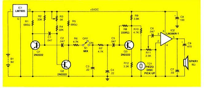
Fig. 3. This neat circuit provides dual functions for the budding musician. The external pickup can be fed directly to a power amplifier or mixed with a precise 440-Hz "A" tone.
