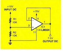
Fig. 1. This handy little circuit forces the opamp's output at a value to be determined by the voltage divider of R1 and R2 and the supply voltage. Use this feature to supply a fixed bias voltage reference for other devices. In the case shown, the output voltage is one-half the supply voltage.
