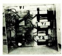
The Fusesaver was mounted in a medium-sized vented metal enclosure. The leads of the two power transformers were bent outward at a 90° angle and then mounted to the bottom of the enclosure. Several layers of electrical tape were positioned directly under the units to prevent them from shorting to the enclosure.
