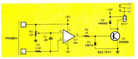
Fig. 5. Need a circuit to sense a voltage change and, in turn, drive a relay? Look no further! When the probes sense a voltage change, such as the presence of water. relay RY1 will be activated and shut down the water valve.
