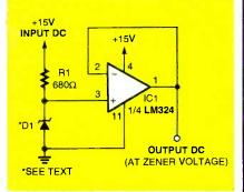
Fig. 2. Similar to the circuit of Fig. 1, but by using the zener diode on the input, the output voltage will be at the zener voltage.
