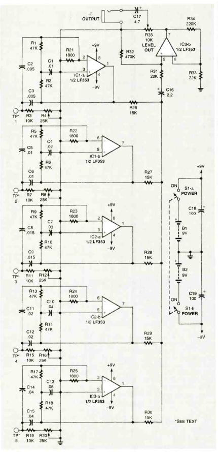
Fig. 5. This electronic bongo produces the sound of practically any percussion instrument. Adding more oscillator circuits will give you the sound of your own orchestra.
