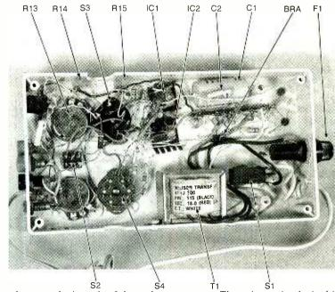
Shown here are the innards of the authors prototype. The unit was hard-wired into its plastic enclosure and the components interconnected with hookup wire. Note that the two trimmer potentiometers (R14 and R15) were glued to the inside wall of the enclosure and connected to the other components using point-to-point wiring techniques.
