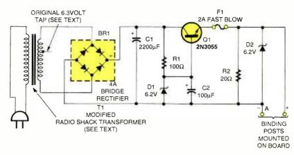
Fig. 1. Schematic of the "A" power unit with parts values noted,
