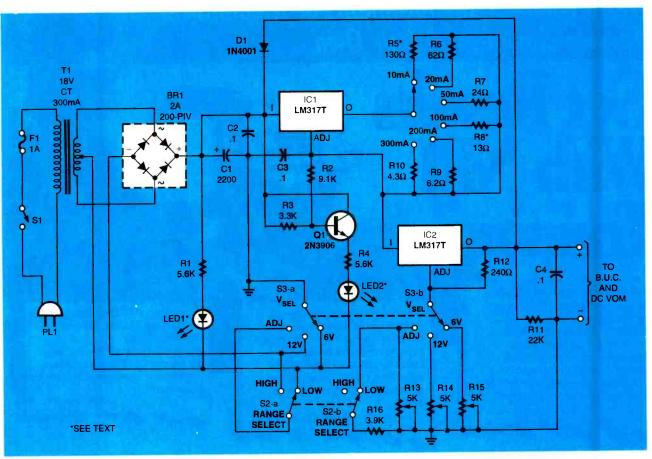
Fig. 1. At the heart of this charger are a pair of LM317T adjustable voltage regulators (IC1 and IC2)—one arranged in a current limiting configuration and the other set up as a simple variable voltage regulator—and fairly a straightforward switching network. Although the circuit is designed as a battery charger, it can also be used as a low-power supply.
