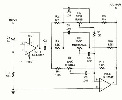
*Fig. 4. Here's a simple one-chip equalizer that furnishes bass, midrange, and treble control to an* **60** *audio input.*
