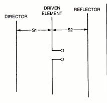
Fig. 2. Three-element Yagi beam antenna
