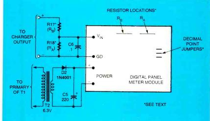
Fig. 2. Although Charge-It is equipped with tip jacks that allow you to plug meter probes into the circuit's output, you may want to go with a permanently connected voltmeter. Here we show you how to connect a low-priced digital panel meter to the circuit.
