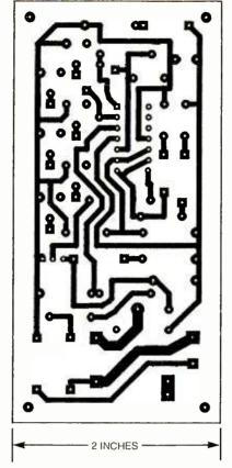
Fig. 2. Although the Fusesaver is simple enough to build using point to point wiring, the bulk of the author's unit was assembled on a printed-circuit board that measures 2 by 4 inches. A template for that printed-circuit pattern is shown here full size.
