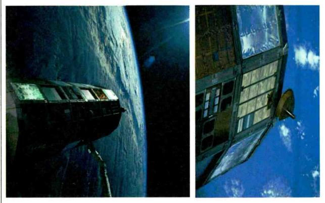
Launched in 1984 and recovered by a 1990 shuttle mission, NASA's Long-Duration Exposure Facility (LDEF) gave scientists a lot of information about how materials such as aluminum, fiberglass, composites, glass laminates, ceramic, paints, polymers, thermal insulation, etc., hold up in the harsh "weather" of low-orbit space.
