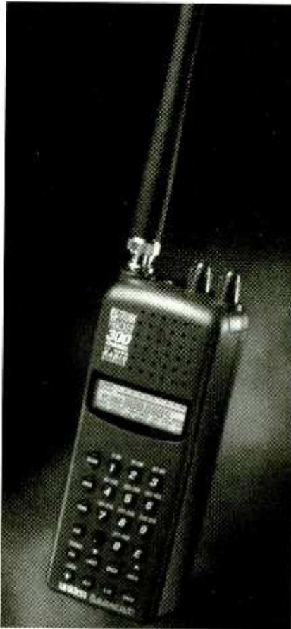
Uniden's revolutionary Trunk Tracker can actually follow trunked conversations as they jump from frequency to frequency.
