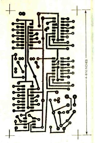
Fig. 3. The display portion of the Solid-State LED Oscilloscope is comprised of twelve 5×7 LED arrays mounted to a section of perfboard to form a 20×20 LED d<mark>is</mark>play matrix. The layout for that matrix is shown here.
