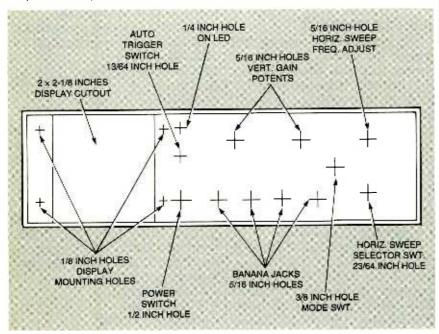
Fig. 6. The author's unit was housed in a standard bench-style instrument case, measuring  $2^{-1}/_2$  inches high,  $8^{-1}/_2$  inches wide, and 6 inches deep. If you choose a similar enclosure for your unit, the template shown here can be used to help layout your front panel. After making the appropriate alterations to the front panel, it can be painted and labeled with dry transfer lettering, and then given a final spray coat of clear plastic to protect the labels.
