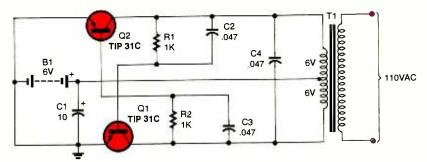
Fig. 4. The inverter circuit pushes and pulls its output through the secondary winding of a 12-volt center-tapped power transformer.
