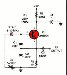
Fig. 4. The Colpits crystal-controlled oscillator uses a tapped capacitor (C1 and C2) to determine the feed back ratio that maintains oscillation. Compare this circuit to the Hartley tapped-coil, oscillator circuit.
