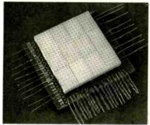
Twelve 5×7 LED arrays were mounted on a section of perfboard in a 3 by 4 configuration, as shown here, to form the oscilloscope's 20×20 display matrix.
