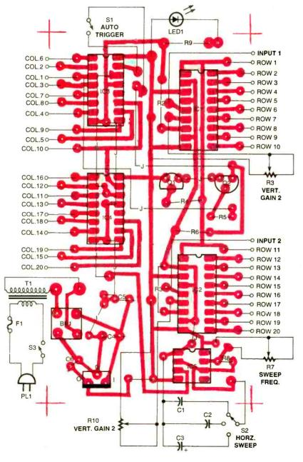
Fig. 4. The control circuits for the Solid-State LED Oscilloscope were assembled on a small printed circuit board, measuring 4-9/16 inches by 2-1/2 inches. This template can be copied and used to etch your own printed circuit board.
