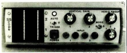
Shown here is the author's prototype unit. The front panel holds all the off-board components—the vertical gain and horizontal sweep potentiometers, as well as the input jacks, home-brewed  $20\times20$  LED matrix display, and sweep frequency selector and power switches—except the fuse.
