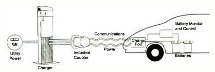
This diagram shows how inductive charging systems work. The Magne Charge system in particular can handle power levels from 1.5 to 25 kW.
