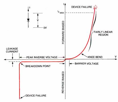
Fig. 1. Here's the characteristic curve of the current through a standard diode vs. the voltage applied across it.
