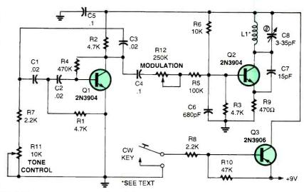
Fig. 3. This low-power, tone-modulated FM transmitter can be used with any FM broadcast receiver for real wireless code practice.
