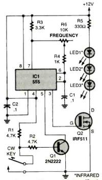
Fig. 5. Here's a CPO that transmits on IR using LED1-LED3.
