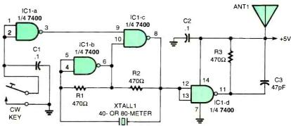
Fig. 4. Using a simple crystal-controlled oscillator, this CPO transmits on the ham bands.
