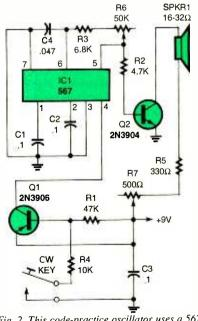
Fig. 2. This code-practice oscillator uses a 567 phase-locked loop, ICI, as its variable tone generator.
