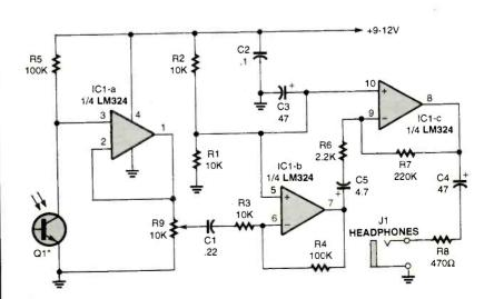
Fig. 6. This IR receiver works with the transmitter in Fig. 5.
