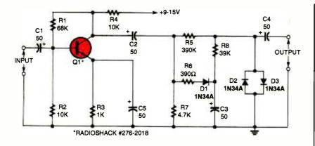
Fig. 3. Here's a compression-type amplifier that can be used to keep the volume level of an organ constant.
