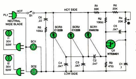
Fig. 2. Here's the schematic for the Lighting System. Lamps II and I2 plug into AC sockets SO1 and SO2, providing two efficient sources of light.
