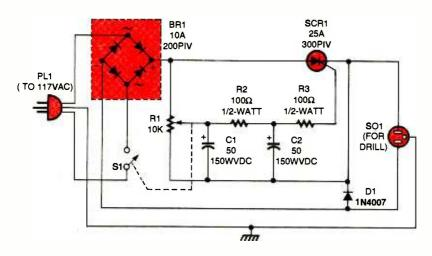
Fig. 5. Add this circuit to a single-speed drill to make it a variable-speed one.
