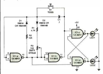
Fig. 7. Here's a simple CMOS coin-toss circuit. Make sure to adjust R3 to a 50% duty cycle.
