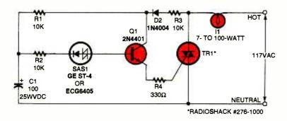
Fig. 4. With the component values shown, this flasher circuit has a rate of approximately once per second.
