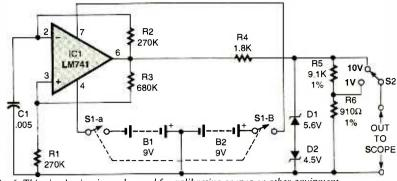
Fig. 6. This simple circuit can be used for calibrating scopes or other equipment.
