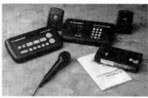
The Thumbs Up 2000 video editor allows you to instantly cut or move scenes anywhere you want in your video production using just two main controls. The large button marked with a thumbs up symbol is used to mark the scenes you want to keep; the thumbs-down button marks those you want to delete. The video editor then assembles all the scenes you want to keep and records them on a blank
