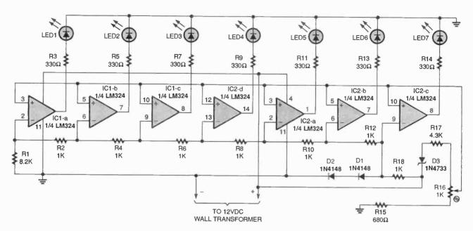
Fig. 1. Here is the schematic for the AC Line-Voltage Monitor circuit. A wall transformer steps down the line voltage and converts it to 12-volts DC to supply the circuit with both power and a small-scale indicator of how the voltage fluctuates.
