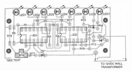
Fig. 4. Use this parts-placement diagram when assembling the circuit on a PC board. Some of the resistors have to be mounted vertically depending on space provided.
