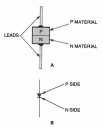
Fig. 1. A diode consists of one junction; its structure is shown in A and its schematic symbol is shown in B.
