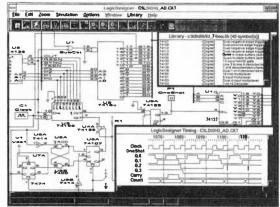
Automatic Glitch detection warns of potential circuit problems.
