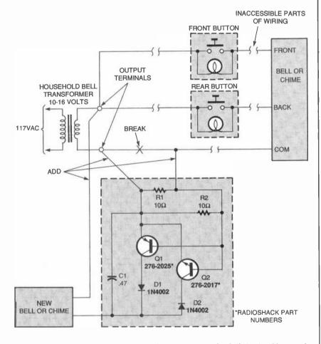
Fig. 7. With this circuit, you can add a remote bell to an existing doorbell circuit, without tearing ont walls to access the wiring between the door button and chime.
