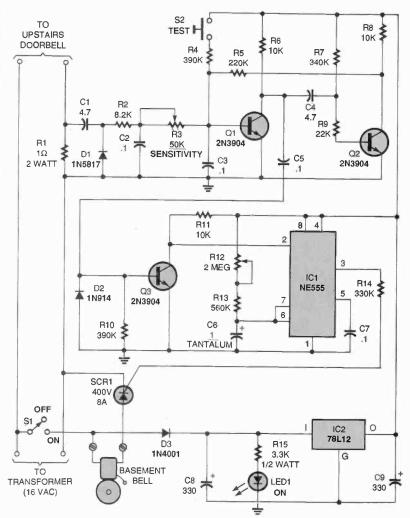
Fig. 5. Hear your doorhell in the basement with this circuit.
