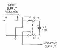
Fig. 2. Move SI from the position shown here to the other one, and you'll have a negative voltage supply.
