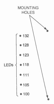
Fig. 3. This drill guide matches the positions of the LEDs and the hardware mounting holes on the PC board. Preparing the cover for the Monitor's enclosure should now be simple.
