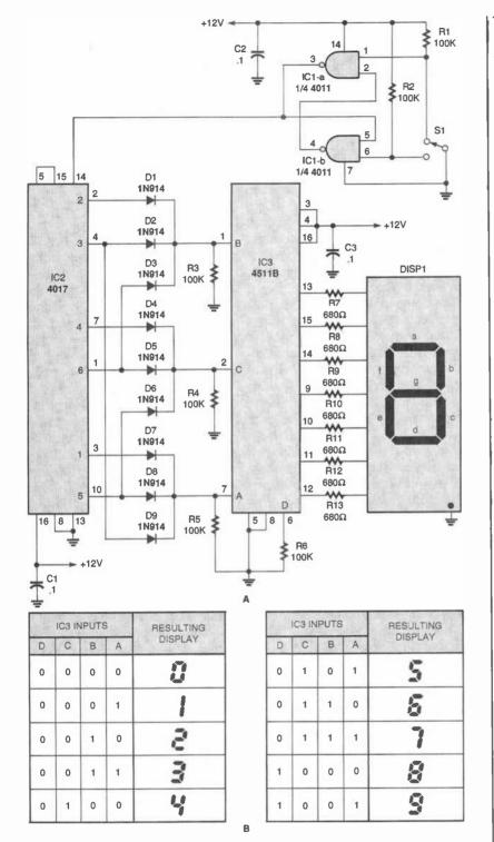
Fig. 6. This sequential stepper and driver (A) uses a seven-segment LED display, DISP1, to show the step position. Follow the truth table (B) for input data.
