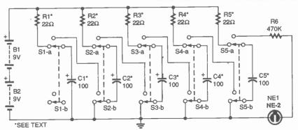
Fig. 3. With this circuit, you can turn 18 volts into 90 volts, which is enough to power neon-lamp NE1.
