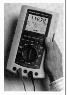
Several innovative technologies were used in the Model 867B's display, including blue LEDs from Nichia of Japan. The color is a broadband, sky blue that is converted to white backlight by means of an amber filter. Coupled with Hitachi's transmissive LCDs, the backlight technology provides higher contrast and a signification of the plant of contrast and a significantly brighter image than other display modes—while using less than half the power of back-
