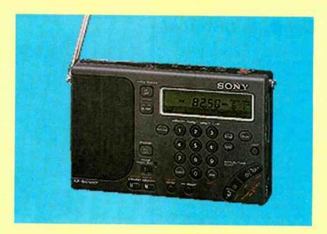
The ICF-SW1000T has two timer settings, so that you can record two different shows. The tape deck is auto-reversing, so you should be able to record up to 90 minutes of programming unattended.
