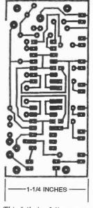
Fig. 2. This full-size foil pattern can be used to make your own PC board.
