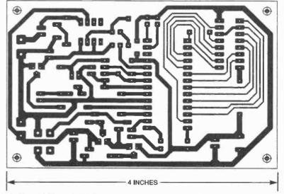
Fig. 2. If you'd like to build the Parrot on a PC board, use this foil pattern as a guide.
