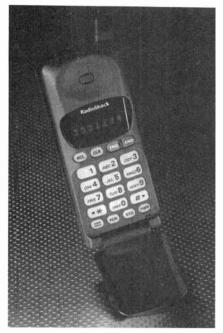
RadioShack's CT-500 is a handheld, flip-style cellular phone that can be set to vibrate instead of ring when a call is received. It can also be placed in "silent mode," where a message on the LCD will signal an incoming call. The compact phone measures 5.6×2.4×1.1 inches and weighs only 8.6 ounces
