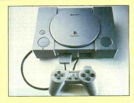
set-top box. At its heart is a 33-MHz, 32-bit RISC CPU that offers a 4-KB instruction cache and a 1-KB data cache. The CPU is backed up by a graphics processor (GPU) that provides a maximum of 16,770,000 colors and 640- × 480-dot resolution. The CPU also handles the texture mapping used in creating 3D games. In terms of audio, the PlayStation delivers CD-quality sound—and can be used to play audio CDs as well as games. The
