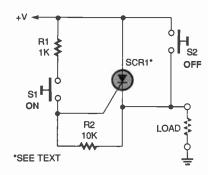
Fig. 5. This latching circuit can be used as an onloff switch with a memory.
