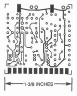
Fig. 2. This is the solder side of the Decoder circuit board.
