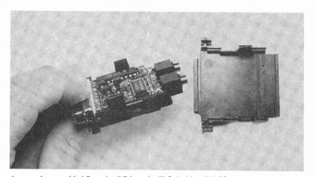
A properly assembled Decoder PC board will fit inside a DB-25 connector hood.
