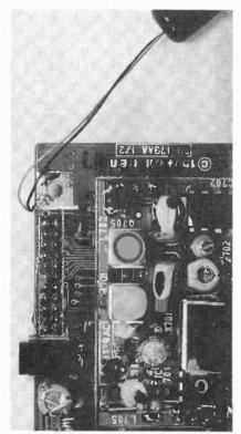
Fig. 6. This close-up shot shows you where to make the ground connection for demodulator output on a Uniden SC-150.
