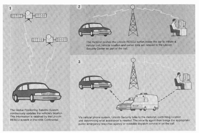
This drawing shows the three basic steps that Ford's RESCU system uses to get help to motorists.
