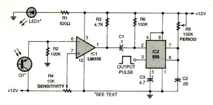
Fig. 5. Unlike the other sensors, this circuit produces an output when LED1's light is reflected from an object back to photo-transistor Q1.
