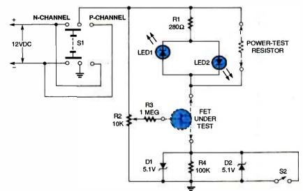
60 the pinch-off voltage is reached. The | Fig. 4. This Tester is good for all kinds of FETs and even tests power output.
