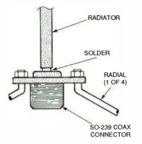
Fig. 5. Here are the base-connector details for the vertical antenna shown in Fig. 4. Only one of the four radials is detailed.
