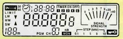
The front-panel LCD provides a very readable display of receiver functions, and includes a liquid-crystal S meter.
