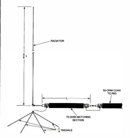
Fig. 4. You can build a  $5_{18}$ -wavelength vertical antenna like this one tonight. See text for all the details.
