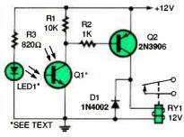
Fig. 1. Any opaque object blocking the light path between LED1 and Q1 will cause RY1 to 68 open.
