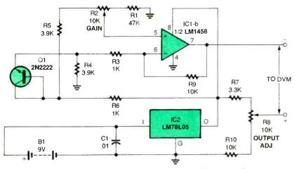
Fig. 1. Here's the schematic for the Temperature Adapter. The circuit allows your DMM to measure from -40 to +300 degrees Fahrenheit.
