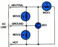
Fig. 2. If MOV2 shorts to ground, it could tie the neutral and ground lines, violating the National Electrical Code.
