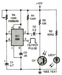
Fig. 4. The timed output pulse in this circuit will not occur until photo-transistor Q1 is unblocked.
