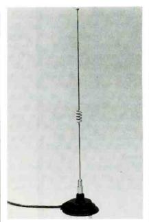
Fig. 2. Magnet-mount mobile antennas like this one grab the metal surface of your car's roof or trunk. Interconnecting coax-cable is usually long enough for most sedan models.
