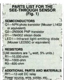
infrared emitter LED (LED1) is aimed at an infrared photo transistor (Q1). As long as the IR light path remains uninterrupted between the two, transistor Q2 will keep relay RY1 closed. Any opaque object blocking the light path will cause RY1 to open.
