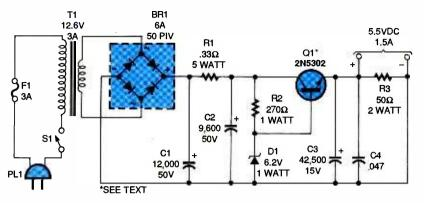
Fig. 3. This antique-radio power supply has filtering sufficent enough to make it as stable as a car battery.
