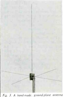
Fig. 3. A hand-made. ground-plane antenno costs only pennies to build.
