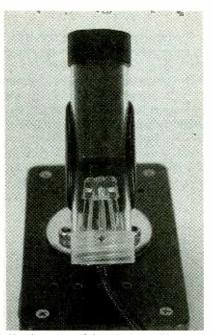
Here's a view of the tube assembly, showing how the four LEDs are mounted.
