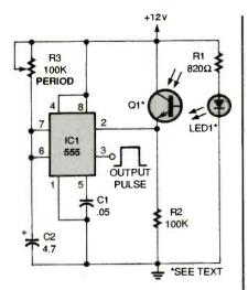
Fig. 3. This IR sensor, with a timed positive-output pulse, will operate with older and slower PLCs.
