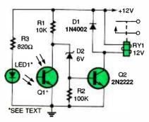
Fig. 2. In this circuit, RY1 remains open until the light path between LED1 and Q1 is blocked.
