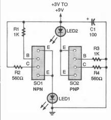
Fig. 4. When a good T092 transistor is placed in the carrect socket of this tester, the circuit turns on according to the kind of transistor being tested.
