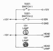
Fig. 4. This simple test setup will let you determine if your DRL circuit is working before you install the latter in your vehicle.
