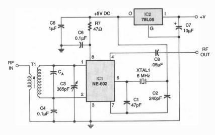
Fig. 2. This converter circuit, built around an NE-602, will translate WWV's 10-MHz signal to the 75-meter ham band.
