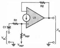
Fig. 5. Here is a noninverting follower built around a current-difference amplifier.
