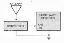
Fig. 1. Here's how an external frequency converter is hooked up to a typical communications
