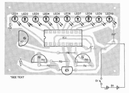
Fig. 3. If you're building the Thermometer circuit on a PC board, use this partsplacement diagram as a guide.
