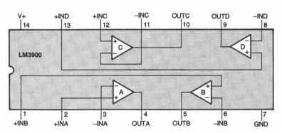
Fig. 3. Here's the pin out of a common current-difference amplifier IC, the LM3900.
