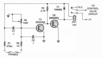
Fig. 3. This circuit builds upon the principles used in the circuit of Fig. 1 to provide automatic operation of a watering system when a dry-soil condition is detected.
