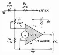
Fig. 9. This variable-voltage source can provide between 0.6 to 20 volts, depending on the setting of R1.
