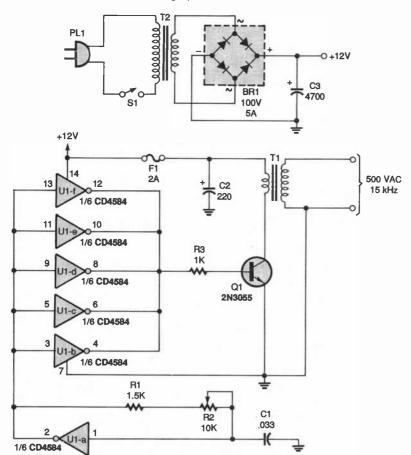
Fig. 1. Here's the schematic for the High-Voltage Power Supply. A 15-kHz pulse, generated by U1, drives switching-transformer Q1. Transformer T1 then steps up the generated AC to 500 volts.
