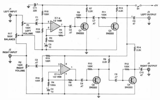
Fig. 5. This stereo amp can be used with a Walkman or portable CD player, and a pair of speakers, to provide a room-full of sound.
