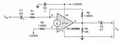
Fig. 8. Here is a practical 20-dB gain AC amplifier built using the LM3900 CDA.
