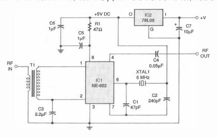
Fig. 3. This circuit is similar to the WWV converter shown in Fig. 2, except that it is used to translate VLF signals to the 6000-kHz region.
