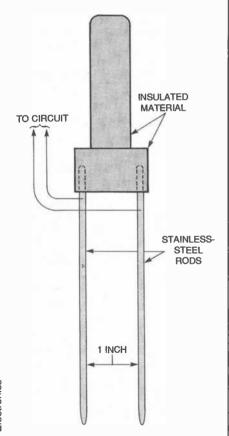
Fig. 2. This probe assembly can be used with the circuit in Fig.1, as well as other circuits in this month's column. While some dimensions are specified, they are not critical so feel free to use whatever is handy.
