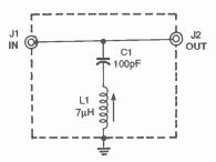
Fig. 4. If your receiver is "desensitized" by the converter's local oscillator, this 6.000-MHz wavetrap could help minimize the problem.
