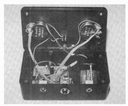
This internal view of the author's prototype shows how it was built on a universal assembly board.
