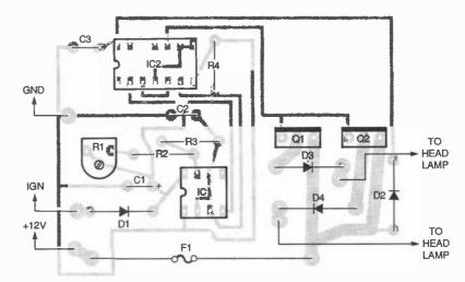
Fig. 3. Use this parts-placement diagram as a guide when assembling the PC board, and when connecting it to your vehicle.
