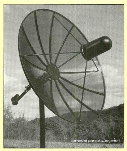
the wind. When we installed the feedhorn, only minor adjustments were required to get the feed to the 31¾-inch focal point of the dish.
