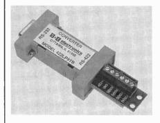
All of the converters are powered from the RS-232 handshake line's DTR and RTS (one must be high). The continued on page 16
