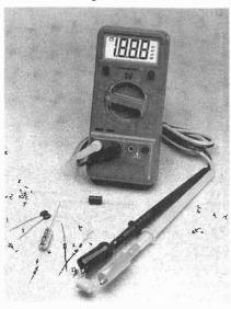
resolution in the 20-ohm range. The meter features a capacitance zeroadjust button to compensate for testlead and stray capacitance. The 20-ohm range, typically found only in expensive, bench-quality meters, also features the zero-adjust button to compensate for test-lead resistance. The CR50 also includes a beeper for fast and convenient continuity measurement, and a diode test.
