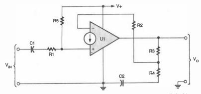
Fig. 6. In applications where larger than normal voltage gains are needed, this super gain CDA-based amplifier can be used.
