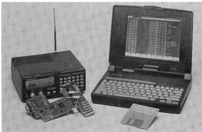
A Radio Shack Pro-2005 scanner equipped with an Optoelectronics OptoScan 456 computer-controlled interface, a PC, and the appropriate software, all form a complete computer-aided VHF/UHF scanning system.
