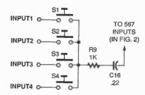
Fig. 3. This circuit illustrates the theory behind the routing system used in the cable tester's receiver.
