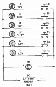
Fig 6. Though deceptively simple, this buttery tester can help you weed out marginal cells that might otherwise test good.
