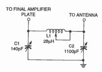
Fig. 2. In a pi-network, the output capacitor (C2) is typically a 1100-pF, three-section, broadcast variable with relatively wide spacing,
