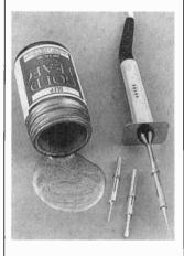
The tips are available in interchangeable slide-on needlepoint, chisel, and spade shapes. They have no threads to bind or screws to freeze.
