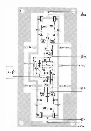
Fig. 5. When assembling the Amplifier board, use this partsplacement diagram as a guide. Watch the polarity of those offboard jack connections!
