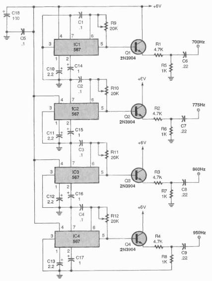
Fig. 1. Here's the transmitter for our cable-tester system. The circuit generates four distinct audio tones that are available at the output as shown.
