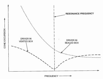
Fig. 3. At lower frequencies, the cone excursion is significantly lower in a vented-box (bass-reflex) system.
