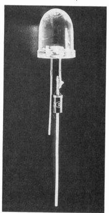
Fig. 2. Solder the LED and diode together, as shown here, so that the overall length of the soldered leads is 3/8 inch
