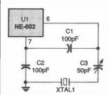
Fig. 2. Here, a variable capacitor is added to the circuit of Fig. 1 to make it easier to obtain the desired frequency.
