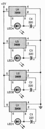
Fig. 5. Using LED's and 3909 IC's, you can make a flashing-light circuit that runs for months on two AA batteries.
