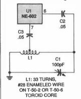
Fig. 6. In this Hartley VFO, feedback is provided via a tap on the inductor.
