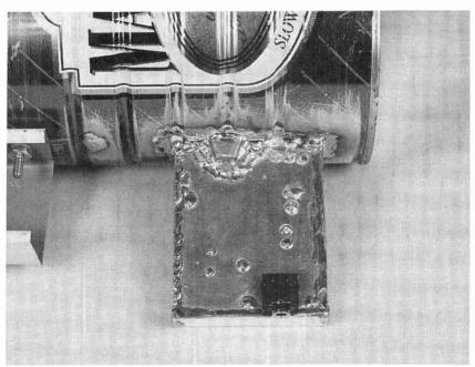
Center the oscillator-board antenna in the 4-inch hole, 17% inches from the closed end of the can, and solder it to the can assembly, completely filling the gap with solder.
