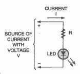
Fig. 1. Perhaps the most common use of a resistor is as a current limiter. Here one is shown keeping the current (1) produced by the voltage (V) to a safe value for LED1.
