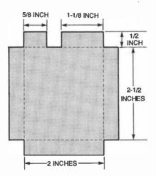
Fig. 7. This is the template for the tin shield that covers the oscillator board. The sides of the shield are bent up at 90-degree angles (where dotted lines are shown) to form a cover. The opening is for the antenna.
