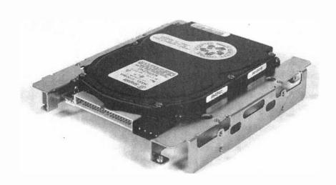
A mounting kit adapts the hard drive to fit in a 51/4-inch drive bay.
