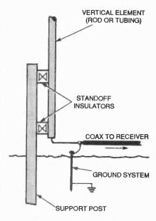
Fig. 3. Verticals take up little real estate and give good results. With a vertical, you connect the center conductor of the coax transmission line to the vertical portion and the coax shield to ground. Note that a good RF ground is important.
