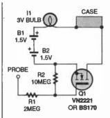
Fig. 3. Apparently, this circuit is a favorite of more than one reader. It has appeared in this magazine twice already! Note that the BS170 used in the original version is easier to find than the VN2221.
