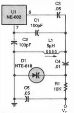
Fig. 7. You can use a varactor diode (DI) to tune a VFO circuit electronically. This figure shows a parallel-resonant, voltage-tuned Colpitts oscillator.
