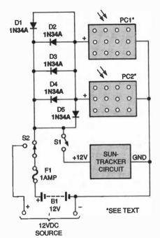
Fig. 2. This application circuit provides rechargable solar power for the Sun Tracker, as well as for another 12-volt device.
