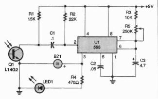
Fig. 2. With this audible tester, you can see and hear if your remote is transmitting or not.
