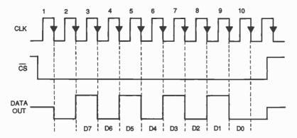
Fig. 2. Here's the timing diagram of the ADC0831. In the application discussed in the article, the CLK signal is derived from a PC's parallel port, and the Data Out is sent to the same parallel port.
