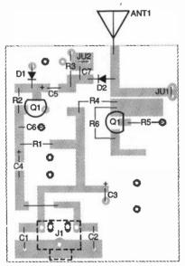
Fig. 6. Careful soldering and the shortest possible lead lengths are important on the microwave-oscillator board. Any lead shown mounted over a circular pad goes through the board and is soldered on both sides, and all other leads are tack soldered on the surface. Note that JI mounts on the solder side.
