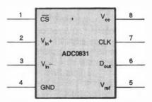
Fig. 1. This is the pinout of the ADC083I, which is the heart of the A/D Converter.
