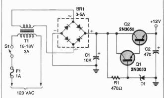
Fig. 7. Here's a 12-volt power supply that is easy-to-build while producing a smooth output.
