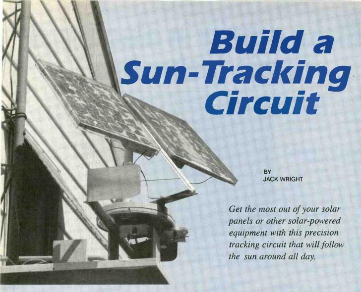
ere Is a circuit which, with your own drive creation, will track the sun with an accuracy of better than half a degree. It is called the *Sun Tracker*, and you can use It to direct a payload of solar (photovoltaic) modules, or to track the sun for other purposes, such as measuring ultraviolet intensity.
