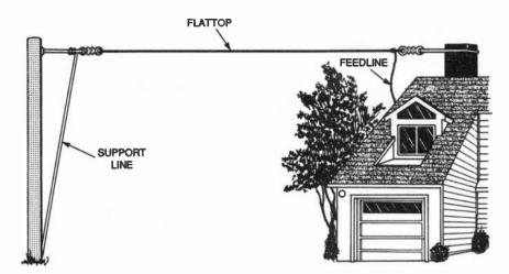
Fig. 1. A random length of wire is the simplest of horizontal antennas. You can use practically any length of wire, even a very short one, but lengths between 25 and 100 feet and strung as high and in the clear as possible work best.
