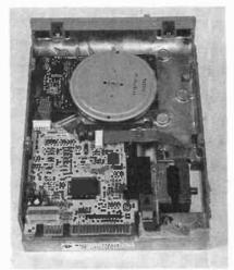
A 5%-inch drive has a 34-pin card-edge connector on the back end along with one or more power connectors.
