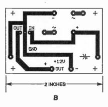
Fig. 2. A helpful reader was so happy with the freeze-sensor circuit, he's provided us with foil patterns for it (A) and the power supply he uses (B).
