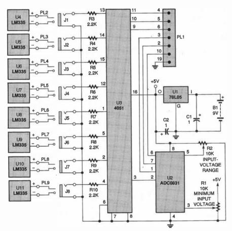
Fig. 5. The actual processing circuitry of this AID Converter consists of only four parts: U2, U3, R1, and R2. As you can see, eight temperature probes are used with the circuit; however, they can be replaced with other types of sensors, as long as resistors R3-R10 are removed.
