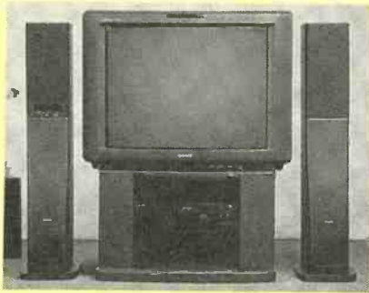
Sony's SA-VA1 home-theater speaker system, shown here with a 32-inch TV, features two front tower speakers that include a Dolby Pro Logic decoder, amplifiers, subwoofers, and inward-firing center-channel drivers. Two rear surround-sound speakers complete the system.
