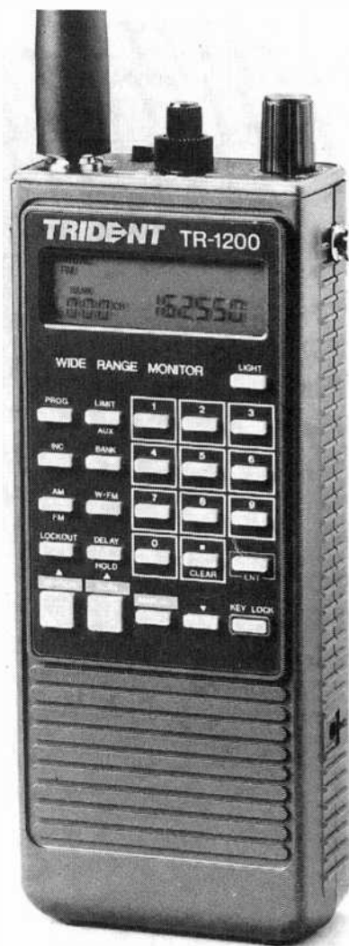
The handheld Trident TR-1200 offers a very wide tuning range and 1000 memory channels.
