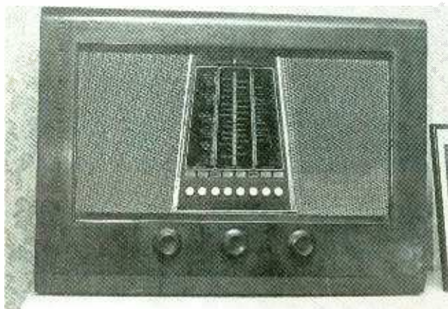
The Bush 22 Series boasts pushbutton tuning, and an imposing three-scale dial.
