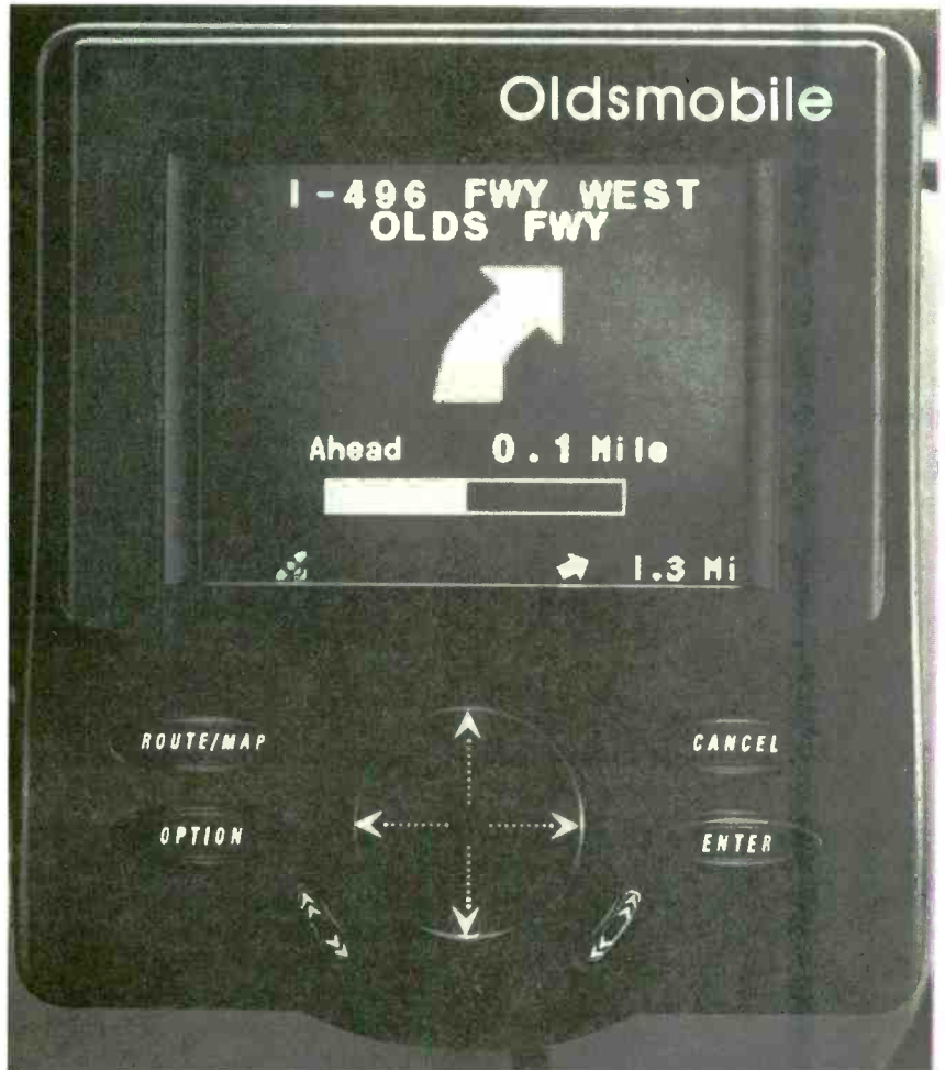
"Turn-by-turn" route guidance provided by simple arrows is augmented by synthesized-voice instructions. The screen also shows the distance to the next required maneuver as well as the direction and distance to the final destination. (Photo courtesy of Oldsmobile.)
