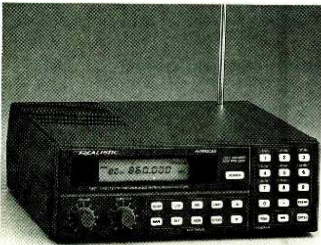
This handsome desktop scanner from Radio Shack, the PRO-2030, allows users to search and scan in quick (50-channel-per-second) Hyperscan mode, or at a more leisurely 12 channels per second.
