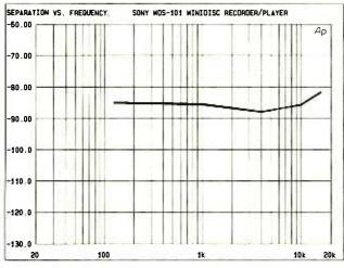
Stereo separation was above 80 dB even at the highest test frequency of 16 kHz.
