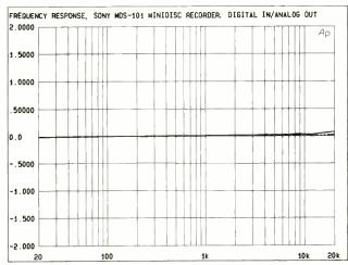
When the optical (digital) inputs were used, frequency response was again virtually flat, but the output levels for both channels was nearly identical.
