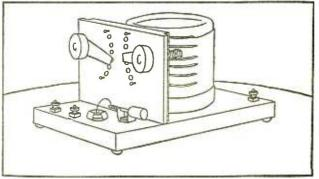
This is a general view of the NBS crystal set. The cylindrical object in back of the panel is the 76-turn tuning coil.
