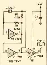
Fig. 3. In this circuit, three inverters along with XTAL1 are used to form an oscillator circuit capable of operating at up to 10 MHz.
