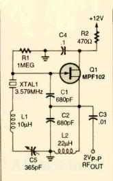
Fig. 4. This FET-based crystal oscillator, known in the ham community as a VXO (variable crystal oscillator), can be made to shift the crystal's frequency slightly to achieve a more exact frequency.
