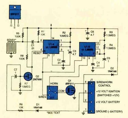
Fig. 1. At the heart of the Motorcycle Alarm is a LM556 dual oscillator/timer, a pair of FET's, and a rather unusual sensing unit (SENSI)—which is comprised of adjacent circuit board traces and a small stainless-steel ball bearing.
