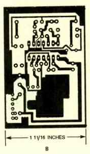
Fig. 2. The Motorcycle Alarm was assembled on a small double-sided, printed-circuit board, measuring about 2 by 11/16 inches: A is the template for the component side, and B is the solder side. The board can be ordered from the supplier given in the Parts List.
