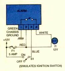
Fig. 4. In this simple test set-up, a 12-volt lamp is used in place of the horn.
