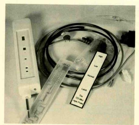
The logic-probe kit comes with everything that you'll need to put together a professional-looking probe, including the case and front-panel decal.
