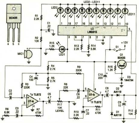
Fig. 4. This volume meter can be handy anywhere you need to measure the relative sound level in a room. It is readily adjustable to increase its usefulness.
