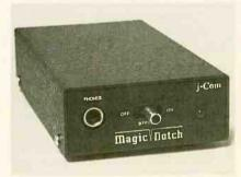
The MagicNotch interference filter is an automatic notch filter that requires no tuning or user intervention. When it detects a heterodyne signal, it immediately filters it out using a sharp rejection filter. Audio of other frequencies, such as speech, is passed through without attenuation.
