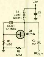
Fig. 2. The unijunction oscillator shown here allows higher frequency operation, and like the previous circuit, uses a quartz crystal (XTALI) to set its operating frequency.
