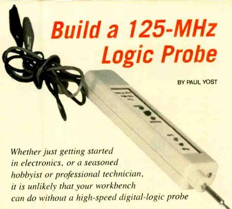
and trace their paths. The simplest way to do that is by using a logic probe. A logic probe is a device that allows the technician a fast and convenient way to "look inside" a digital circuit and see exactly which paths are high, which are low, and which are pulsed.
