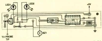
Fig. 4. Whether choose to purchase a kit or "roll your own," once you have all of the parts, you need only install the parts in the positions and with the orientations shown in rhis parts-placement diagram.
