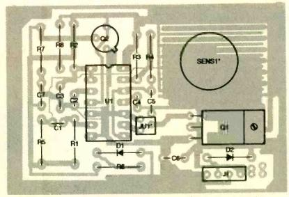
Fig. 3. Here are the proper locations and orientation of the various parts that comprise the Motorcycle Alarm. When assembling the board, watch out for the polarities of C3 and C6.
