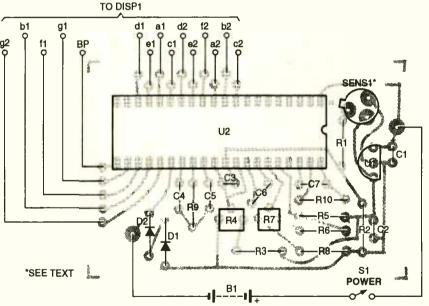
Fig. 4. When assembling the senor board be sure that all of the polarized components are correctly oriented and installed in their proper locations.
