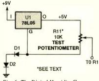
Fig. 6. The Digital Humidity Gauge can be calibrated using two procedures. The first is a two-point method, outlined in this diagram. It requires a potentiometer and digital voltmeter to set R4 and R7. (See the text for more details.)
