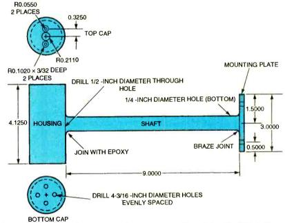
Fig. 5. The generator housing was fabricated from a 4½-inch length of 1½-inch diameter PVC pipe, a ½-inch length of electrical conduit, a  $1-\times 3-\times 4$ -inch strap, and two 1½-inch PVC end caps.
