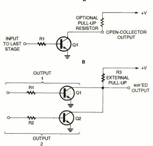
Fig. 1. These are crude representations of logic-IC outputs. In A a totem-pole output is depicted. In B we show an open-collector output. In C we show how two open-collector outputs can be NOR ed together.
