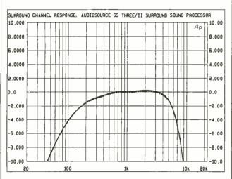
Fig. 3. The response curve for the surround channels (shown here) was obtained by feeding out-of-phase left and right signals to the line inputs of the SS Three/II.
