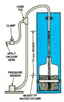
Fig. 7. For those who wish to obtain the greatest possible accuracy from the circuit, this set up can be used to calibrate the Digital Barometer using a procedure founded in some basic laws of physics.
