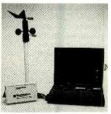
and accessed by other real-time DOS programs. An alarm function sounds the audible annunciator in the computer whenever the peak wind speed exceeds the value set by the user. An optional relay can also activate an external device whenever the wind speed alarm limit is exceeded.
