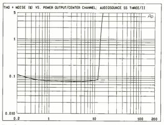
Fig. 5. The actual continuous power rating of each of the amplifier channels was about 12 or 13 watts; above those levels, overload and high distortion levels occur. Below that output level, total harmonic distortion was a comfortably low 0.08%, or even a bit lower.
