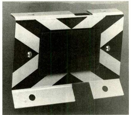
This is the forward Forewarn radar transmitter/receiver, which mounts on the front of a school bus. It warns drivers of children that are out of sight, under the hood line.
