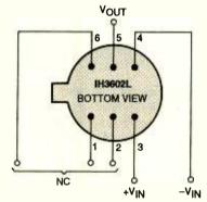
Fig. 7. The Hy-Cal IH3602L sensor, SENSI (a 6-pin CMOS device with only 3-active terminals), is at the heart of the humidity measurement system. The IH3602L provides a DC output voltage that varies linearly with relative humidity levels from 0 to 100%.
