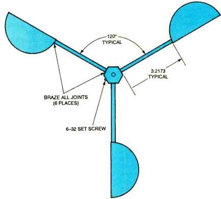
Fig. 4. Three rotor spindles were fabricated from 3½-inch lengths of straight ¼-inch diameter peg board hanger, and the wind cups were fabricated from 2½-inch diameter soup ladles.
