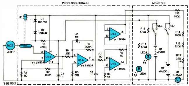
Fig. 2. The anemometer is comprised of the generator (denoted MOTI), an LM324 quad op-amp (UI, whose four op-amps form a preamp, an integrator, and buffer); a pair of light-emitting diodes (LEDI and LED2, which are used to monitor battery voltage), an ammeter (MI), and a few support components.
