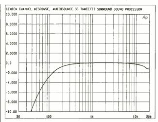
Fig. 2. The low-frequency roll-off of the center channel is deliberate, and is prescribed by the Dolby Surround system. The center channel deals essentially with spoken dialogue, so ultralow frequency response is not required.
