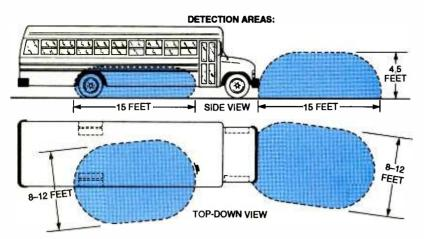
Fig. 1. Shown here are the detection areas monitored by the Forewarn two-sensor system. Note the protection corridor on the curb side of the bus.
