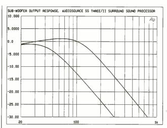
Fig. 4. This plot shows the response available at the subwoofer line-level output jack. Note that two crossover frequencies (80 and 150 Hz) are available, and the response for each is shown.
