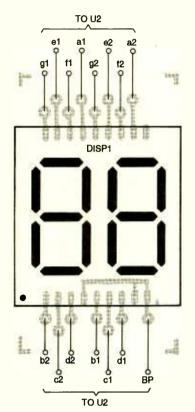
Fig. 5. The display board (as shown by this parts-placement diagram) holds only one component, the LCD readout. Although, from appearances it may seem difficult to assemble this board the wrong way, looks can be very deceiving, so make absolutely sure that the readout is properly oriented on the board.
