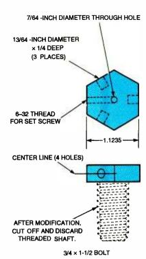
Fig. 3. The rotor hub was fabricated from a <sup>3</sup>/<sub>4</sub>-inch × l<sup>1</sup>/<sub>2</sub>-inch bolt head. The bolt head was drilled (as shown in this diagram) and shaft of the bolt was cut off. The bolt head was retained as the rotor hub and the shaft was discarded.
