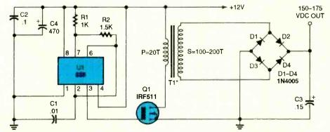
Fig. 6. In this DC-to-DC converter, the 555 is used to produce a rising and collapsing field in Tl's primary, generating a higher voltage in Tl's secondary winding. That voltage is then fullwave, bridge rectified by D1-D4, and filtered by C3.
