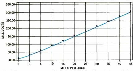
Fig. 1. The generator/rotor assembly was mounted on top of the author's van, which was driven at speeds ranging from 5 to 45 miles per hour (mph) in 5-mph increments on a windless evening. The generator's output voltages—measured at various vehicle velocities, using a high-impedance voltmeter—were recorded, and the data was used to develop this graph.
