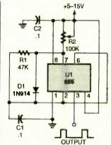
Fig. 2. At the instant that power is applied to the 555 astable, timing capacitor CI is initially discharged, causing the output of the chip output at pin 3 to be high. Once CI has charged to about ½ of the supply voltage, its output goes low, and the discharge transistor turns on, draining the charge on CI.
