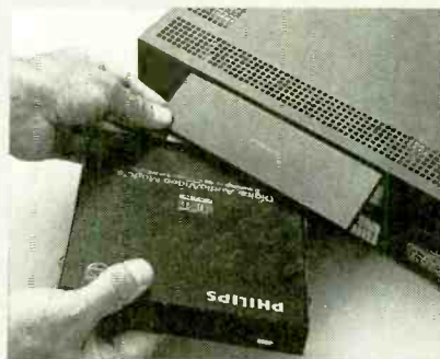
With the addition of a plug-in adaptor cartridge, Philips CD-I player is updated to provide full-motion video and extra memory storage.
