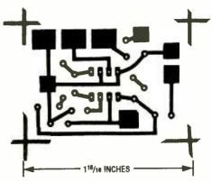
Fig. 2. The author's prototype was assembled on a printed-circuit board, measuring about 13/8 by 115/16 inches. A template of the printed-circuit layout is shown here.
