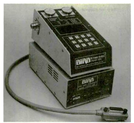
Shown here is the Bird Model 4391 Power Analyst, a high-accuracy and expensive buscompatible digital-display RF-power and SWR meter. It is best suited for commercial and laboratory installations and those amateurs who insist on professional-quality instrumentation.
