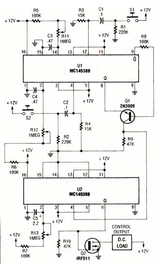
Fig. 5. The timed safety circuit, built around a pair of MC14538B dual retriggerable monostable multivibrators, makes SI and S2 individually adjustable.
