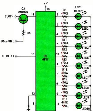
Fig. 4. If you prefer, the circuit of Fig. 3 can drive a discrete LED display.
