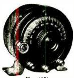
The remarkable degree of precision in adjustment of this condenser is obtained through the extreme smoothness of operation together with a friction type of Vernier. An accurately ground steel shaft and self-aligning bronze cone bearings are used.
