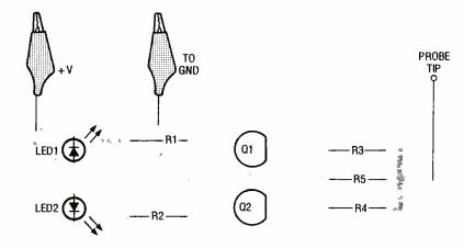
Fig. 5. Assemble the Digital Logic Probe using this parts-placement diagram as a guide. Once complete, the board can be housed in an enclosure just like the one used for the Continuity Tester (see text for details).
