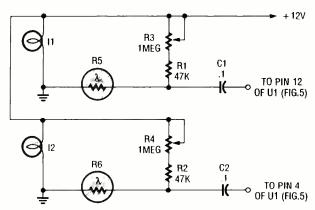
Fig. 6. This circuit, which is built around two cadmium-sulfide light-dependent resistors and a pair of lamps, is designed to replace the mechanical switches in safety control systems.
