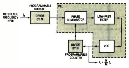
Fig. 3. The PLL can be used to generate new frequencies from a stable reference source by either frequency multiplication and division, or transition.
