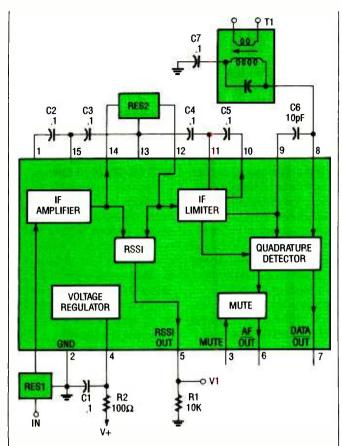
Fig. 2. The primary winding of a 455-kHz IF transformer (T1) serves as the phase coil needed by the NE604 FM/IF subsystem's the quadrature detector.
