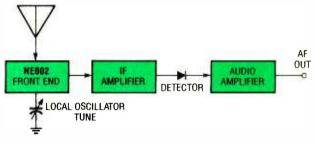
Fig. 1. The minimalist superhet-receiver system suggested by this functional-block diagram is based on a design that uses an NE602 for the front-end, and either an NE604 FM/IF subsystem or an MC1350P as the IF amplifier.
