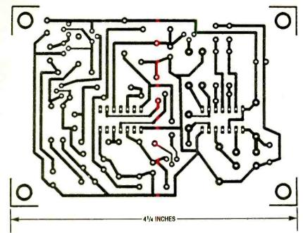
Fig. 3. The prototype of the Electronic Doorbell was assembled on a printed-circuit board measuring about 41/4 by 215/16 inches. A template of that printed-circuit pattern is shown here full size.
