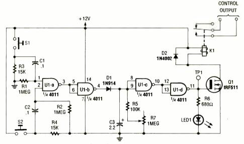
Fig. 3. The electronic safety-control is built around a 4011 quad two-input NAND gate and an IRF511 hexFET.
