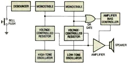
Fig. 1. Here is a functional block diagram of the Electronic Doorbell. When the doorbell switch is pressed, the two monostables stages are activated in sequence, applying bias to a pair of voltage-controlled resistor stages, which then modulate the outputs from a pair of tone generators, and the resulting signals are then fed to an audio amplifier, and then to the speaker.
