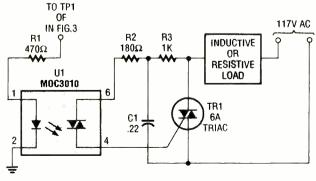
Fig. 4. The relay-replacement circuit (shown here) can be used to operate inductive or resistive loads.
