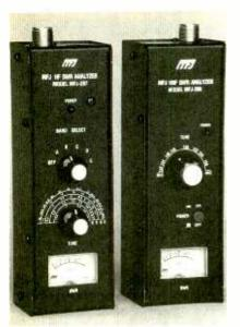
The MFJ-207 HF and MFJ-208 VHF SWR Analyzers physically resemble oldstyle dip meters, but the analyzers contain a built-in SWR bridge and RF source. When you sweep the band within which the antenna is supposed to be resonant, you get an estimate of the antenna's resonant frequency by observing the dial frequency at which the SWR dip occurs.
