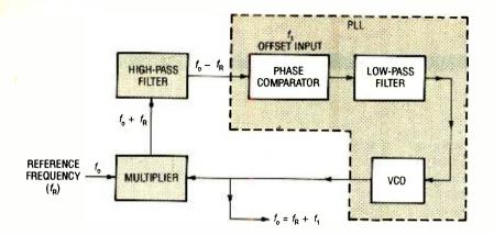
Fig. 4. By adding a multiplier and an additional low-pass filter to the PLL as shown here, it is possible to form a frequency-translation loop.
