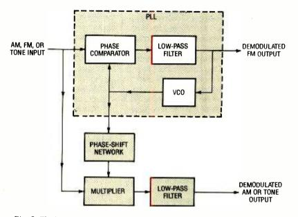
Fig. 5. The basic PLL circuit can be converted to a synchronous amplitude-modulation (AM) detector by adding a non-critical phase-shift network, an analog multiplier, and an external low-pass filter to the basic system.
