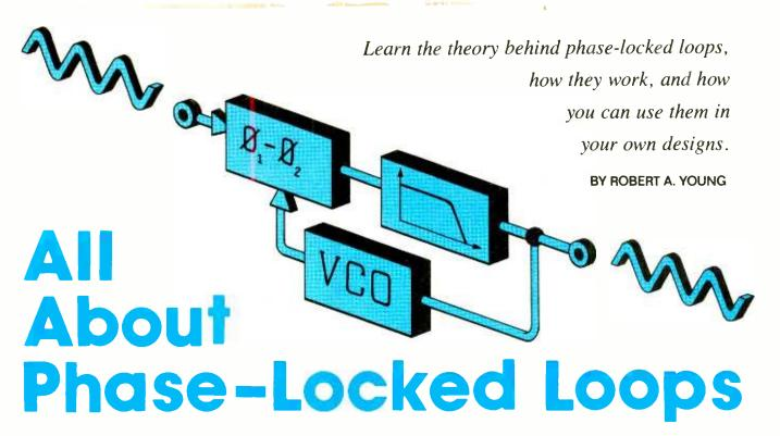
ince the phase-locked loop (PLL) was reduced to a single IC package, it has had a significant affect on electronics design. The phase-locked loop provides frequency-selective tuning and filtering without the need for colls or inductors. As shown in Fig. 1, the PLL, in its most basic form, is a feedback system comprised of three basic functional building blocks: a phase comparator, a low-pass filter, and a voltage-controlled oscillator (VCO).
