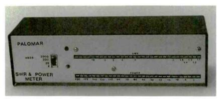
The M-835 SWR and Power Meter is an instant reading LED-display device that shows single-sideband peak-envelope RF power. The meter also computes SWR automatically and displays it on a bargraph. The unit features two 30-element, six-inch LED readouts for a reading resolution of better than 3% of full scale.
