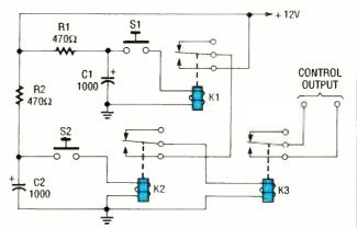
Fig. 2. This safety control switch offers an improvement over the previous on in that SI and S2 must be depressed at about the same time to power the load circuit.
