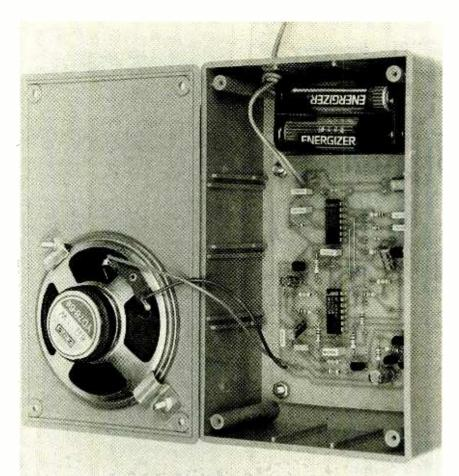
This view shows the completed electronic doorbell in the commercially available enclosure. The printed-circuit board is secured in its enclosure elevated on 5-mm tapped standoffs. Note: It may be necessary to mount the 100-µF, capacitor (C2) with its body flat against the board so that it clears the speaker.
