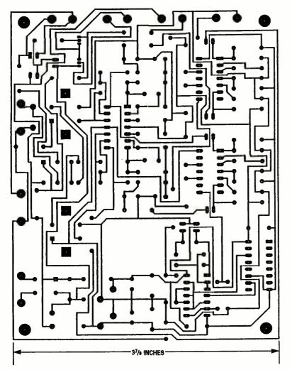
Fig. 3. This template for the Telephone Scrambler's printed-circuit board is presented for those who prefer to roll their own. However, if you are so inclined, you can purchase a prefabricated board from the supplier listed in the Parts List.
