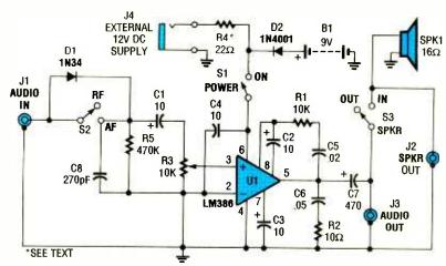
Fig. 1. The Test Bench Amplifier (which is designed as a "building block") is built around an LM386 low-voltage, audio-power amplifier (U1).
