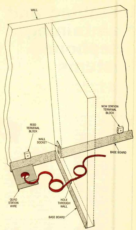
Fig. 3. When installing a new station, map out the route that the wire run is to take. If the new station is to be located in another room, which often requires that a hole be drilled through a wall, avoid (as best you can) AC receptacles.
