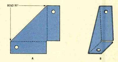
Fig. 2. For saftey reasons, it's also important that the duplex socket mounted to the rear panel of the enclosure be able to withstand power-cord insertion force without the case flexing and possibly forcing the AC wiring to contact the case or other components. To that end, reinforcing brackets fabricated from scraps of sheet aluminum were placed at one end (either end) of the outlet, although placing brackets at both ends makes for a much sturdier project.
