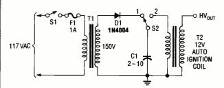
Fig. 3. The Capacitor-Discharge Driver—which is manually operated—consists of two transformers (Tl and T2), a diode (D1), a fairly large value capacitor (C1), and a SPDT switch (S2).
