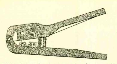
Fig. 7. This is what the crimping tool required to attach a modular plug to quad line cord looks like. To use it, simply load a plug into the tool, insert the line cord into the slot on the plug, and squeeze.
