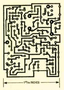
Fig. 4. The author's prototype was assembled on a printed-circuit board that measures about 115/16 by 2 inches. This full-size template of the printedcircuit artwork is provided so that you can etch your own printed-circuit board.
