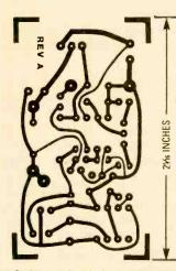
Fig. 3. Using this foil pattern to generate a printed-circuit board will make the assembly of your own current injector a snap.
