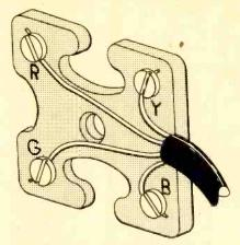
Fig. 1. Regardless of the telephone's line-cord termination, all domestic phone installations begin with the basic quad-terminal connection block like the one shown here.
