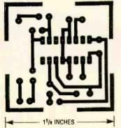
Fig. 2. The prototype of the Tel-Tale was assembled on a small printed-circuit board, measuring about 15/8 inches square, a full-size template of which is shown here.
