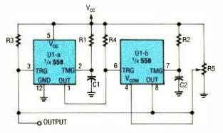
Fig. 2. By adding a potentiometer, the astable oscillator shown back in Fig. 1 can be turned into a constant duty cycle voltage-controlled oscillator with a 50-to-1 adjustment range.
