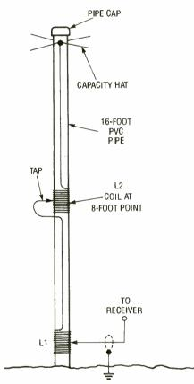
Fig. 1. A typical low- frequency antenna can be made from either a single 16- foot length or two 8-foot sections (coupled at the middle) of thick-wall PVC pipe, as shown here.
