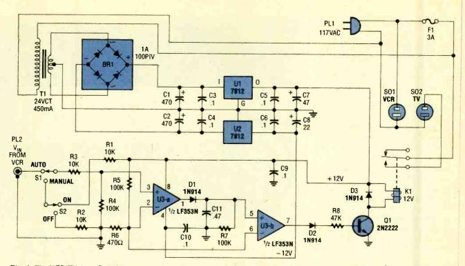
Fig. 1. The VCR/TV Auto-Switch is comprised of a 24-volt center-tapped transformer (T1), a 1-amp, 100-PIV, fullwave bridge rectifier, and two 12-volt regulators (U1 and U2), which form dual-polarity, regulated, power supply; a dual BiFET op-amp (U3) and a general-purpose NPN silicon transistor (Q1), which form the basis of a signal detector/trigger circuit; a 12-volt relay (K1); two AC sockets (SO1 and SO2); and a few additional components.
