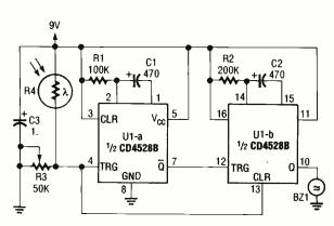
Fig. 5. Do you have someone in your house that forgets to close the refrigerator door? This may be a cure for their poor memory and your high-electric bills.
