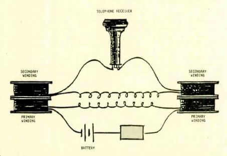
The rheotome (R) used in Hughes' induction balance to produce current pulses in the circuit's primary windings initially consisted of a mechanical interrupter, but later was changed to a ticking clock and microphone.
