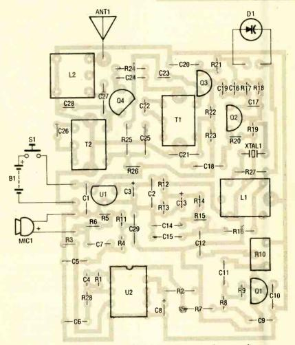
Fig. 5. Assemble the printed-circuit board using this parts-placement diagram as a guide. It is recommended that an IC socket be provided for U2. Before you begin assembling the project, however, it is important that you decide on what frequency the circuit is to operate and to select a crystal accordingly.
