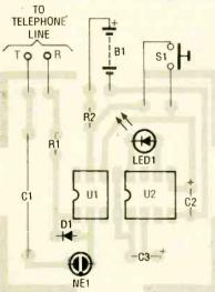
Fig. 3. Once you've etched your board and gathered all the parts listed in the Parts List, construction can begin, guided by this parts-placement diagram. In the author's prototype, a single 16-pin IC socket is used for both U1 and U2 (6and 8-pin devices, respectively).
