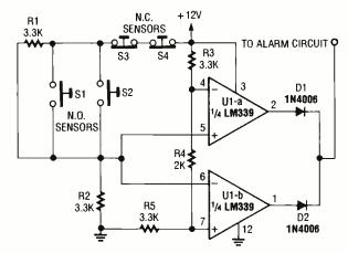
Fig. 6. This alarm actuator is a bit better than the usual alarm circuits found in this column because the wiring to the sensors is protected.
