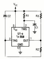
Fig. 3. A single 558 timer section can be used as an astable oscillator in a pinch. However, using this trick is only advised if the output load does not change too much.
