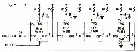
Fig. 4. This ring counter could be just the right control circuit for a sequential light display. Of course, you could add as many 558 sections to the loop as you need.
