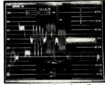
The multiburst pattern shows the acceptable frequency response performance of recorded NTSC signals.
