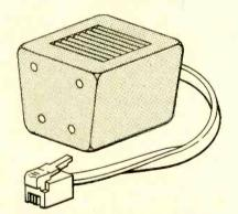
Fig. 5. The adapter in A allows you to use a modular telephone in an older plug-in system; the adapters in B and C can be used to make older plug-in telephones compatible with a modular system.
