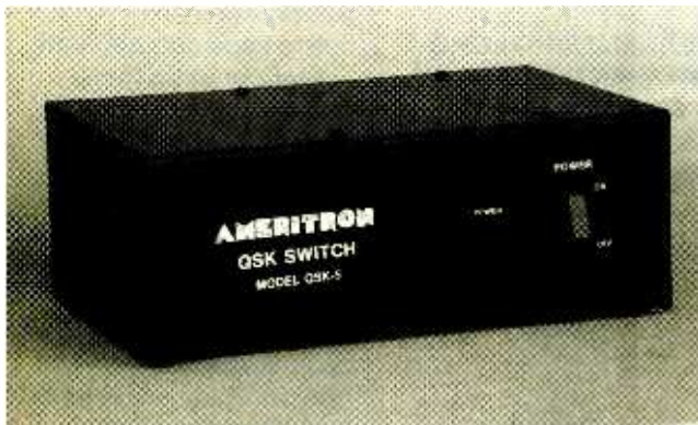
The Ameritron Model QSK-5 external QSK switch (which uses PIN-diode switching) is six times faster than vacuum relays, and preserves linear-amplifier tubes by turning off their plate current between dots, dashes, and digital words.
