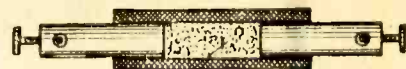
Fig. 1. The Branly coherer consisted of loosely packed coarse metal filings between two metal plugs in a non-conducting tube.
