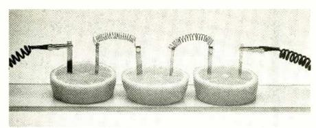
Your organic power cells can be wired together to form multi-cell batteries. Three lemons connected in series should give about 2.8 volts. The negative electrodes on the right side of each lemon slice are zinc; the positive electrodes on the left are copper.
