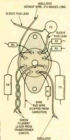
HOOKUP WIRE, 2½ INCHES LONG Fig. 5. Before mounting the tube socket on the board, wire C3, C5, C6, R1–R4, and the three connecting wires to the socket.
