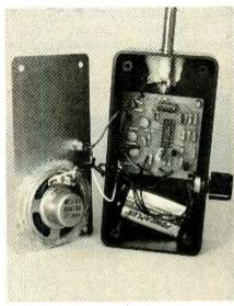
The antenna and speaker for the Countersurveillance Monitor are held in place with silicone cement.
