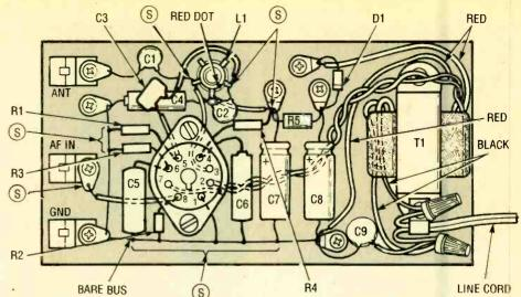
Fig. 6. Mount the tube socket, using two 1½-inch, #6 round-head wood screws. After that, make all of the connections shown here to complete the transmitter.
