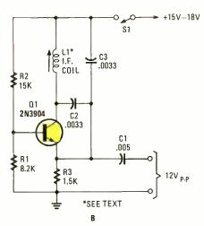
Fig. 6. Here are some simple oscillators. The one shown in A is excellent for testing audio circuits. The one in B would make a good RF receiver tester.
