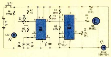
Fig. 4. This more-intelligent transmitter modulates the 40-kHz carrier at a frequency determined by R8.
