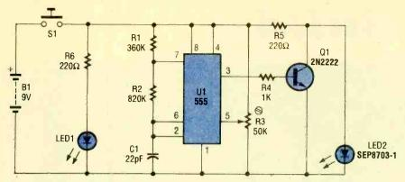
Fig. 1. This simple-looking transmitter makes a 555 timer jump through some amusing hoops: It provides a 50% duty cycle.
