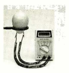
A lemon cell can generate significant voltage if built with the right metal electrodes. Here one is shown connected to a voltmeter.
