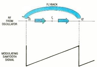
Fig. 1. In a sweep generator, when the modulating sawtooth's signal voltage is zero, the RF oscillator signal is at F1, and its frequency increases as the sawtooth voltage increases until the sawtooth peaks at F2. When the sawtooth drops back to zero the frequency abruptly "flys" back to F1.
