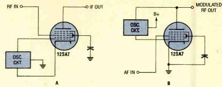
Fig. 1. The 12AS7, typically used in superheterodyne receivers, was configured as a frequency converter as shown in A. When used in a radio transmitter, however, the 12AS7 was configured as shown in B.
