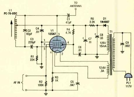
Fig. 2. Here's a complete schematic diagram of the transmitter. In that circuit, an audio signal is applied to grid 3 at pin 8 of VI via the AF IN terminals, and is mixed with the output of a Hartley oscillator.
