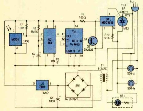
Fig. 2. The basic receiver contains a power supply, an infrared-detector module, a pulse stretcher, a toggling flip-flop, and power-control circuitry.
