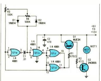
Fig. 2. This circuit uses a method similar to that used in the previous circuit to provide an efficient way of controlling the speed of a DC motor.
