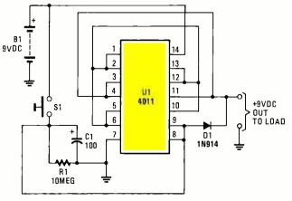
Fig. 5. This battery saver circuit can automatically turn off a small piece of test equipment after a desired period of time, allowing you to leave your shop worry free.
