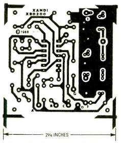
Fig. 2. This full-size template for the Countersurveillance Monitor's printed-circuit artwork is provided for those who wish to etch their own boards. For those not so inclined, a pre-etched and pre-drilled board, as well as the parts that mount on or connect to it, can be purchased from the supplier listed in the Parts List.
