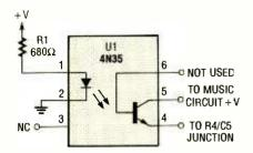
Fig. 5. Optoisolator/couplers, such as the one shown here, can replace SI, thereby allowing the SSMC to be triggered by some other electronic device. Other optoisolator/coupler units, containing various output devices, can also be used in the circuit depending on the intended application of the circuit.
