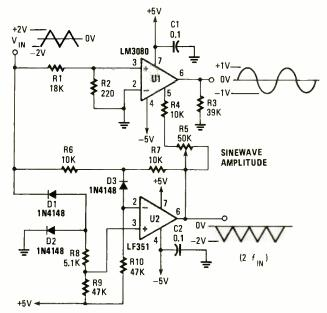
Fig. 7. Unlike most sinewave shapers, this circuit is temperature stable. It varies the gain of a transconductance amplifier to transform an input triangle wave into a good sinewave approximation.
