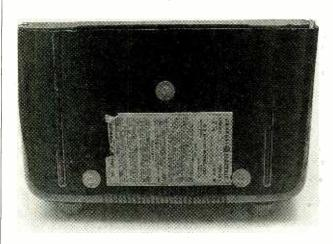
The metal screws holding the chassis to the cabinet are likely to be "hot" when the chassis is. Never touch them with the set plugged in, and never place the radio on a grounded object.
