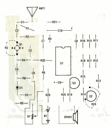
Fig. 3. Assemble the circuit's printed-circuit board using this parts-placement diagram as a guide. Note that transistor Q1, resistors R3 and R24 (all of which are shown as dashed lines) must be installed on the copper side of the board.
