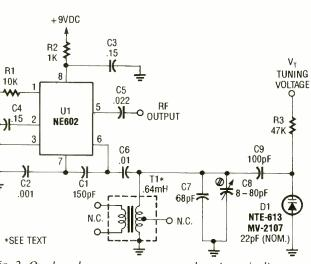
Fig. 2. Our homebrew sweep generator, the schematic diagram for which is shown here, is based on the NE602, an 8-pin DIP integrated circuit that contains a double-balanced modulator and internal oscillator circuit.
