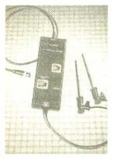
gains, high CMMR, DC to 15-MHz bandwidth, and a constant input impedance of 2 megohms, and 2.5 pF. It is useful with inputs as high as ±700 volts and provides 2% accuracy for outputs as high as ±3.5 volts across loads as low as 1000 ohms. Both inputs are protected against damage to ± 1000 volts. The SI-9000 can be used in monitoring, testing, designing, and troubleshooting applica-
