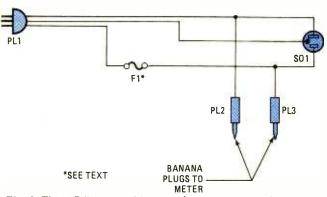
Fig. 1. This AC line-to-multimeter adapter can make checking line voltage safer. You can use it to find taxing loads on your household wiring.
