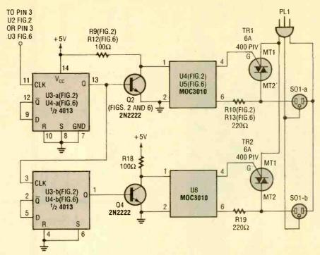
Fig. 8. With a few more components, the receiver can be made to operate two devices or power-control one
