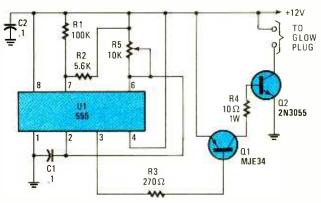
Fig. 1. In this circuit, a 555 oscillator/timer (U1), configured as an astable pulse generator, the output of which is fed to a single-transistor inverter (Q1), which feeds a power transistor (Q2).
