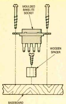
Fig. 4. Once the wiring outlined in Fig. 3 is complete, prepare the baseboard to accept the tube socket. The socket rests atop a ½-inch length of 5/8-inch diameter hardwood dowel.
