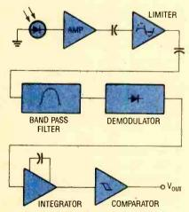
Fig. 3. The infrared detector module performs the task of detecting only the desired infrared signal and converting it into a logic-level signal.
