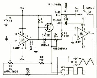
Fig. 8. If you need a source of triangle waves for the circuit of Fig. 7, this circuit will do. It consists of a squarewave generator whose output is filtered to produce triangle waves.
