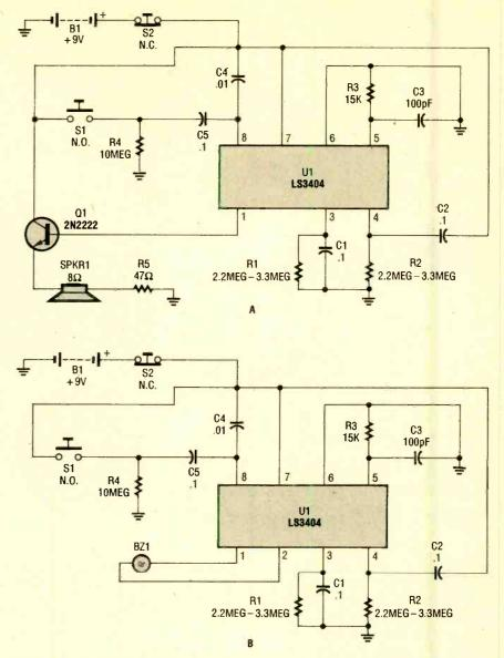
Fig. 1. The circuit in A is designed to drive a conventional 8-ohm speaker, while the one in B is configured to drive a piezo-electric transducer. Other than that, the operation of each circuit is the same.
