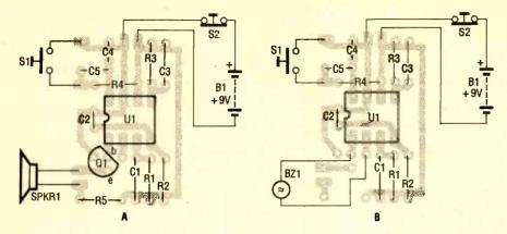
Fig. 3. The parts-placement diagram for the speaker version of the SSMC is shown in A, while B shows the transducer version. Assemble your unit using the appropriate parts-placement guide.
