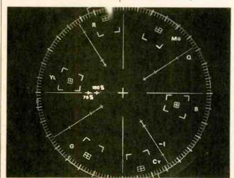
As shown by the location of the white spot in this vectorscope photo, the phase accuracy and color saturation of the Pocket 8 was close to perfect.
