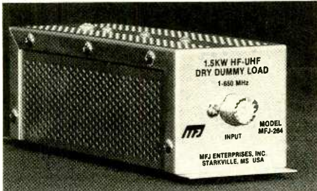
It is improper to tune on the air any more than is absolutely necessary. The proper way to tune up is into a dummy load (artificial antenna), such as this one, and then switch to the real antenna for touch-up and operation.
