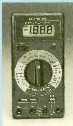
DMM with transistor gain and capacitance measurement features. DIGITS: 3½ DC VOLTAGE RANGE: 1000 volts, 5 ranges AC VOLTAGE RANGE: 750 volts, 5 ranges CURRENT RANGE: 10 amps, 4
