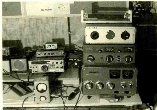
A view of the author's ham-radio station. The dummy load on top of the antenna tuners, although open for modification, is normally shielded. The RF wattmeter in the foreground is usually placed between the rig and the power amplifier. The output of the rig can be switched from the dummy load to the real antenna with a coaxial switch.
