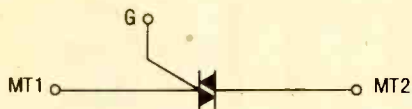
Fig. 1. Triacs are multi-layered three-terminal semiconductor devices. Each terminal has a different function.
