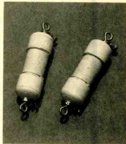
People with space limitations can use shortened dipoles with coils such as these in the two poles.
