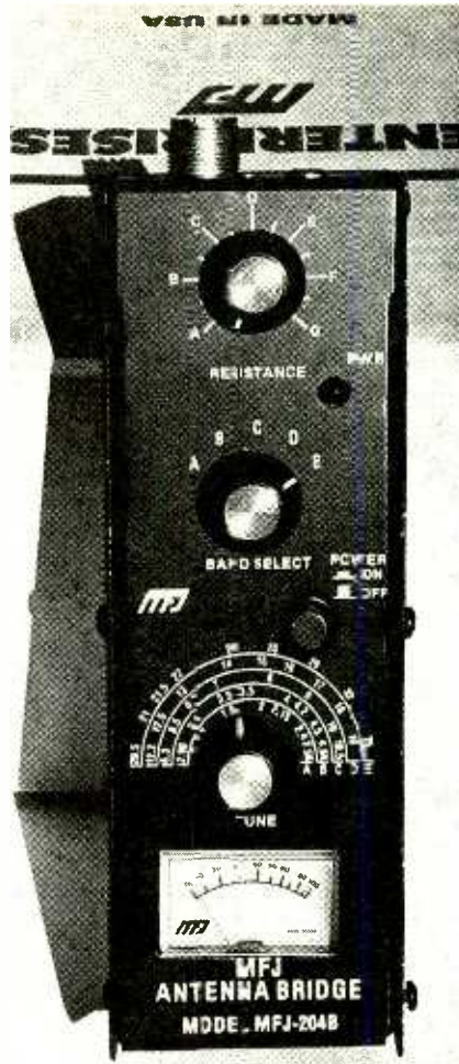
This Z bridge contains a built-in RF generator. That's very helpful to shortwave listeners as they have no broadcast equipment.
