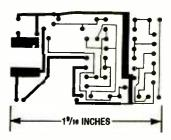
Fig. 2. The Sonic Defender was assembled on a tiny printed-circuit board, the template for which is shown here.
