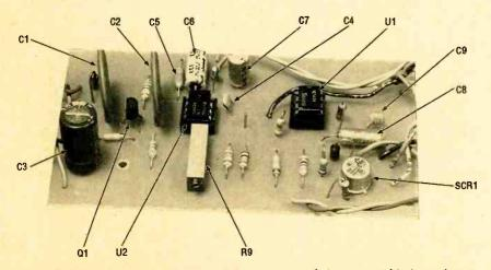
Here is the fully assembled printed-circuit board prior to being mounted in its enclosure. Note that five resistors (R5, R7, R11, R13, and R14) and diode D1 are vertically mounted to the board.
