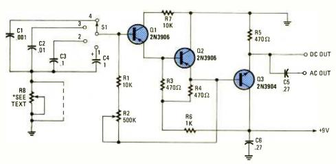
Fig. 1. The variable-frequency pulse generator produces narrow 7-volt positive-going pulses and has a frequency range of 2 Hz to over 50 kHz.
