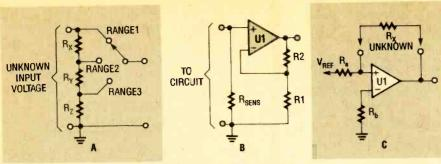
Fig. 7. These various input circuits can allow for a digital-meter circuit to detect voltage (A), current (B), and resistance (C).
