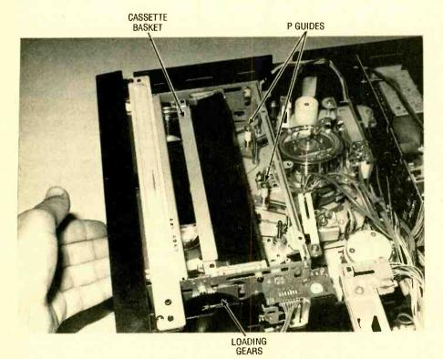
Fig. 2. When you insert a cassette, a switch activates a motor that drives the cassette basket. The basket pulls the cassette in and then lowers it onto the reel table. If the loading gears become out of time (slip a tooth), then the mechanism will jam as it lowers the basket.
