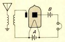
Fig. 4. The audion with external electrostatic control used a plate that was external to the the tube. It was soon followed by a device with an external coil.
