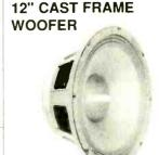
12" woofer made in the USA by Eminence. Paper cone and dust cap with treated cloth surround. 80 oz. magnet. 2-1/2" vented voice coil. 8 ohm. 170W RMS, 235W max. 40-4.5KHz response
