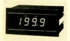
Here's a typical digital panel meter with an LED display. It requires front-end circuitry and switches to be really useful.
