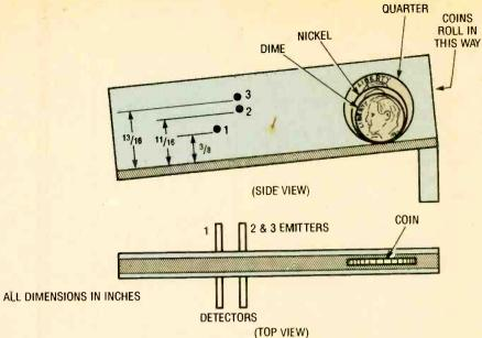
Fig. 2. There are three pairs of IR emitters and detectors: pair I forms a trigger/dime detector, pair 2 is for nickels, and pair 3 is for quarters.
