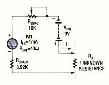
Fig. 4. A meter's internal voltage source is used to drive an ohmmeter circuit.
