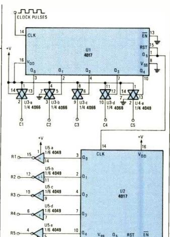
Fig. 5. Two dividing 4017's can be configured to count up to 100. The circuit shown here can count to 25.
