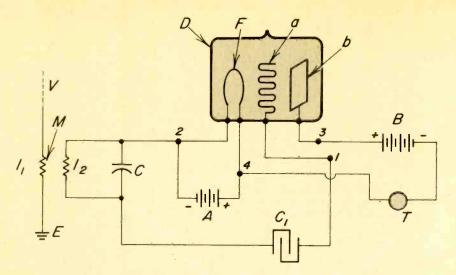
Fig. 5. Lee de Forest's grid audion was the first grid-containing low-vacuum tube. Multiple-electrode tubes were soon to follow.
