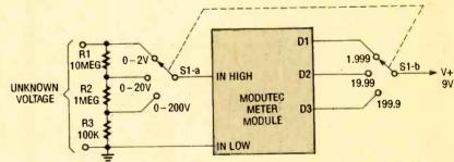
Fig. 9. A simple voltage divider can greatly extend the range of your digital voltmeter. Note the switch selects the proper decimal point for a reading.
