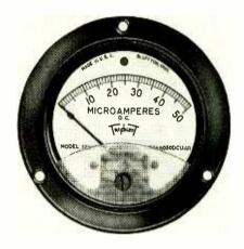
This is the front view of a typical d'Arsonval-type meter movement. Note the zero-adjust screw.
