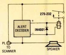
Fig. 4. The buzzer can be replaced by a reed relay provided that your receiver's output jack can drive a speaker directly, thereby allowing you to listen to the warning message.
