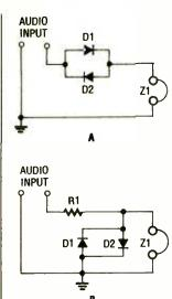
Fig. 2. There are two basic forms of passive noise limiters: the series type (A) and the shunt type (B).
