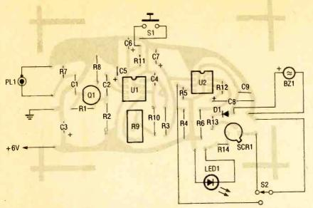
Fig. 3. Use this parts-placement diagram as a guide when assembling the Weather Alert Decoder's printed-circuit board. Note that R5, R7, and R11–R14, as well as D1, are vertically mounted, and that C3, C5, and C6 each have extra mounting holes to allow the use of either axial- or radial-lead capacitors.
