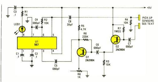
Fig. 2. The proximity detector consists of a 567 tone decoder, a couple of transistors, and a few support components.
