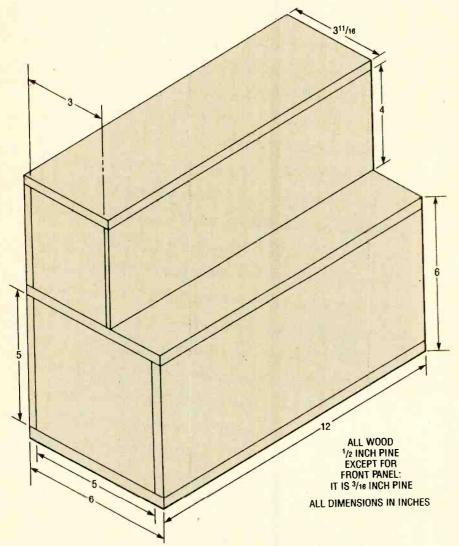
Fig. 9. These are the basic measurements of the cabinet. The top section is hinged to allow access to the bank's coin compartment and the reset button.
