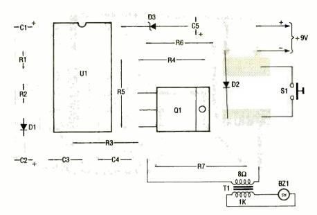
Fig. 3. Assemble the printed-circuit board, using this parts-placement diagram as a guide. Note that because of the small size of the board, it will be necessary to mount several axial-lead components vertically.
