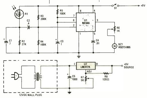
Fig. 7. This simple circuit can turn light into sound. The 555 IC is shown connected as a monostable timer that turns on a buzzer when light strikes R1.
