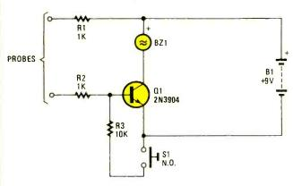
Fig. 3. The moisture detector is nothing more than a transistor (in a common-emitter configuration) that is used as a simple switch.
