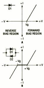
Fig. 1. Shown in A is the current (1) vs voltage (V) curve for a PN diode; B is the curve for a pair of backto-back diodes.
