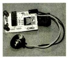
Here is the Sonic Defender's printedcircuit board prior to the mounting of Tl. Once Tl is mounted, the integrated circuit will no longer be visible.
