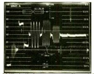
At 2.0 MHz, the video-frequency response was off by some 3.65 dB, which is about average for a basic VHS recorder of this type. At 3.0 MHz, the response had dropped to -17.8 dB. The frequency response of the VCR improved somewhat when the unit was in its edit mode.
