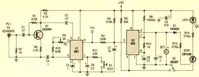
Fig. 1. The Weather Alert Decoder is built around two IC's, a couple of additional semiconductors, and a handful of support components. The heart of the circuit is the Ul (567 tone decoder), which locks onto any signal within its preset capture range.
