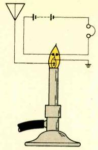
Fig. 2. The second style of flame detector had a local battery circuit which allowed it to operate better.
