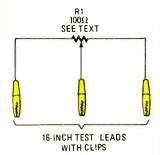
Fig. 4. The variable resistance box can be assembled from junkbox components, and will be of greater service than its simple appearance suggests.
