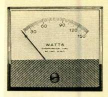
This specialized analog meter is based on a d'Arsonval movement modified to measure watts.
