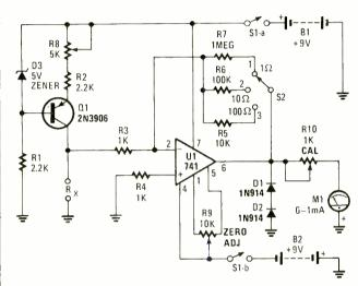
Fig. 4. In this circuit, a general-purpose PNP transistor (Q1) and a 741 op-amp (U1) combine to provide a low-resistance range for your ohmmeter.
