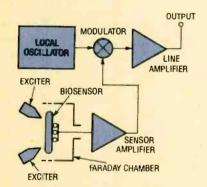
Fig. 2. A cell-type biosensor assembly beats the biological signals with a local carrier oscillator via a modulator.
