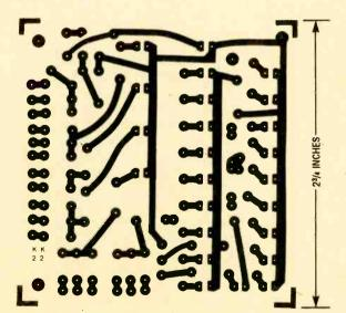
assembly and reduce the possibility of error, printed-circuit construction is recommended. Here's a template for the circuit-board layout used by the author.
