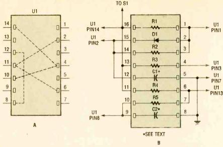
Fig. 3. If you wire the socket for UI as shown in A, and the component socket as shown in B and interconnect them, you'll only have to connect the buzzer, battery, and switch to get your project up and running.
