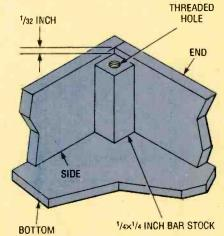
Fig. 4. One way to handle lid mounting is to cut 1/4-inch square bars of acrylic to about 1/s2-inch shorter than the height of the sides. Cement the four pieces into the four corners of the enclosure. Once dry, place the lid on the enclosure and drill screw holes through the lid and into the lid mounts.
