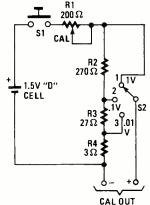
Fig. 3. As with all circuits used to monitor some quantity, the voltmeter circuit of Fig. 2 must be calibrated against a standard. This circuit is ideally suited to that task.
