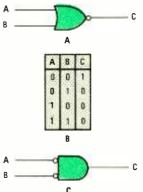
Fig. 1. A NOR gate (A) only goes high when both inputs are low, as shown in B. That is just what a negative-logic AND gate (C) does.
