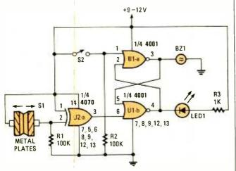
Fig. 9. When this alarm tatches, it activates its own buzzer. Note the use of the NOR-implemented R-S latch.
