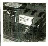
its self-stick backing to attach it to the inside of the computer case, and then plugging the power cable in-line with a disk-drive power cable. Sized to fit inside most desktop and tower computers, the device measures  $3\% \times 2\% \times 2$  inches.
