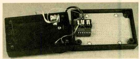
The components are more visible with the two capacitors out of the way. As you can see, using an IC socket keeps the project neat and small.
