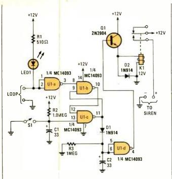
Fig. 8. This alarm-control circuit provides an entry delay, an exit delay, and latching action.
