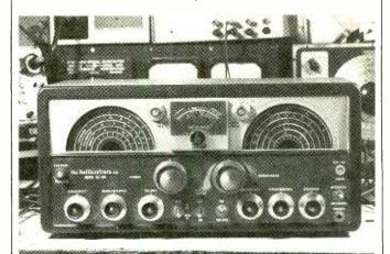
Fig. 4. By the mid to late 1950's, receivers such as this Hallicrafters SX-100 receiver, which used glass-envelope, miniature vacuum tubes, were available.
