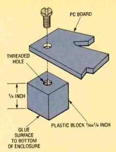
Fig. 3. Printed-circuit mounts can be added to the enclosure by first screwing 1/4 -inch square scraps of acrylic to the board, applying a little acrylic cement to the bottom surfaces of the acrylic squares, and placing the assembly in the desired location within the enclosure.
