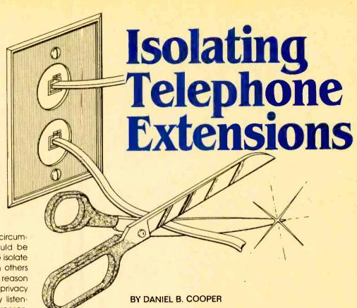
phone jack in the manner we'll describe, it's necessary to understand the fundamentals of home-telephone wiring. All phone circuits require two wires, called (for historical reasons) tip and ring. When the phone is not ringing, the wires carry a direct current with the ring wire at a negative potential with respect to the tip wire.
