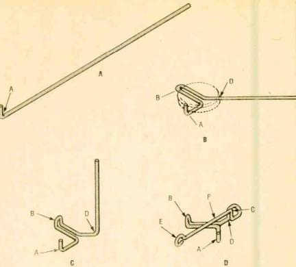
Fig. 3. Follow this clip-bending diagram to form the battery holder for the Electronic Fish Lure. Starting with a straightened large paper clip, make a bend at point A(A), follow by the bend at point B(B), and then the bend at point D(C). Then form a loop at point C and another at point E(D).
