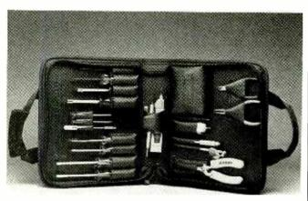
wire crimper/stripper; a four-inch compudriver; an RS-232 insertion extraction tool; a DIP inserter and a DIP extractor; an inspection mirror; and an adjustable 4-inch wrench. The tools are held securely in place in a compact ( $11\frac{1}{2} \times 10 \times 2\frac{1}{2}$ -inch) case that features two roomy outside pockets.
