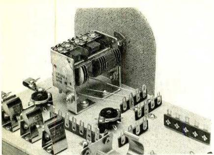
Fig. 5 The lengths of bare bus wire connected to the lugs on the variable capacitor, passed under the body of the unit, and are connected to a terminal strip mounted on the baseboard.
