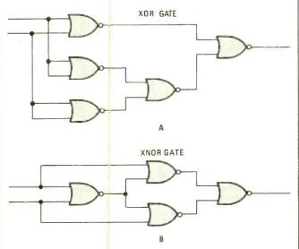
Fig. 4. The logic required to make an XOR is not only a little complex, it requires five gates, as shown in A. The logic required to make an XNOR gate from NOR gates is a little complex, but we show such a circuit in B.
