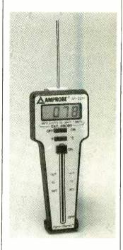
table sensor with a range of  $-50^{\circ}$ F ( $-46^{\circ}$ C) to  $300^{\circ}$ F ( $149^{\circ}$ C). It has both degrees-Fahrenheit and degrees-Centigrade capabilities.
