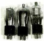
Fig. 6. By the early 1930's, four-, five-, six-, or seven-pin tubes like these (some having grid caps) began to appear.
