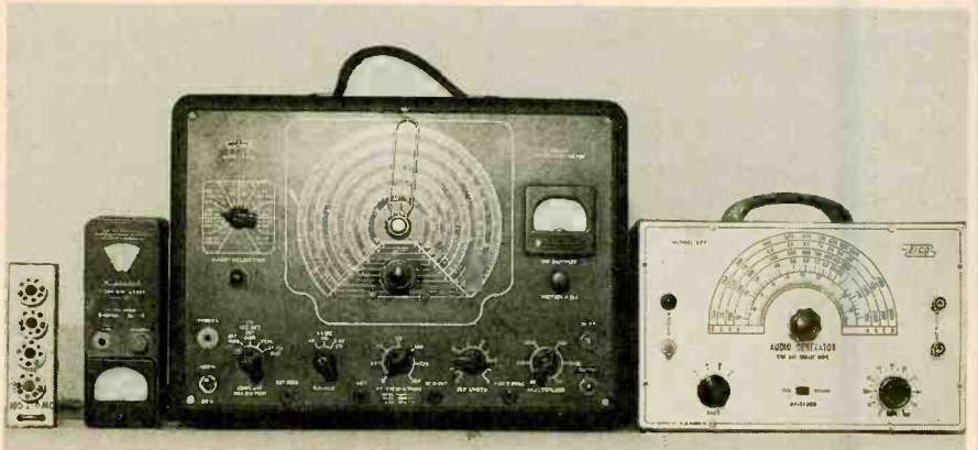
A typical grid-dip oscillator, RF sweep-generator, and audio oscillator. Units like these can be found at most hamfests for around $10.
