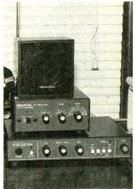
The Heathkit HD-1424-A SWL Active Antenna kit makes an attractive and worthwhile addition to any SW-listening set up. It is shown here with Heathkit's HD-1418 Active Audio Filter.
