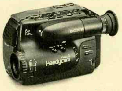
Sony's—and the world's—smallest camcorder, the CCD-TR4, weighs only one pound, nine ounces and measures a mere 4 3/8 x 4 1/8 x 6 5/8 inches. Despite its small size, it has nearly all the features of its larger predecessor.
