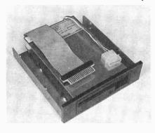
This photo shows a Sony 720K 3- $\frac{1}{2}$ -inch drive. It is setup for mounting in a 5- $\frac{1}{4}$ inch frame with the proper adapter cables to allow this drive to be plugged in as a physical replacement for a 5- $\frac{1}{4}$ -inch drive.
