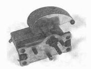
An offset shaft and unusual rotor plates allow this capacitor to track frequency (or wavelength) in LC-tuned resonant circuits.
