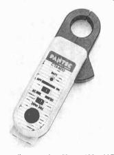
meter readings require either a 100-mV DC voltage range or a 1-volt DC voltage range. The clamp-on adapter requires a 9-volt battery source; an LED low-battery indicator is built-in. The CTA-600 is equipped with standard banana-jack outputs. It has a minimum load impedance of 40 Kohm/V and an operating temperature range from  $0 - 40^{\circ}$ C.
