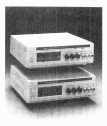
metered displays provide simultaneous viewing of output voltage and current. That feature eliminates the need to measure the output to obtain an accurate output voltage or to limit the output current. In addition, the MPS100 features remote sensing, which regulates the output voltage at the load to compensate for test-lead voltage loss. Both models offer several protection features, including current limiting, reverse-polarity protection, and isolated outputs.
