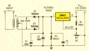
Fig. 7. You could actually construct the variable-output power supply shown here. It can supply your workbench with 1.25 to 12 volts DC.
