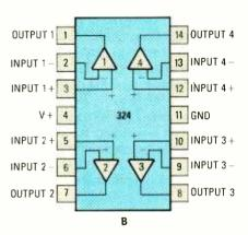
Fig. 6. In this circuit (A), the voltages that  $ar\epsilon$  to be compared are derived from typical voltage-divider networks: R1 and R3 for the inverting inputs; and the R2/R4 and R6/R5 combinations, for the non-inverting inputs. Shown in B is the pinout diagram for the 324 quad op-amp.
