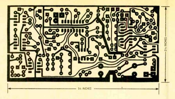
Fig. 2. This printed-circuit template was used by the author to produce his prototype unit. This pattern can be copied to a printed-circuit slug (unetched PC board material) to produce your own board.
