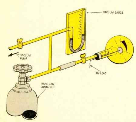
Fig. 6. Small amounts of rare gases were introduced into the plasma globe using this set up. A high voltage was then applied to study the effects of the gas.
