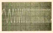
An expanded view of the frequency-sweep signal output by the Audio Sweep/Burst Generator. The signal starts (left) at a relatively low frequency (left), and increases at a rate determined by the operator, as the generator's output is swept through the audio spectrum.
