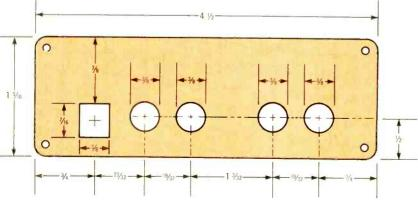
Fig. 4. Here are the front- and rear-panel layouts for the enclosure used by the author to house his prototype unit: A shows the template for front-panel layout and B is the rear-panel layout.
