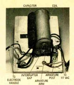
Here's a restored generator circuit. Use as much fresh hardware as possible. The screws going into the compartment lid should be fairly short; long ones will go straight through and damage the outer surface.
