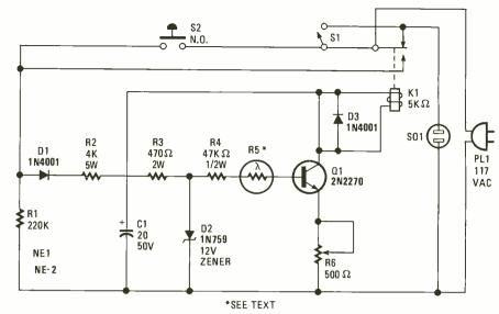
Fig. 9. This circuit is little more than a light-dependent switch circuit that's used to trigger a relay, which in turn feeds AC power to the device connected to the socket (SOI).
