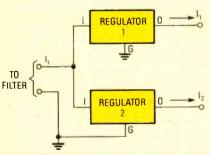
Fig. 6. To get multiple voltage outputs from a power supply you simply have to piggy-back the regulators provided the other components can handle the additional current requirements.
