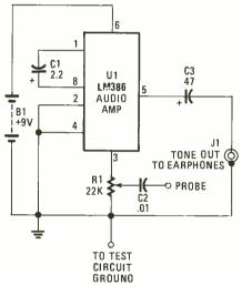
Fig. 8. The Signal Tracer circuit presented here is essentially a variable-gain amplifier.
