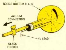
Fig. 5. A high voltage was applied to the electrode while air was evacuated using a simple one-stage vacuum pump.
