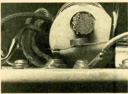
Contact surfaces should be parallel. You can bend the armature arm with your fingers so be careful. Note how all the wires have been bent clear of the interrupter gap assembly.
