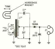
Fig. 6. In this unusual tunable crystal radio, the hard-to-locate broadcast-band tuning capacitor is replaced by a fixed capacitor and a horseshoe magnet.
