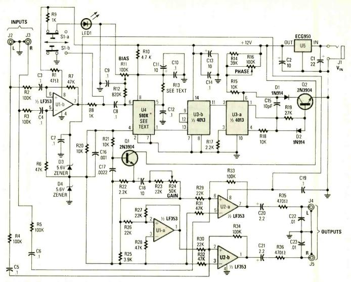
Fig. 1. At the heart of the Sonic Emulator is a bucket-brigade device (U4, one of a series of 510X devices), which is used to place delay in the audio signal, thereby expanding stereo imaging to produce concert-hall-like effects.
