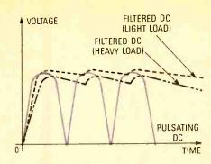
Fig. 3. As you can see, when pulsating DC is filtered insufficiently the troughs between peaks deepen. Using the right capacitor for the right job is a good motto to learn from this.
