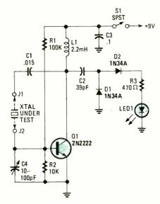
Fig. 4. In the Crystal Tester circuit, transistor QI is connected in a Pierce oscillator configuration with the crystal under test supplying the feedback from QI's collector to its base to produce and sustain oscillation. If the circuit oscillates, the crystal under test is good.
