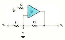
Fig. 4. Single-ended comparators with hysteresis are also possible.
