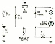
Fig. 5. The Instrument Alarm is nothing more than a simple tilt switch, whose operation is wholly dependent upon SI (a mercury switch).
