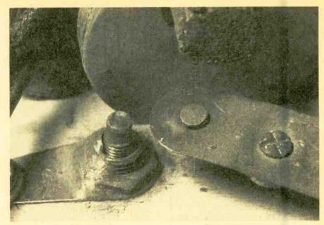
The output of the Violet Ray Generator can be improved by carefully cleaning the contact points. Both the armature arm and the adjusting screw can be removed to make the job easier.
