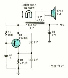
Fig. 5. This tunable tone generator uses a horseshoe magnet to vary the inductance of LI, thereby altering the output frequency of the circuit.
