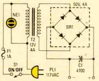
Fig. 2. This simple circuit allows the power supply to be operated from 117-volts
