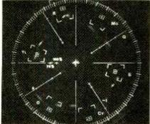
This vectorscope measurement of NTSC record/play tapes shows that color phase (accuracy) and intensity was near perfect.
