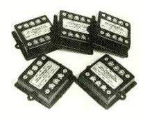
Custom units for up to 1024 lines are also available, and multiple banks can be added in parallel for larger systems. The 2-, 6-, and 8-line units are configured in individual modules using screw terminal connectors. Larger systems use plug-in circuit cards of 16 lines each that plug into a custom integrated rack-mount system. Each cabinet features an interconnecting backplane, power supplies, and a distribution network.
