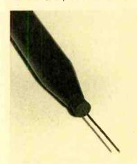
Push the loop into the barrel, fit the stopper down over the wire, and your probe is done.
