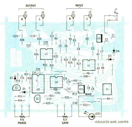
Fig. 3. Using this parts-placement diagram as a guide, begin assembly by installing IC sockets at all positions where IC's are indicated, except U3. Install the jumper connection that runs beneath U3 first, and then install the socket for that IC. After all IC sockets and jumper connections are in position, install the rest of the components—resistors, capacitors, transistors. IC's, etc.
