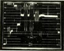
A low-frequency video-burst signal was used to evaluate playback video-response. The test results in the PAL mode at SP speed are shown here.
