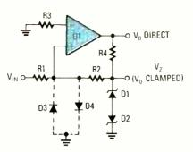
Fig. 5. Adding a Zener-diode clamping network in the positive feedback loop is one solution to the varying thresholdvoltage problem.
