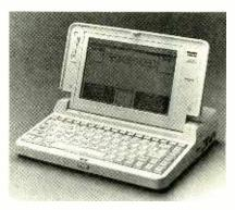
has a parallel printer port, a serial communications port, and one dedicated internal modem slot.
