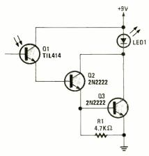
Fig. 7. The IR Remote Checker consist of little more than an infrared-sensitive phototransistor, and a pair of generalpurpose transistors connected in a Darlington configuration, to provide sufficient drive to light LEDI (a visible light unit).
