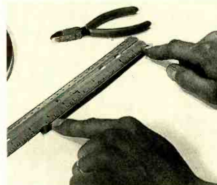
Replace the rubber drive belt with one that's a 1/4-inch smaller than the old belt. Fold it or combine the pieces along side the roller for correct size.
