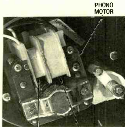
This portable turntable motor has a separate winding to power the audio amplifier. The motor acts as a transformer and the AC voltage is full-wave rectified.
