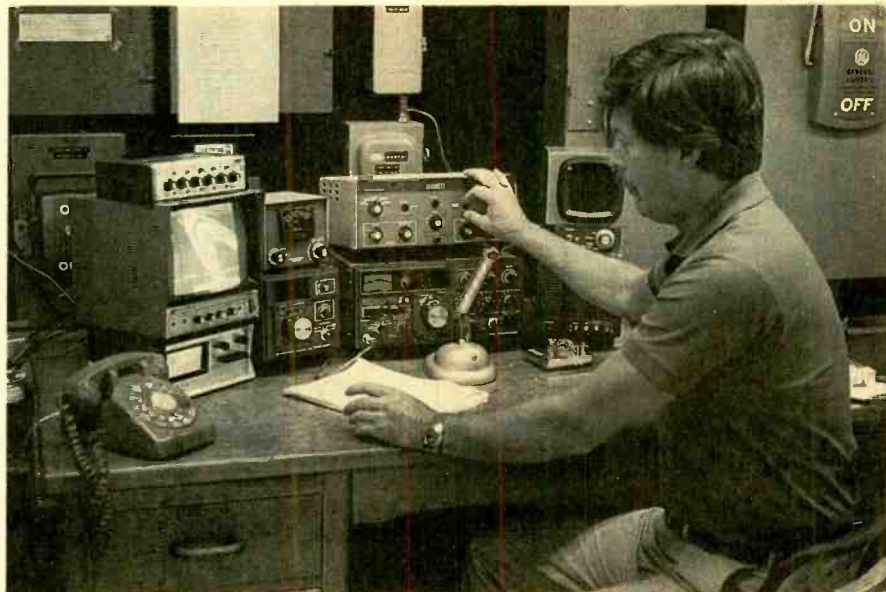
Here's a fellow ham using slow-scan television to view Voyager 2 pictures of Saturn. The images are retransmitted to ham radio operators worldwide by members of an amateur radio club at The Jet Propulsion Laboratory in Pasadena, California moments after scientists there received the images from space. (Photo courtesy of American Radio Relay League.)
