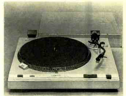
Notice if the arm keeper is locked over the pickup arm when it will not play or reject. Also check for a broken lever.
