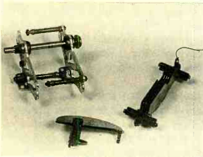
Here's how the capacitor looked after being dismantled for rebuilding. Frame is at upper left; stator at right; rotor (with most of its plates missing) is in foreground.
