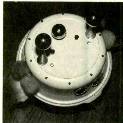
Antennas are mounted to the outside of the bottom half of the bowl. Two giant LED's are mounted near the center of the bowl between the antennas, and jumbo LED's are ringed around the bowl's perimeter.
