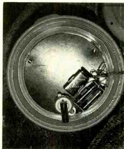
Mounted to the lid of the bowl that houses Shaky's circuit board are the motor (MOT1) with off-balanced weight and the batteries that provide power for the circuit.
