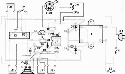
Fig. 3. After preparing your printed-circuit board, consult this parts-placement diagram for the location and orientation of Auto-Scan's board-mounted components. The components not shown on the board are mounted on the front and rear panels of the enclosure.
