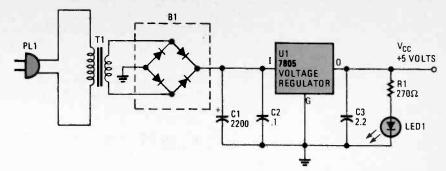
Fig. 1. The power supply shown here was developed in the previous article. The LED and series resistor (LED1 and R1) are additions to the power-supply circuit that was assembled in the previous exercise.
