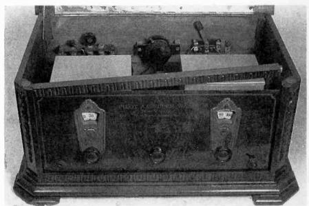
Here's the A.C. Super-Wasp just prior to disassembly for inspection. Locking rail at top of panel is partly removed (see text).
