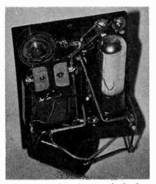
Although large by today's standards, the Cummings Solodyne was very compact for 1928. All components are mounted to the front panel by either the pin jacks or the screws holding the variable capacitor,
