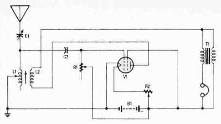
Fig. 1. The basic solodyne circuit used a single battery to power a two-grid tube. The same thing can be accomplished with a triode as well.
