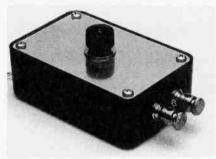
Under the knob on top of the unit is an old plastic single-pole, single-throw rotary switch. A small SPST toggle switch will work just as well.
