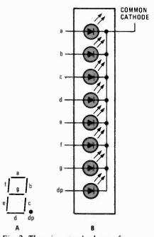
Fig. 2. There is a standard way of labeling the segments of a seven-segment display (A). Electrically speaking, a 7-segment display is nothing more than a group of light-emitting diodes (assembled) in a single package with one side of each connected together as shown in B.
