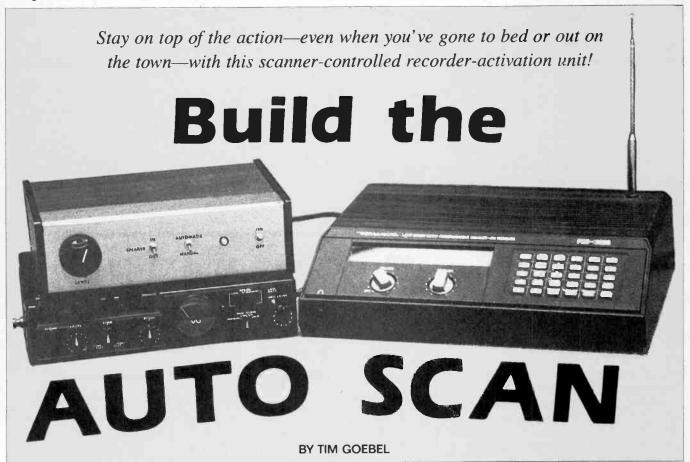
Some of the hottest action to come over the airwaves for months, and you missed it...that is, until *Auto Scan*. With Auto-Scan connected between your scanner and a tape recorder (via the recorder's microphone or auxiliary input and its remote start jack), you'll never have to worry about missing any of the action.
