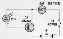
Fig. 1. When the solar cell is illuminated, a positive bias is placed on the base of Q1, causing the transistor to conduct, thereby applying power to the motor.
