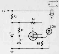
Fig. 12. Solid-state switching devices usually incorporate more circuitry than the examples we've used thus far. This circuit should give you a better feel for the internals of such a device.
