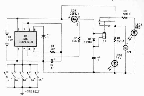
Fig. 1. This burglar alarm circuit is built around a 555 oscillator/timer (UI), configured for monostable operation.
