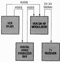
Fig. 2. Should your receiver not have video and audio input jacks, two VCR's are required to process the signal.
