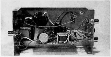
An interior view of the Sferic Level Monitor just prior to the sealing of its aluminum enclosure. The perfboard assembly, which contains the circuit's major components, is mounted to the enclosure wall with "L" brackets.
