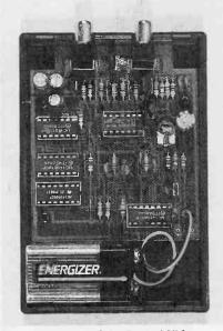
This inside view of the Digital Video Stabilizer RXII reveals an uncrowded circuit board with five IC's and a handful of other parts. A 9-volt transistor-radio battery powers the project for more than a year, so no on/off switch is required.
