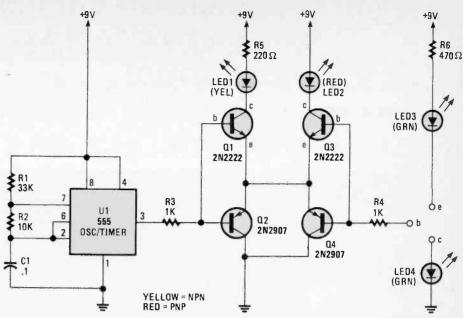
Fig. 5. The transistor tester, aside from giving a visual indication as to the fitness of the unit under test, can also help identify whether a transistor is a PNP or NPN type.
