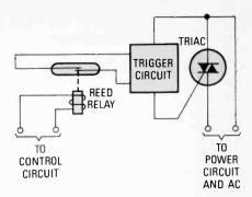
Fig. 7. The small size of reed relays makes them good isolation devices for solid-state relays.
