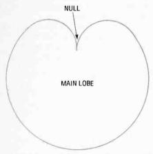
Fig. 3. The cardioid pattern of a proper RDF antenna is a lot less ambiguous than the bidirectional antenna.
