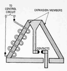
Fig. 10. By using two expansion members to hold the moving contact, the effect of ambient temperature is canceled out.
