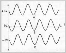
Fig. 2. This is the affect of applying DC offset to a sine wave. Shown are offsets of +3 VDC (A), 0 VDC (B), and -3 VDC (C) all affecting the same wave.
