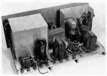
Rear view of Wasp's chassis. Shield can for screen-grid RF stage has been partially dismantled to gain access to wiring.
