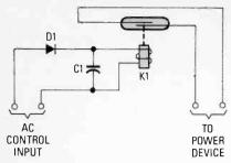
Fig. 9. By rectifying and filtering an AC control signal, it can be used to actuate a DC reed relay provided C1 can charge sufficiently on any given halfcycle.
