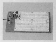
Connecting the jumpers as shown before the rest of the circuit will be very helpful to you because they set up supply and ground lines for the experiment.
