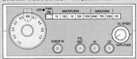
Fig. 1. This is the front panel of a generic low-cost function generator. A standard audio generator differs from the function generator in that it has a precise output control, and may generate only sine waves.
