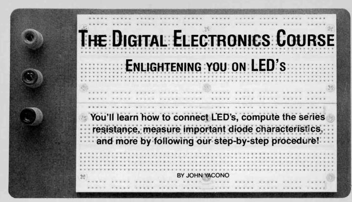
ight-emitting diodes (or LED's) are small diodes that give off light. All diodes are composed of two different substrates sandwiched together. A terminal is connected to each substrate; one is called the anode and the other the cathade. When the anode is slightly more negative than the cathode, current will not flow through the diode. That is called reverse biasing the diode would be forward biased and it will allow current to flow.
