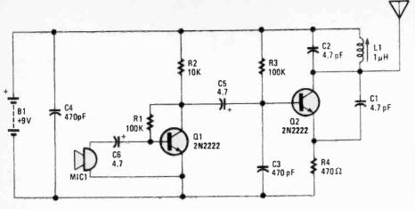
Fig. 7. The wireless mike is really an electret-microphone element feeding its output signal to a miniature transmitter, operating somewhere in the range of 88 to 95 MHz.
