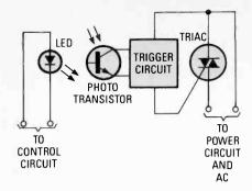
Fig. 4. The greatest isolation between power and control circuits is displayed by optical-coupling devices. They are also among the fastest-acting devices.
