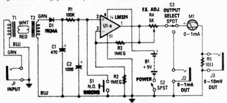
Fig. 4. Here is the schematic diagram for the Sferic-Level Monitor.
