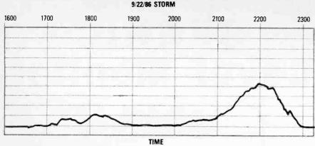
Fig. 1. Here is a chart recording showing sferic level vs. time, which was collected during the approach and passage of a storm.
