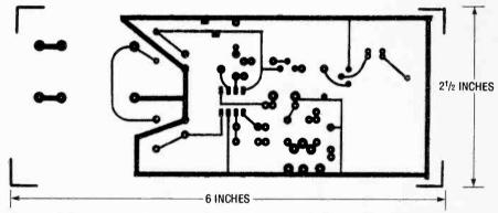
Fig. 2. While there is nothing critical about the layout of the circuit-board components to prevent you from devising your own design, using the printed-circuit foil pattern shown here will certainly make things go a bit easier.
