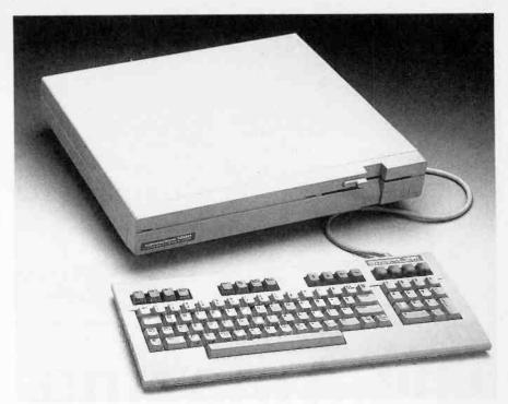
First it was the venerable Commodore 64, then the 128, shown here, that were popularly dubbed the "flagship" of Commodore's fleet; now the Amiga carries the flag. The C-128 is an 8-bit C-64 upgrade that is 100% compatible with C-64 programs and also offers an 80-column screen and CP/M operation. (Photo courtesy CBI, Inc.)
