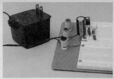
Your completed power supply should look similar to this. Note how the leads are carefully routed around components.
