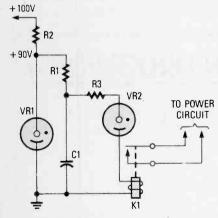
Fig. 11. Charge-operated vacuum-tube devices can be used to sense voltages above a certain level to provide switching control for a relay.
