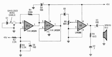
Fig. 1. Our drum simulator uses a capacitor to detect the tapping of the stick. The detected signal is then amplified, conditioned, and used to drive a 4-ohm speaker.
