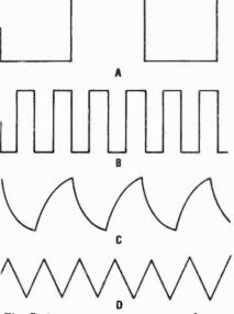
Fig. 7. As you pass square waves of various frequencies (shown here are 100 Hz (A), 1000 Hz (B), 5000 Hz (C), and 50 kHz (D)) through a 5-Hz low-pass filter it dampens some of the wave's harmonics, transforming the wave into a new shape (triangle).
