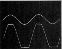
Fig. 4. When an input sine wave (top) is clipped by an amplifier, it develops plateaus, as the lower trace shows.
