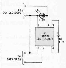
Fig. 6. The capacitor tester/analyzer is built around an LM3909 oscillator/flasher (UI), in fact, you might say that the LM3909 is the whole thing.
