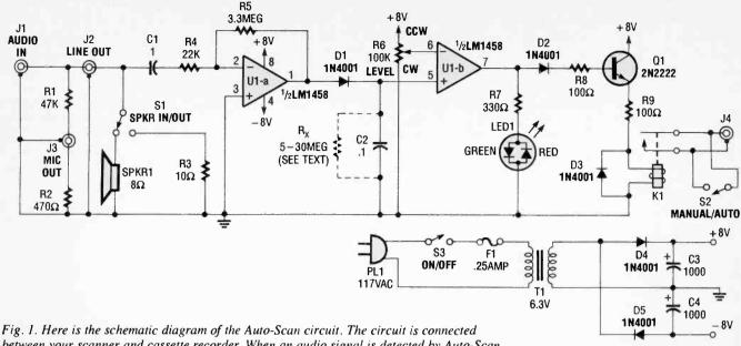
between your scanner and cassette recorder. When an audio signal is detected by Auto-Scan, it activates the recorder, keeping you in touch with all the action.
