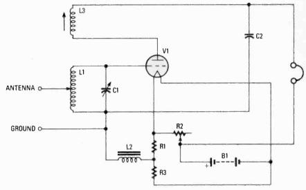
Fig. 2. The Cummings Solodyne was unusual in the fact that it only uses one battery instead of the usual three batteries as did most of the receivers of the era.
