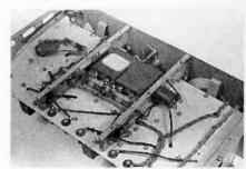
View of the set's underside. Cathode bias resistors for two of the stages, along with their associated bypass capacitors, are located in the center section.
