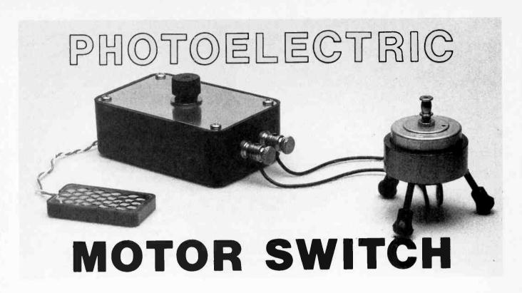
This simple photovoltaic switch project helps you to understand how photo cells can be used to your advantage.
