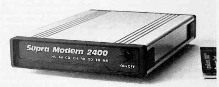
The SupraModem 2400 is an inexpensive 2400-baud modem that supports most computers w an RS-232C interface, including all Amiga models. (Photo courtesy Supra Corporation.)
