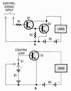
Fig. 6. Buffering the control signal from the power-switching component, as in A, provides some degree of isolation. Of course, some applications require little isolation, so the simple transistor switch in B will do for DC control signals.
