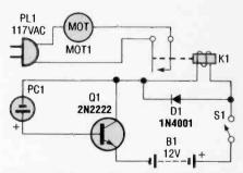
Fig. 2. With a simple modification to the basic photo switch of Fig. 1, the circuit can be used to activate of line-operated devices such as motors, lamps, etc.
