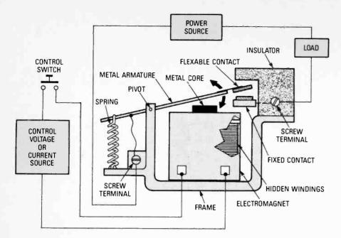
Fig. 1. The ever-enduring armature-type relay is an elegantly simple device. The electromagnet attracts the armature and pulls it down so the contacts touch.
