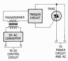
Fig. 5. The DC-AC converter in the circuit is not necessary for an AC control signal. However the transformer would still be useful as an isolating device.
