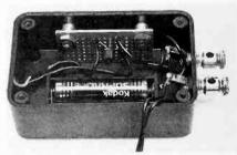
A small project box provides just enough room for a 3-volt "AAA" battery pack and a piece of perfboard for the transistor.
