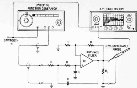
Fig. 5. This is the set-up you would use for testing a low-pass filter or other frequency-selective amplifier using a sweep frequency generator.
