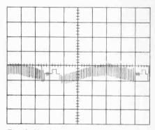
Fig. 3. Here's what your video signal would look like if the video signal is sinewave encoded. The coded sync pulse is below the level of the video signal and can be hidden from your TV set, causing it to run wild.
