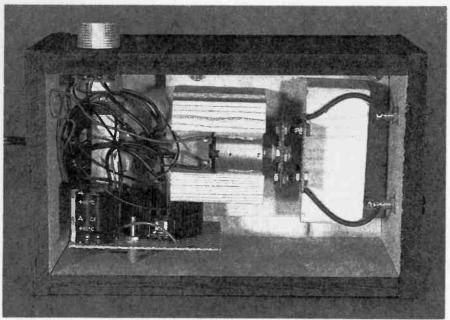
Here's an inside view of the rotary spark gap; note the tight spacing between the perfboard rotor and the stationary post. The wires coming from the stationary post are connected to J4 and J5, through which the rotary spark gap is connected to the Tesla Coil circuit.
