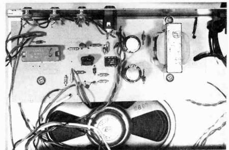
Here is an overhead view of Auto-Scan's printed-circuit board mounted into its enclosure. Note that the speaker is mounted on the bottom of the enclosure with the board hovering above it on stand-offs.
