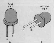
Fig. 3. New or unused LED's can be inspected and the cathode determined without making any tests. The shorter lead (denoted K)—which is also nearest to the flat portion of the LED's lower rim—is the cathode.
