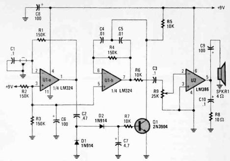
Fig. 2. This circuit is similar to the circuit in Fig. 1, except that the signal detected by the capacitor sensor is used to trigger the circuit.
