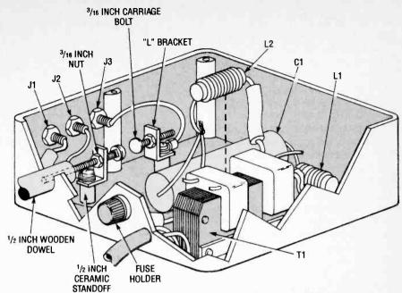
Fig. 3. The stationary spark gap is made from two 3/16-inch carriage bolts supported by "L" brackets mounted to spacers so that they face each other. One bolt is made stationary, while the other is made adjustable so as to vary the spark gap.
