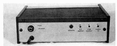
This is a view of Auto Scan's rear panel. The fuse, as well as the remote-input, mic-output, line-output, and audio-input jacks are located on the rear panel of the enclosure. All connections to and from the Auto-Scan unit are through those jacks.
