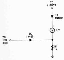
Fig. 2. This lights-on reminder is probably the simplest one yet, consisting of only four extremely non-critical, commonly available components!
