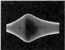
Fig. 9. The output waveform from testing an LC tank circuit without rectification looks like this. Rectifying the output would give you an accurate frequency-response curve of the tank circuit under operation.
