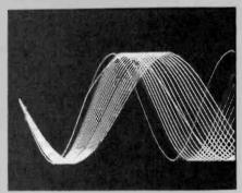
Fig. 3. A frequency-swept sine wave will draw many traces on an oscilloscope. Notice how they all start at the same point due to the oscilloscope's triggering mode, but they diverge because of their different frequencies.
