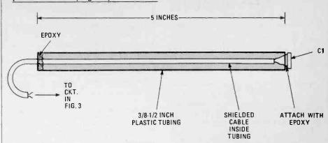
Fig. 4. Shown here are construction details for the probe unit used with the knock-detector circuit.
