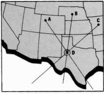
Fig. 1. Illustrated here is the method used in triangulation. Bearings on the hidden transmitter are taken from three or more directions, and plotted on a map. The point where the lines intersect is the location of the the hidden transmitter.
