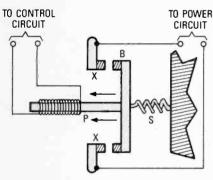
Fig. 2. The plunger relay is excellent for switching high voltages because of the large distance between the contacts.
