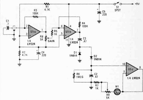
Fig. 3. Here is a circuit that should be of interest to car buffs and others involved with tracking down the source of strange knocking noises in electro-mechanical devices.
