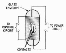
Fig. 3. The reed switch is an interesting electromagnetic relay in that the contacts are made to attract one another and close.
