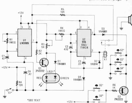
Fig. 4. This auto-alarm circuit has a variable exit delay, an LED indicator, and an auto-reset function—some of the same features touted for commercially available units.
