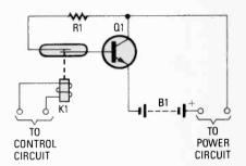
Fig. 8. For DC-power control, a reed-relay/transistor combination makes an effective switching device.
