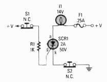
Fig. 2. This circuit uses an SCR, two pushbutton switches, and an incandescent lamp to indicate whether your vehicle has been tampered with.
