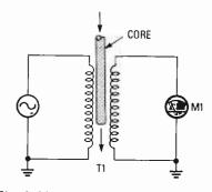
Fig. 6. Movement of the core results in changing the coupling between the transformer windings, and thus the reading on AC meter M1.
