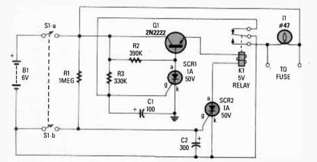
Fig. 1. The rocket launcher is a rather simple circuit, whose operation is almost solely dependent on two SCRs and a relay.
