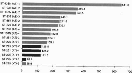
Fig. 1. Shown here is a performance comparison of several popular drives. What's being measured is the raw-data transfer rate—the fastest rate at which a particular combination of drive, controller, and system bus can operate.
