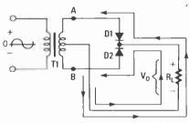
Fig. 4. The arrows on both sides of the supply line going to load resistor,  $R_L$ , indicate the current flow during the two half cyles of the waveform.
