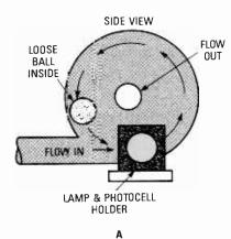
Fig. 9. As you can see in the side view (A) the loose ball is allowed to rush past the lamp/photo cell assembly (B) and the frequency of the pulses produced by the photo cell will be proportional to the rate of flow of the fluid propelling the ball.
