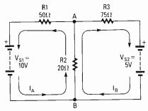
Fig. 3. Two loops for this circuit have been arbitrarily selected to assist us in writing the voltage equations.
