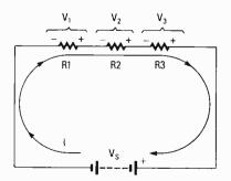
Fig. 1. This series circuit should make Kirchhoff's voltage law obvious. The sum of the voltage drops around the loop must equal the source voltage.
