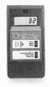
level. The unit can be interfaced to a computer for recording monitored levels, or to an external warning device. The Geigertube radiation detector is sensitive enough to measure radiation from uranium-oxide pottery glazes, old radium-dial clocks and watches, gas camping-lantem mantles, and rock collections. The Radalert is powered by a 9-volt battery; a jack is provided for an optional AC adapter.
