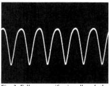
Fig. 3. Full-wave rectification allows both halves of the AC waveform to be used by effectively flipping over the negative excursion through diode switching.
