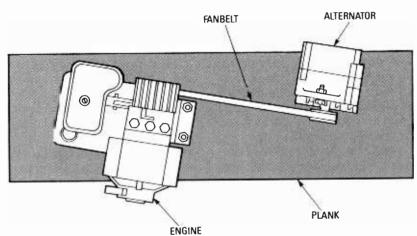
Fig. 2. As shown by this overhead view, the engine and alternator are mounted somewhat off-center, with their drive shafts opposing each other.
