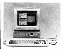
floppy-disk drive occupy two of the three half-height drive slots; one slot is left for additional mass storage, or for other disk formats. The floppy-disk controller (on the system board) supports 5<sup>1</sup>/4-inch drives in 360K and 1.2-meg configurations, and 3<sup>1</sup>/2inch drives in 720K and 1.44-meg formats. A software-setup utility guides the user in setting up system parameters for any combination of drives and formats.
