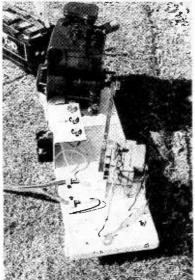
Note the slight angling of the alternator and engine. If the alternator and engine were not mounted in that manner, a wider wooden plank would be needed to accommodate the assembly.
