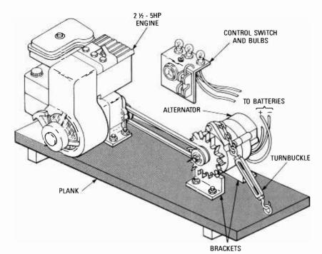
Fig. 1. Here is a general layout of the Homemade DC Generator.
