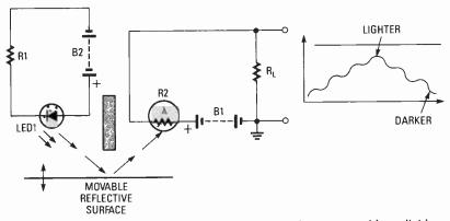
Fig. 11. By placing an LED and LDR close to each other, but separated by a divider, they can be used to indicate the relative proximity of a reflective surface.
