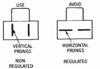
Fig. 3. This illustration shows the two types of sockets likely to be found on the alternator. The one on the left (with its vertical prongs) is suitable for this project, while the one on the right (having horizontal prongs) should be avoided.
