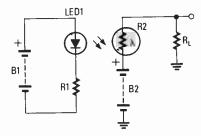
Fig. 10. Interrupted light applications include things such as smoke detectors.
