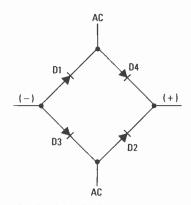
Fig. 5. The diode bridge full-wave rectifies AC without the aid of a center-tapped transformer.
