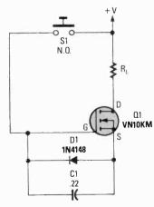
Fig. 3. In this circuit, an FET along with a capacitor is used as an automatic cutoff, electronic switch.
