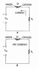
Fig. 2. When the diode is forward biased (A) it allows the AC voltage to be presented to the load. When reverse biased, the diode shuts off and acts like an open circuit (B).
