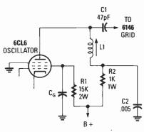
Fig. 1. Here's a partial schematic diagram of the crystal oscillator in the DX-60B. After many years in storage, the slug in LI-the tuned coil-had changed somewhat and the coil was no longer resonant.
