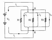
Fig. 2. The current entering a circuit (or any one node) must be equal to the current leaving it, as this circuit makes apparent. Nodes don't have leaks.
