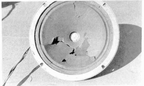
Speaker cones in this sad state can be made to work again if one is desperate or determined enough. In this case, a replacement loudspeaker would be the best alternative.
