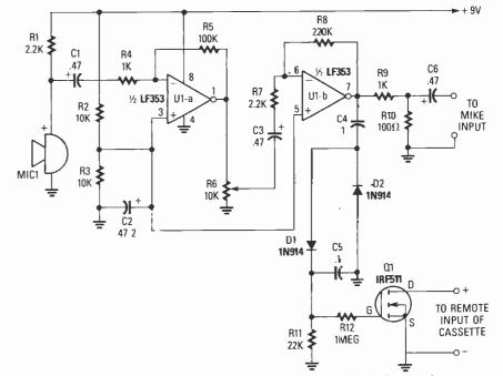
Fig. 7. The electret microphone MICI picks up the sound and feeds the signal to a two-stage amplifier circuit, consisting of UI-a and UI-b, the output of which is fed to a voltagedoubler circuit (made up of D1, D2, C4, and C5).
