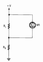
Fig. 1. Variations in the sensing resistors resistance,  $R_s$ , will show up as voltage changes across the load resistance,  $R_1$ , for display on M1.
