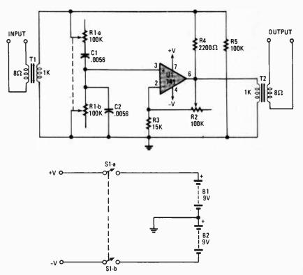
Fig. 1. The Audio Q-Multiplier combines two old-time circuits, the Q-multiplier and the Wein-bridge oscillator, to make an audio filter that's simple, but very effective. Potentiometer R1 sets the frequency while R2 controls the selectivity from wide-open to razor sharp. The filter will boost the performance of almost any receiver.
