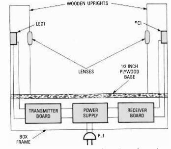
Fig. 2. In the author's prototype, the wires between the receiver and transmitter boards. and the electromagnet (L1), the solar cell (PC1), and the IR diode (LED1) were run through ducts drilled into the wood uprights, and cross brace.
