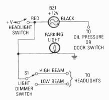
Fig. 6. By properly installing a buzzer in your auto, you'll be alerted whenever you inadvertantly leave on the lights.
