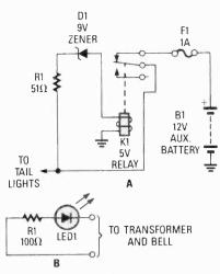
Fig. 5. The circuit in A allows you to charge the main battery in your camper from an auxillery battery while the vehicle is in motion. The circuit in B can be used to replace a burnt out lamp in your doorbell system.
