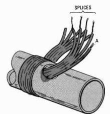
Fig. 2. Use these connections if your preference is broadcast-band DX listen ing. They put all 5 conductors in series for the maximum physical length.
