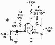
Fig. 1. In this circuit the IRF511 is configured as a class A amplifier. Ideally, for class A operation, the voltage across Q1 and the load resistor should be equal. By Charles D. Rakes
