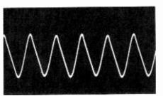
Fig. 10. A close up of the ripple on top of an already filtered pulsating DC looks pretty bad. However, it can be eliminated through the use of a regulator.
