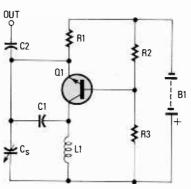
Fig. 4. Changes in the output frequency of this circuit indicate changes in its sensing capacitance,  $C_s$ .
