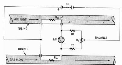
Fig. 3. The flow rate and quality of air can be measured with this device. The circuit is normally balanced 'till some condition in one of the tubes changes.
