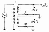
Fig. 5. Even small changes in the sensing capacitance will strongly vary the voltage sent to the VTVM.
