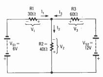
Fig. 6. This is a revised version of Fig. 5 with the branch currents and voltages with polarities in place.
