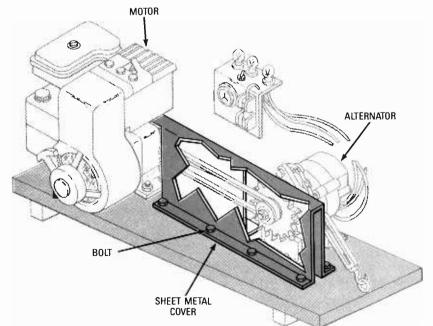
Fig. 6. As a safety measure, it is recommended that a cover for the fanbelt/pulley assembly be fabricated from a piece of sheet metal. Be sure to make the cover large enough to allow free movement of the fanbelt/pulley assembly, without obstructing the free movement of the rest of the project.
