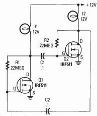
Fig. 4. In this circuit, two hexFETs are configured as a simple astable multivibrator to alternately switch the two lamps, 11 and 12, on and off.
