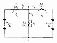
Fig. 4. The three individual branch currents help us determine the polarity of the voltage drops in the circuit as well as the currentnode equation.
