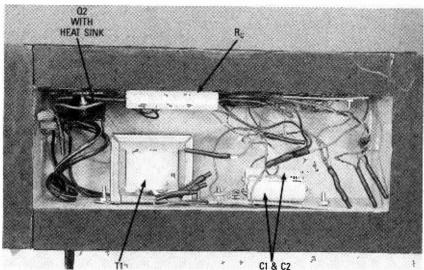
Here's an inside view of the sectionalized circuit mounted in the base of the Anti-Gravity Generator. The large high-wattage resistor  $(R_c)$  is connected in series with the electromagnet (L1) to bring L1's impedance up to at least 30 ohms.
