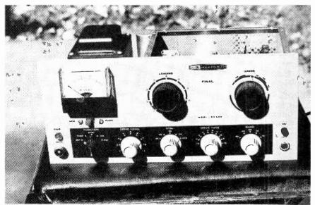
Before purchasing old equipment of any type, it's best to check out its innards. Pay particular attention to the electrolytic capacitors and the power transformer.
