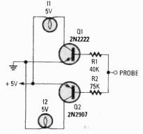
Fig. 7. By connecting this circuit to a logic device that's under power, you can get an indication as to its status.
