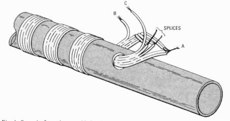
Fig. 1. Once the 5-conductor cable has been wound onto the pipe, splice and solder the ends of the conductors, and insulate with shrink tubing or wrap with tape. Tuck the connections into the holes for a neat-looking project.
