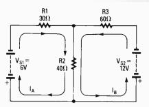
Fig. 5. Using the parts values and loops supplied you must solve for the currents through each component.
