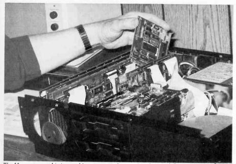
The Megamate card is inserted into an unused expansion slot in a PC XT clone computer. The 3.5-inch diskette drive connects to a jack on the read panel and requires no power plug.
