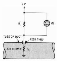
Fig. 2. Current is used to heat the sensing resistor while air flow cools the resistor down. As the resistor's temperature changes, its resistance changes, which shows up on M1.
