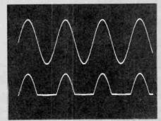
Fig. 1. Here we show how an AC waveform (uppermost) has its lower portion chopped-off by a half-wave rectifier.
