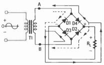
Fig. 6. The solid and dashed lines indicate the flow of current during the two half cycles of the AC waveform. Notice that the current to the load will always travel in the same direction.
