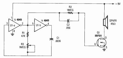
Fig. 5. This simple VFO circuit can be used for audible-tone testing, driving someone nuts or it can be transformed into a simple electronic musical instrument—an electronic organ, for example.
