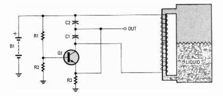
Fig. 7. As the liquid rises or falls in the container, it alters the inductance in the oscillator, and so it alters the output frequency also.
