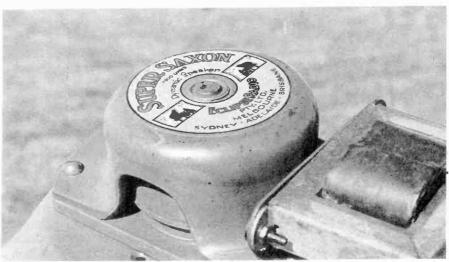
The field coil impedance of an electrodynamic speaker is usually marked on the back of the field coil. If the marking is no longer visible, it can be checked with an ohmmeter.
