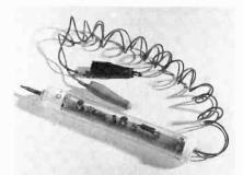
D. W. Naylor enclosed his logic probe in a clear plastic housing. A small brass screw was used as the probe tip.
