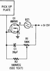
Fig. 3. The sensitivity of this Proximity Switch can be varied by adjusting R1. Note that R2 is specified as a 100-megohm unit, if that value cannot be located tie five 22-megohm resistors in series and use that combination for R2.
