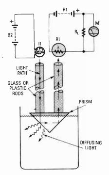
Fig. 8. When liquid wets the side of the prism, it allows the light to diffuse instead of reflecting it.
