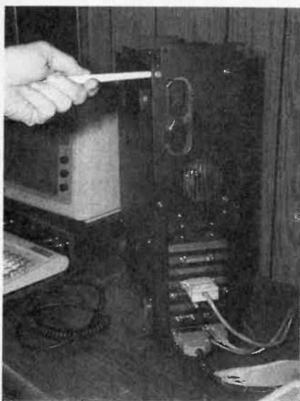
The rear panel has four mounting screws to secure the regulated power supply to the chassis. There are no mounting screws on the bottom surface of the chassis. The cables to the printer, modem, and monitor need not be disconnected.
