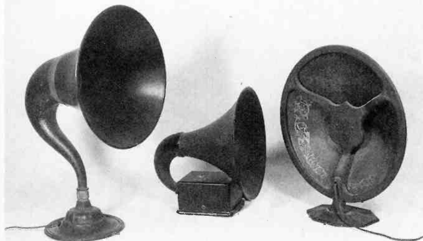
Horn-type speakers of the 1920's took many shapes and forms; two typical horn speakers are the ones made by Music Master (left) and Dictagraph (center). Cone-type speakers, like the Crosley unit (right), began to appear by the middle 1920's.
