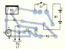
Fig. 3. If you've elected to etch your own printed-circuit board from the foil pattern provided, follow this layout.
