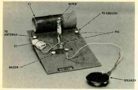
The positioning of the parts on the board you use is not critical. Notice how the capacitor is bundled instead of being rolled up to demonstrate how forgiving the circuit is.
