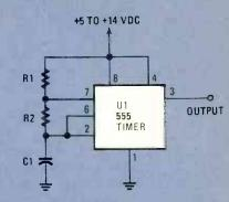
Fig. 1. Here's a 555 timer set up in its standard oscillating configuration. The timing is fairly independent of the supply voltage which is shown as a range.
