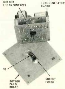
The bottom panel of the enclosure is made from a piece of printed-circuit material. A square hole is cut in its center to allow access to the control lever of S5 when the project is completed.
