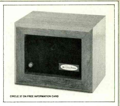
speaker. It plugs into any standard 110-120-volt outlet in an area where pests have been seen, such as the kitchen, basement, or attic. The only indication that the unit is powered is the red flashing-LED light. Dogs and cats were unbothered by its ultrasonic vibrations that range, according to the instructions, from 23 kHz to 56 kHz.
