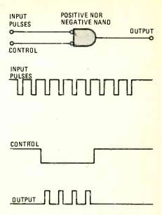
Fig. 7. A negative NAND gate can be used to control the flow of pulses. One input receives the input pulses, and the other a control signal. When the control goes low, the inverted input signal appears at the output as shown.
