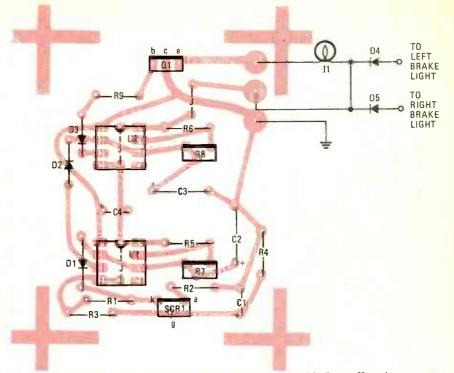
Fig. 3. You should use this parts-placement diagram as a guide for stuffing the parts on the PC board.
