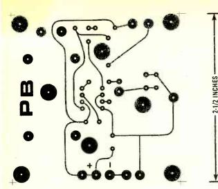
Fig. 2. Here is the printedcircuit pattern for the tonegenerator board.
