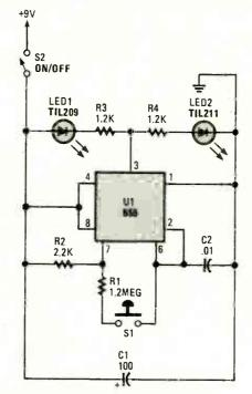
Fig. 4. The Coin Flipper is basically a 555 astable circuit that is used to drive LED1 and LED2.
