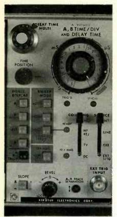
The horizontal-control group (with some trigger controls) is shown here. They are grouped for ease of use.
