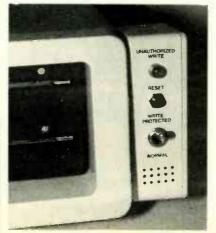
with audio and visual signals, and notifies DOS that the command was unsuccessful. A reset button turns off the light and buzzer, and the device itself can simply be switched off when it is not needed.
