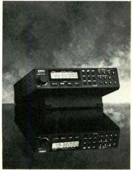
The Under Bearcat 950CXLT has 100-charnels divided into five banks of twenty each and features an optional CTCSS PL (selective calling) decoder board and something called "Service Scan," in addition to all of the usual scanner features.
