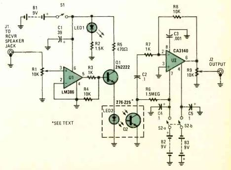
Fig. 1. The transmitting end of the TFOCIU circuit consists of an LM386 low-voltage audio amplifier (U1) feeding a 2N2222 general-purpose silicon NPN transistor, which is used to drive a light-emitting diode (LED2).
