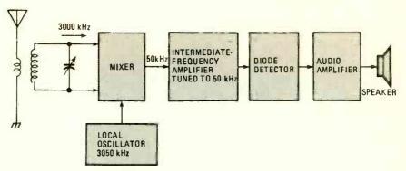
Fig. 2. Armstrong invented this receiver in 1918 to intercept German high-frequency radio communications. The mixer output frequency is the difference between the signal frequency from the antenna (3000 kHz) and the local oscillator frequency (3050 kHz). The 50-kHz signal is then amplified and sent to the detector for demodulation.
