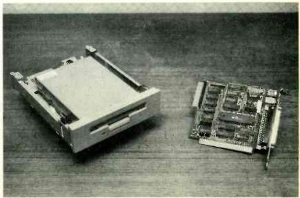
Add a 3.5-inch drive to your 8088-based machine with the CompatiCard. It allows four internal drives, and may function as a secondary disk controller.
