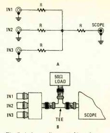
Fig. 8. A shows a linear combiner that allows us to connect 3 devices to an oscilloscope. In B we see the combiner coupled to a 50-ohm dummy load via a tee-connector for 50-ohm system use.
