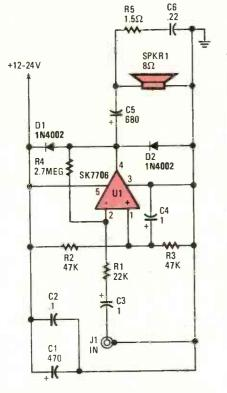
Fig. 2. The Practice Amp has a power output of under two watts.
