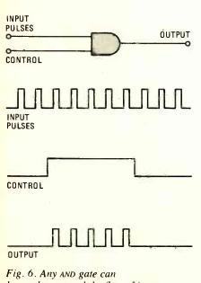
be used to control the flow of input pulses. One input is used to accept input pulses, and the other a control signal. If the control goes high, the input signal appears at the output as shown. complement is available. If the output must be exactly the same as the input, then of course an inverter can be connected to the NAND-gate output, effectively forming an AND gate.
