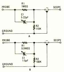
Fig. 5. The probe in A is a 10:1 ratio probe. Its output one tenth the input. In B we see the same sort of idea, but with an input/output ratio of 100:1.
