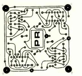
Fig. 3. Here is the printedcircuit pattern for the battery/amplifier board.
