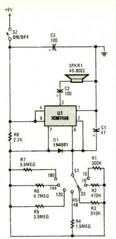
Fig. 6. The Telephone Bill Reducer is built around a 7555 CMOS oscillator/timer.
