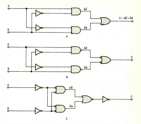
Fig. 11. An XOR can be simulated by combining ANDS, NOTS, and ORS (A); NANDS, NOTS, and negative NORS (B); or negative NANDS, NORS, and NOTS (C).
