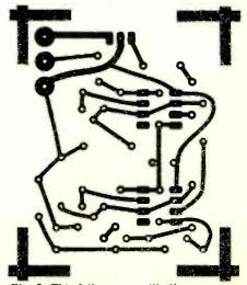
Fig. 2. This foil pattern will allow you to make a printed-circuit board of your own on which to mount the components.
