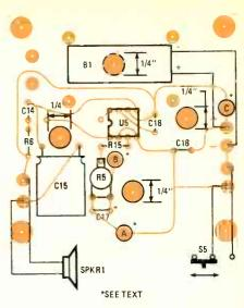
Fig. 5. Assemble the battery/amplifier board, using this layout diagram as a guide. Note the location of the battery, which is mounted on the board (located between four 1/4-inch donut pads as shown), and is held in place by a homebrew (wire) retaining system.
