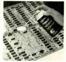
nents and systems with instant freezing of small areas to as low as  $-96^{\circ}F$  ( $-71^{\circ}C$ ). It is also useful for heat-sink protection of components during soldering and testing, and freezing of adhesives to facilitate removal.
