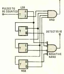
Fig. 8. Here two simple detectors determine when the number six is held by a counter made of flip-flops.
