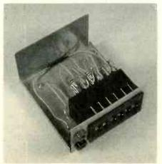
The thumbwheel and all the resistors of the R-Box fit easily into an enclosure measuring  $4 \times 3 \times 2$  inches.
