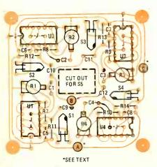
Fig. 4. Assemble the tone generator board, guided by this parts-placement diagram. It is important to note that the miniature mercury switches must be mounted about 4% inch above the board's surface.
