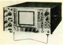
Storage oscilloscopes like this Iwatsu, allow you to capture a waveform(s) in memory for later viewing.
