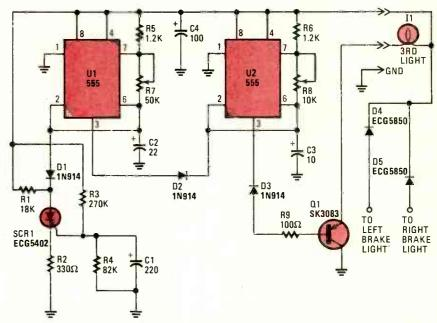
Fig. 1. The flasher consists of two timers with specially configured trigger connections. Integrated circuit UI controls when and how long the flashing should take place. Integrated circuit U2 oscillates to control the flashing itself.
