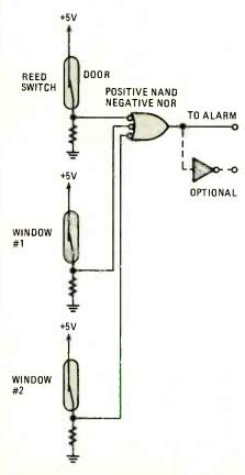
Fig. 10. Reed switches are monitored by a negative NOR gate to tell if a window or door has been opened.
