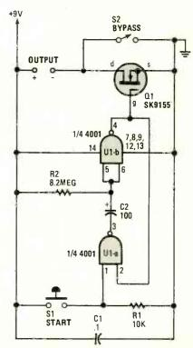
Fig. 5. This simple timer circuit is designed to shut down any device that is connected to it after a pre-set interval.
