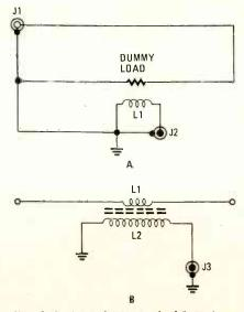
Fig. 9. In A we show a method for using a dummy load to couple att oscilloscope. The dummy load would be used in place of an antenna. Figure B shows a coupler used for displaying a current waveform. In general, a ferrite toroid is used for the current transformer.
