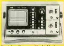
Special oscilloscopes, like this Viz, have the capability of triggering on either the horizontal or vertical TV-sync pulses.
