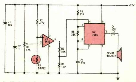
Fig. 1. The Lights-On Reminder sounds an audible alarm when the ambient light level falls below a certain point.
