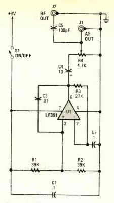
Fig. 3. The Signal Injector is comprised of a simple oscillator circuit (built around an LF351 JFET-input op-amp), with 100% negative feedback.
