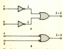
Fig. 3. An OR gate with inverted inputs (A) is called a negated NOR and is drawn with circles at the inputs (B).
