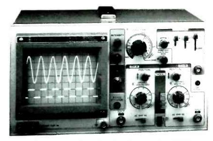
An interesting feature in this oscilloscope from JDR is Z-axis intensity modulation, which gives complex graphs a 3D feeling by altering the beam intensity.
