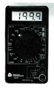
measures from 200-millivolts to 1000volts DC in 5 ranges; from 200 volts to 750 volts AC in two ranges; 200-microamps to 2-amps DC in 5 ranges; 200 ohms to 2 megohms in two ranges; and diode-test and FE measurements.
