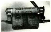
Here's a close-up of the Crosley's gridleak detector assembly. The resistance unit looks a lot like a small fuse. It snaps into a couple of spring clips mounted directly on the grid capacitor.
