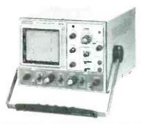
A 10-Mhz dual-trace oscilloscope, such as this B + K, is perhaps the most commonly used oscilloscope for hobbyist work.
