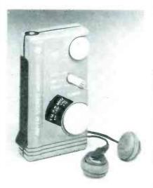
The blue and yellow receiver measures only 1.7  $\times$  3.3 inches, and runs on one AAA battery. The AM/FM-stereo reception offers clear sound; built-in automatic frequency control reduces station drift. There are no external antennas to get in the way. The FM antenna is built into the headphone cord and the AM antenna is built into the receiver.
