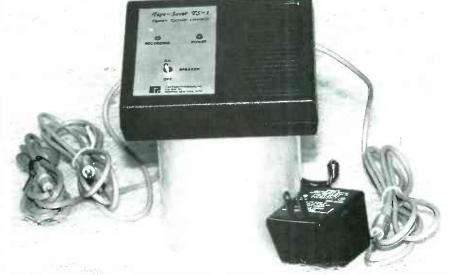
The Tape Saver TS-1 easily connects between your scanner and your cassette recorder via standard plugs. With the Tape Saver TS-1, the cassette recorder remains off during periods when there is no activity on the frequency to which the scanner is tuned. But when the channel is active, the recorder comes to life.
