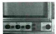
The main control group is shown here. The power switch on many scopes is ganged to the intensity control, but on this Kikusui, it is off to the left of the intensity adjust and is not shown here.
