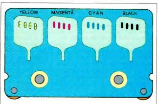
Each of the Xerox 1700's four print heads has four nozzles, for the three colors and black, to provide high resolution.
