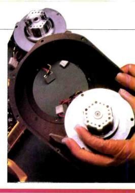
Tandon's aluminum disks are "bathed" in solution to form thin-film cobalt and nickel coatings, smoother and more rugged than oxide-coated media.
